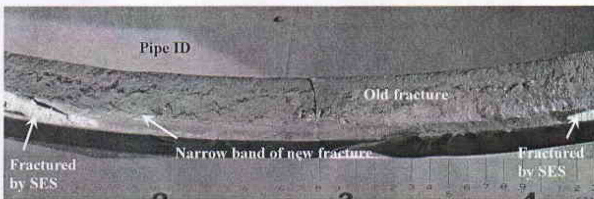
Figure 19. Photomicrograph showing fracture after crack was broken open. Scale divisions are 1/10 th inch.
