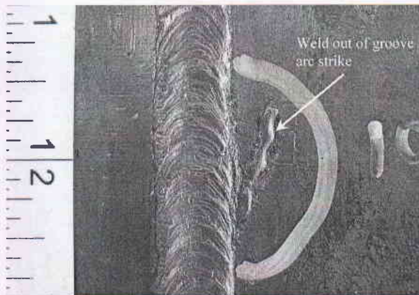
Figure 11. Photograph of root of girth weld in Sample 2. Arc-strike or out of groove weld is clearly visible. Scale divisions are 1/16 th inch.
