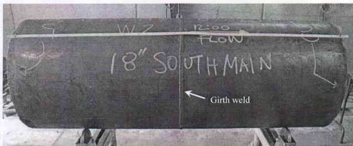
Figure 2. Photograph of pipe Sample 2 as received. Scale shown is in inches.
