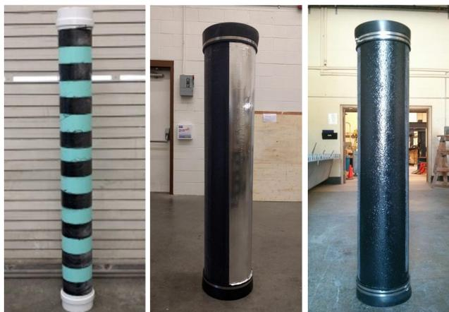
Figure 3. PVC pipe with CFRP rings, GFRP pipe with Aluminum strip, and GFRP pipe with carbon nanoparticle coating.
