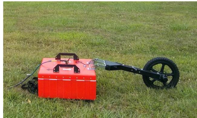
Figure 2. 200 MHz antenna with survey wheel.
