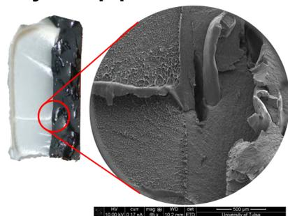
Figure 5: Scanning Electron Microscope image of a cross section of a bilayer PE specimen
