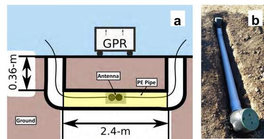
Figure 6: (a) Schematic of in-ground pipe testing setup (b) PE pipe used for testing.
