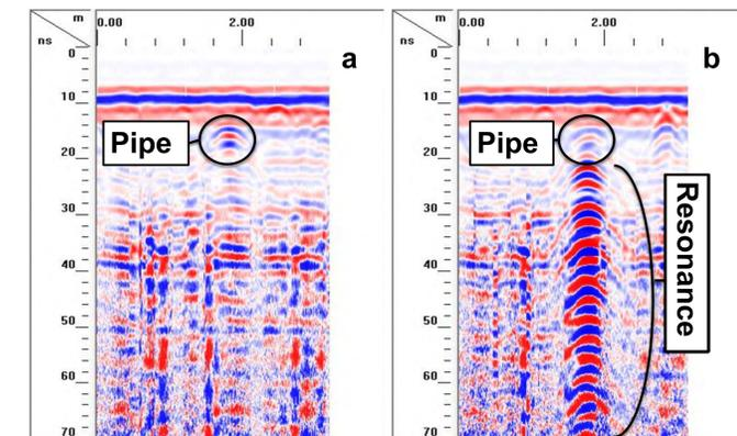
Figure 10: GPR B-scans of (a) PE pipe and (b) the same PE pipe with a cross polarization antenna.
