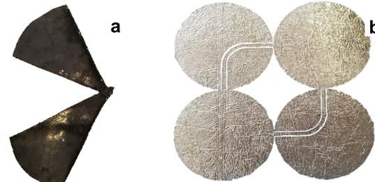
Figure 2: (a) A bowtie antenna made of conductive polyethylene and (b) a cross polarization antenna made from steel foil.
