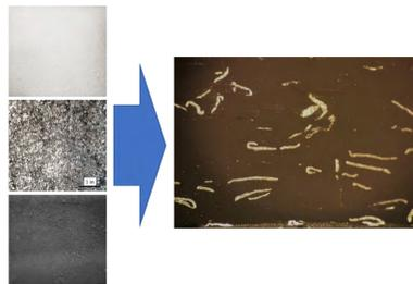
Figure 1: Aluminum flake and carbon black are compounded into PE to create an electrically conductive material.
