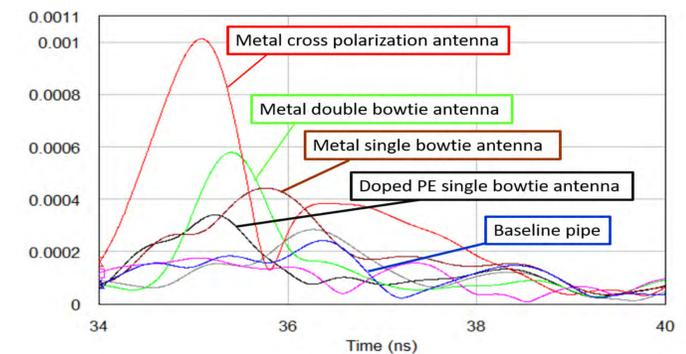
Figure 8: Response of metal and conductive PE antennas to GPR
