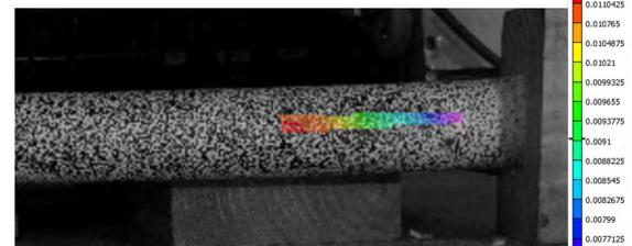
Figure 3: DIC was used to measure strains on a PE pipe.
