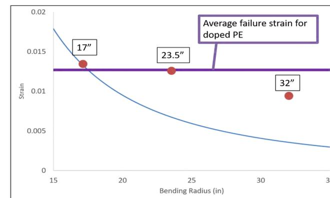
Figure 9: Measured strain on a 1" pipe in bending and the model prediction for strain.
