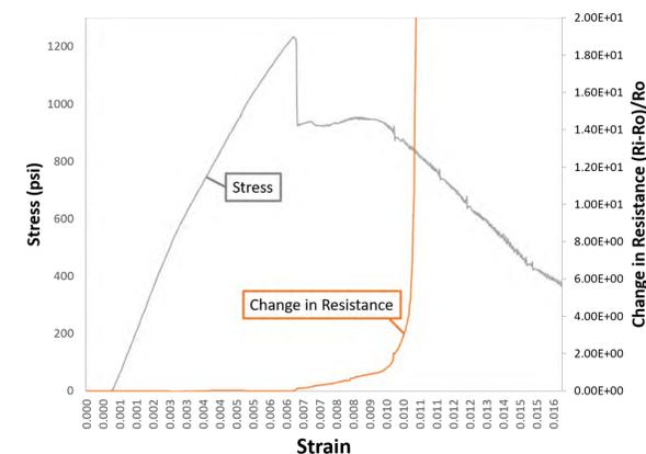
Figure 7: Stress and change in resistance vs strain for bilayer doped and neat polyethylene specimens
