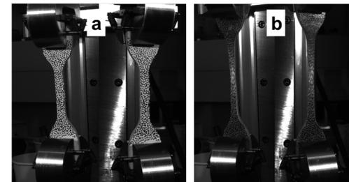
Figure 4: (a) DIC of doped PE specimens (b) DIC of neat PE specimens
