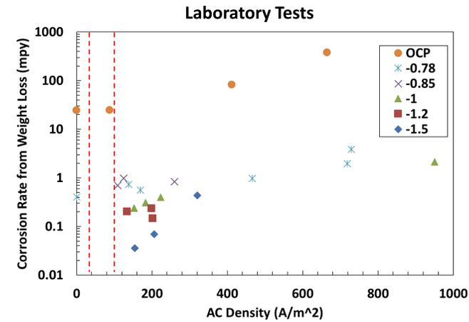
Results from laboratory mass loss experiments on X65 steel samples at various DC potentials exposed to AC voltage for 4-6 weeks. (Voltages vs. SCE)
