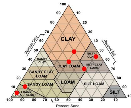
USDA soil texture triangle classifying soil types according to percentage of sand, silt, or clay content (<2mm = Sand, <50µm = silt, <2µm = clay). Red dots indicate soil compositions tested.
