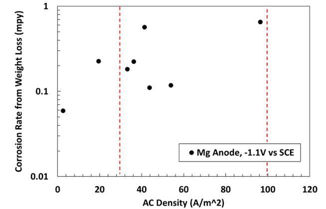
Results from field tests for X65 steel samples bonded to a CP test pipeline protected by a Magnesium anode system for 2-3 months.
