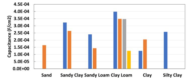
Interfacial Capacitance values of steel obtained for several tests in various soil types by fitting a parallel CPE circuit to EIS data and converting to capacitance with a formula by Hirschorn<sup>3</sup>.
