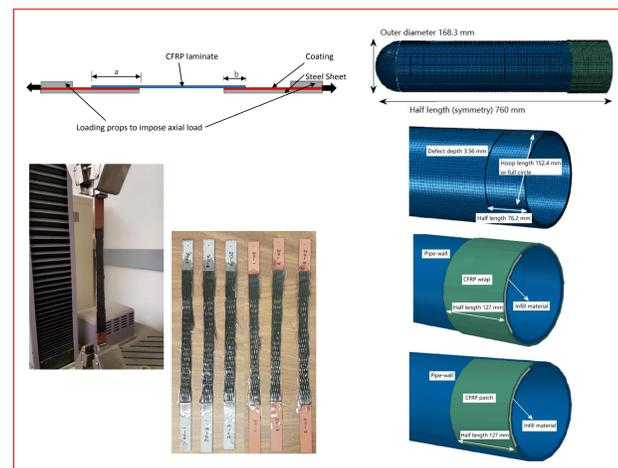
Figure 4. Bonding Strength between Coating and CFRP; Finite Element Analysis of Composite Repair.
