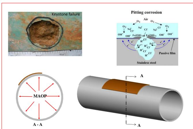
Figure 1. Pipeline Corrosion Failure and Repair.
