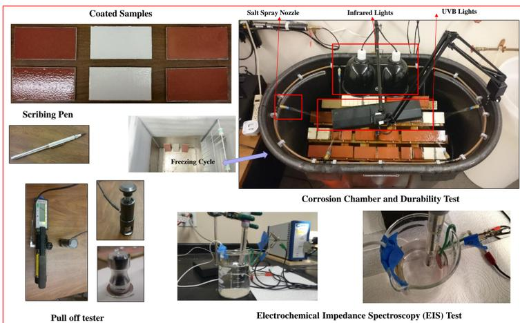
Figure 3. Electrochemical Measurement; Durability and Adhesion Strength after Accelerated Corrosion.
