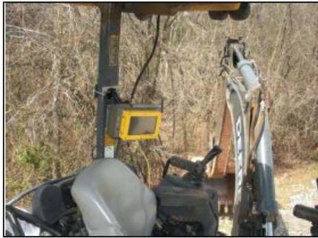
Successful deployment of digging triggers on backhoes & integration into the VA Pilot Program
