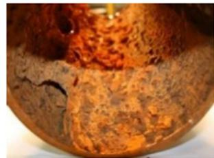
Figure 1. Internal corrosion<sup>2</sup>
