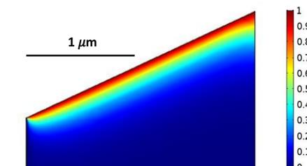
Figure 5. Results from implementation of the vacancy diffusion mechanism in finite element simulation.
