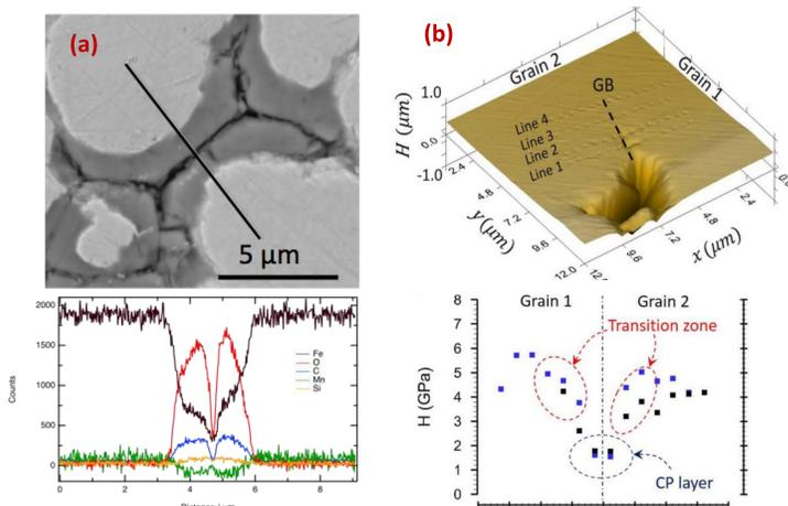
Figure 3. Experimental findings: (a) elevated Si in corrosion product (b) reduced-hardness layer near grain boundaries
