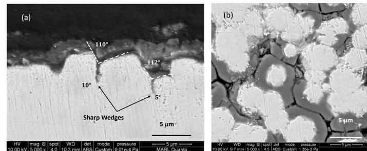
Figure 2. SEM images showing grain boundary (GB) corrosion product wedges. (a) Vertical cross section (b) horizontal cross section
