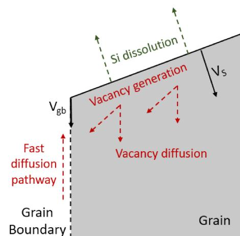
Figure 4. Diffusion model for vacancies introduced by selective Si oxidation. Vacancy diffusion along GB enhances  $V_{gb}$  relative to  $V_s$ , accounting for triangular wedge shape.
