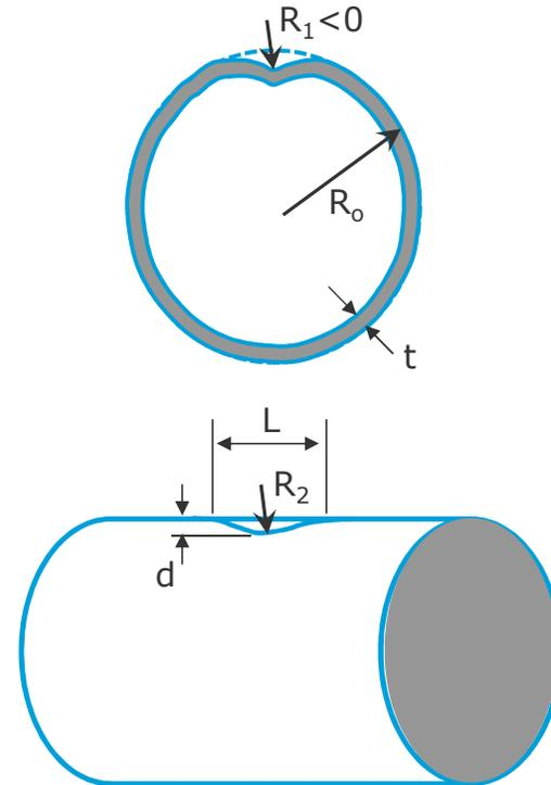
Not valid if the radius of curvature in any direction is less than 5 times the wall thickness!
