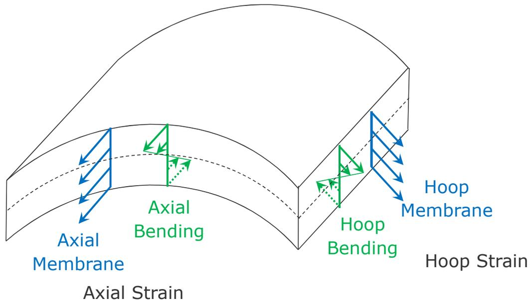
Circumferential membrane strain is assumed to be insignificant due to the flexibility of the pipe in the circumferential plane.
