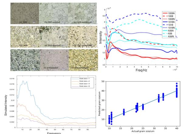
Figure 6. MBN and MAE experiments results
