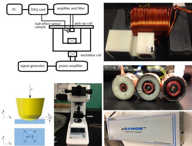
Figure 4. MBN and MAE experiments setup
