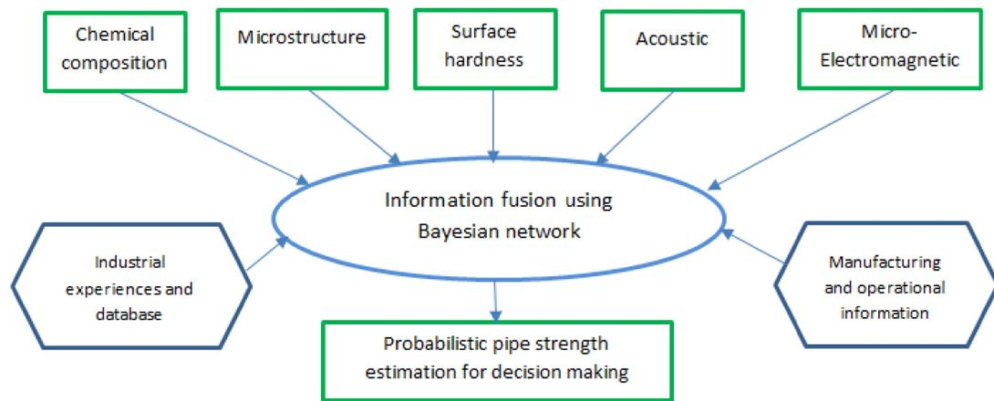
Figure 1. Schematic illustration of the proposed pipe strength estimation framework
