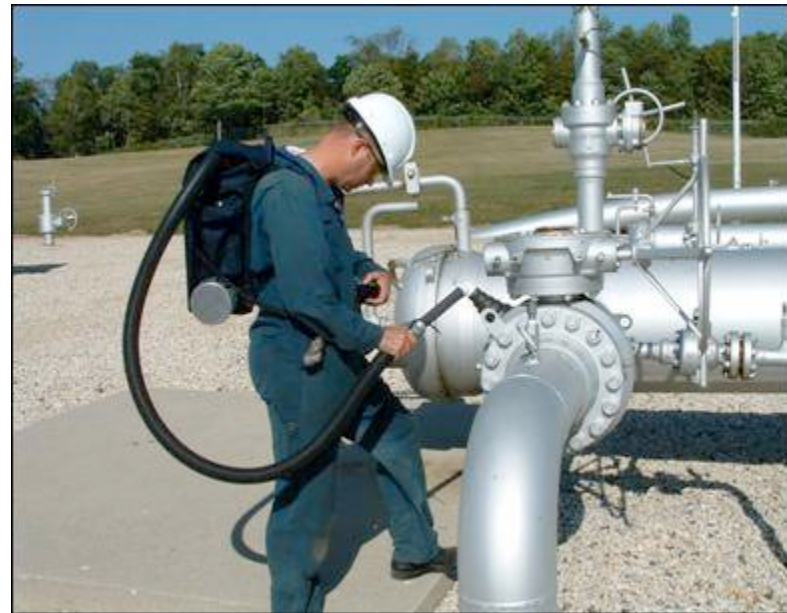
Leak Measurement Using High Volume Sampler
