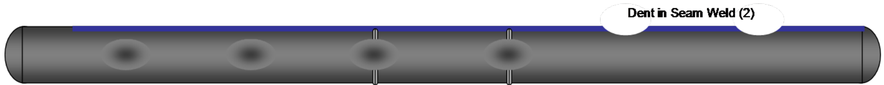
Side View of Pipe Sample (5 defects total)
