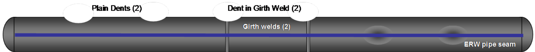
Side View of Pipe Sample (5 defects total)
