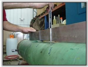
CPRS: Analysis of Adhesive Degradation
