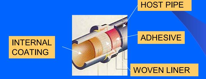
PSC approved CIPL for 6" & 8" Cast Iron mains Service liners up to 2"diameter with offsets
