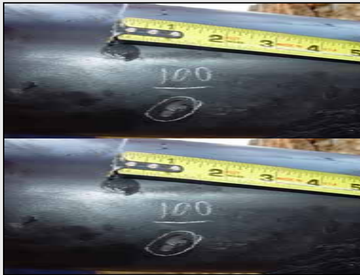
Corrosion defect 50 mils deep. Potential MIC.
