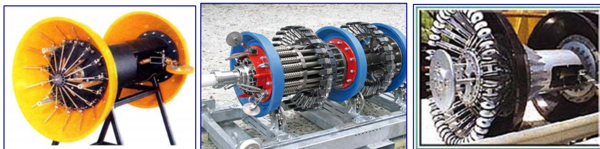
Figure 6.1 – Mechanical Caliper Tools (photos courtesy of Enduro, Rosen, and RAS GmbH)
