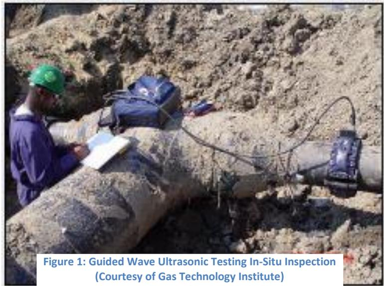
Figure 1: Guided Wave Ultrasonic Testing In-Situ Inspection
