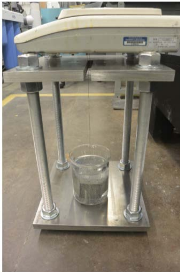
Figure 13 – Setup to determine submerged mass.
