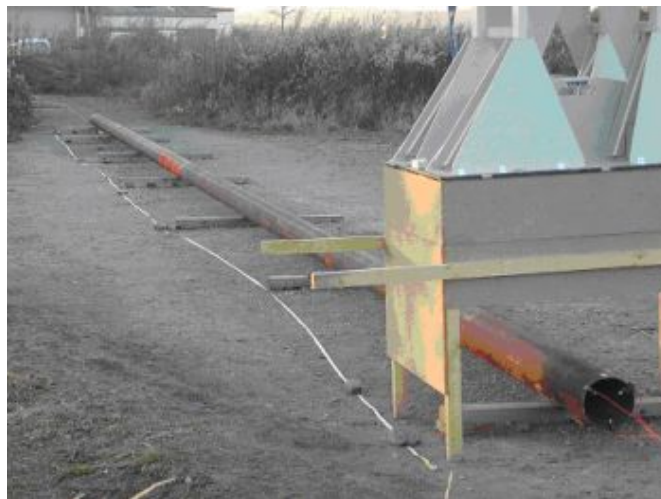
Figure 6.1. Joint #2 with joint #3 on test facility with platform to simulate pipeline coverage.
