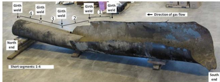
Photograph of the 28-foot-long ruptured section of pipeline
