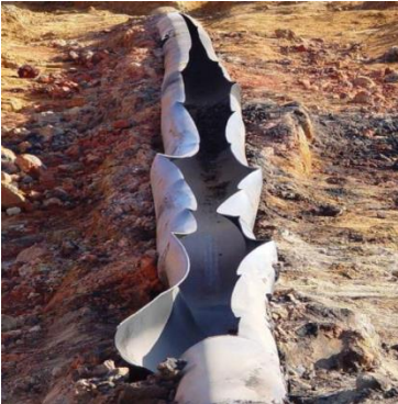
Photograph of the 28-foot-long ruptured section of pipeline
