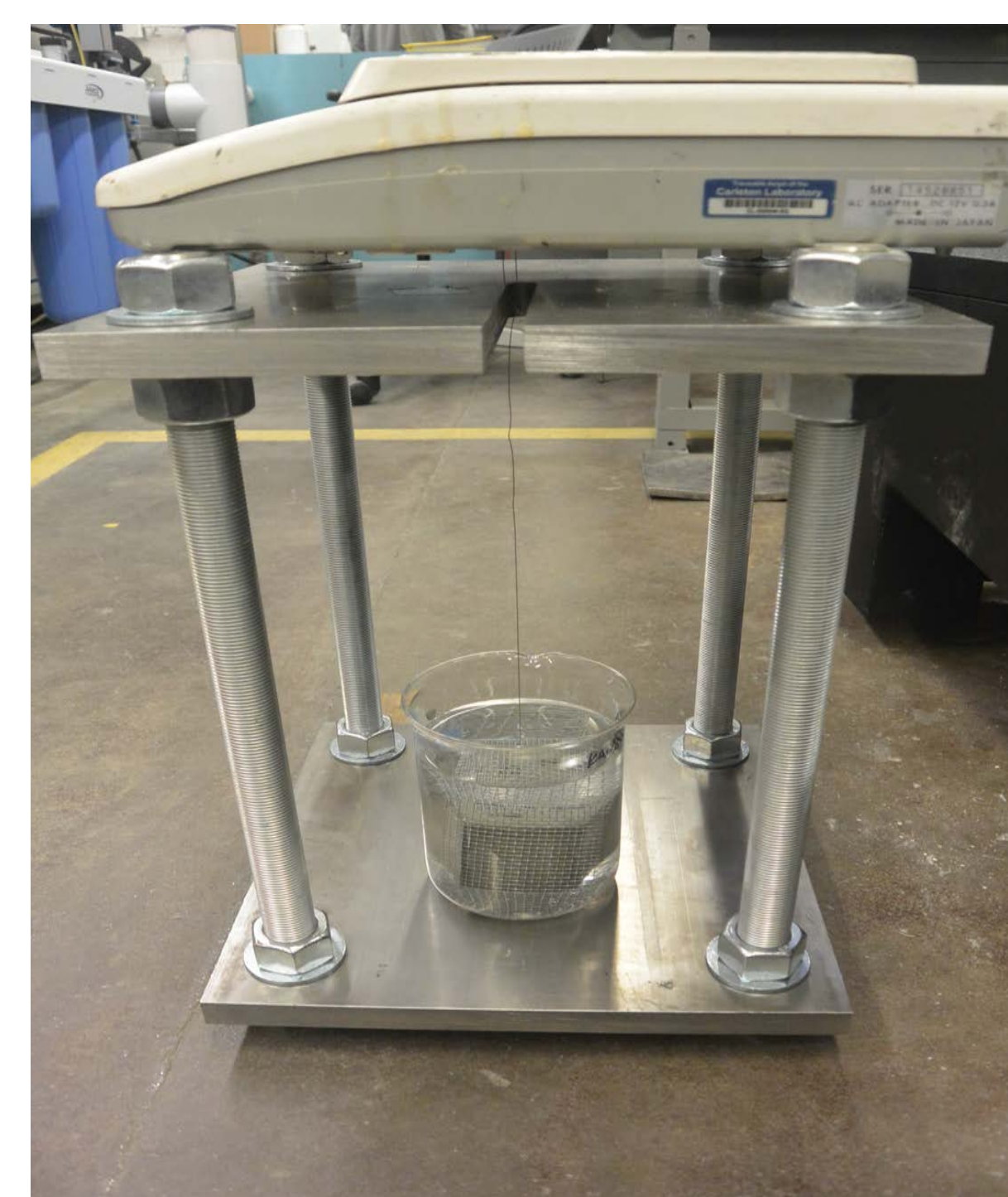
Figure 4. Test setup for measuring porosity
