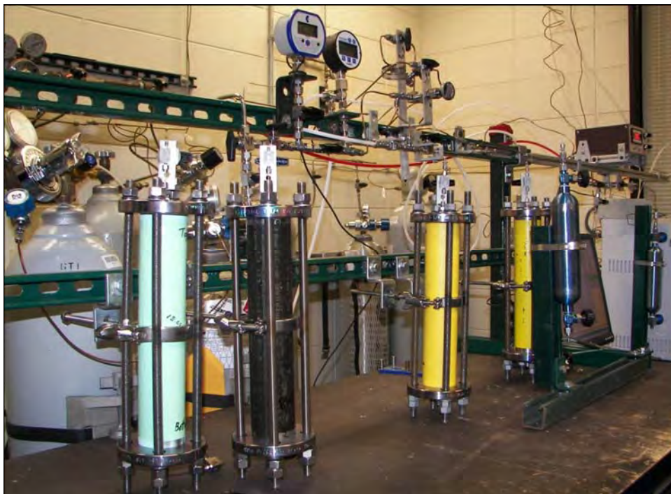
Figure 4. Setup for Static Testing of the Test Pipes
