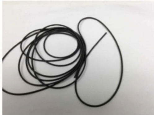
Figure 12: Sensor O-ring. Odyssian Technology has developed for the MDA a smart seal having sensor O-rings that were used to sense changes in sealing force, while at the same time acting as a sealing component. This same technology has been explored for use in O&G seals. Preliminary testing has shown that the O-ring material does change electrical readings when compressed, but additional characterization, material formulation and optimization, and algorithm development is required.
