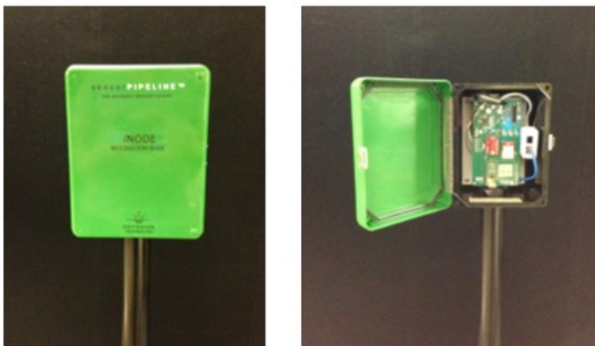
Figure 22: Shown are the sensor node (sNode) and integration node (iNode). Each sensor-laden device (i.e., sensorSEAL, etc.) on the sensorPIPELINE system has a dedicated sNode. Each sensor network, which has multiple sNodes has a single iNode that acts as the master node and is coupled to a single board computer (SBC).
