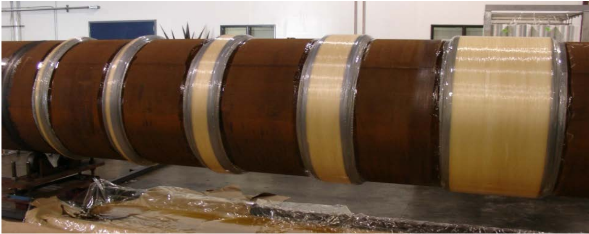
Figure 10 Wrapped SCA array onto test pipe
