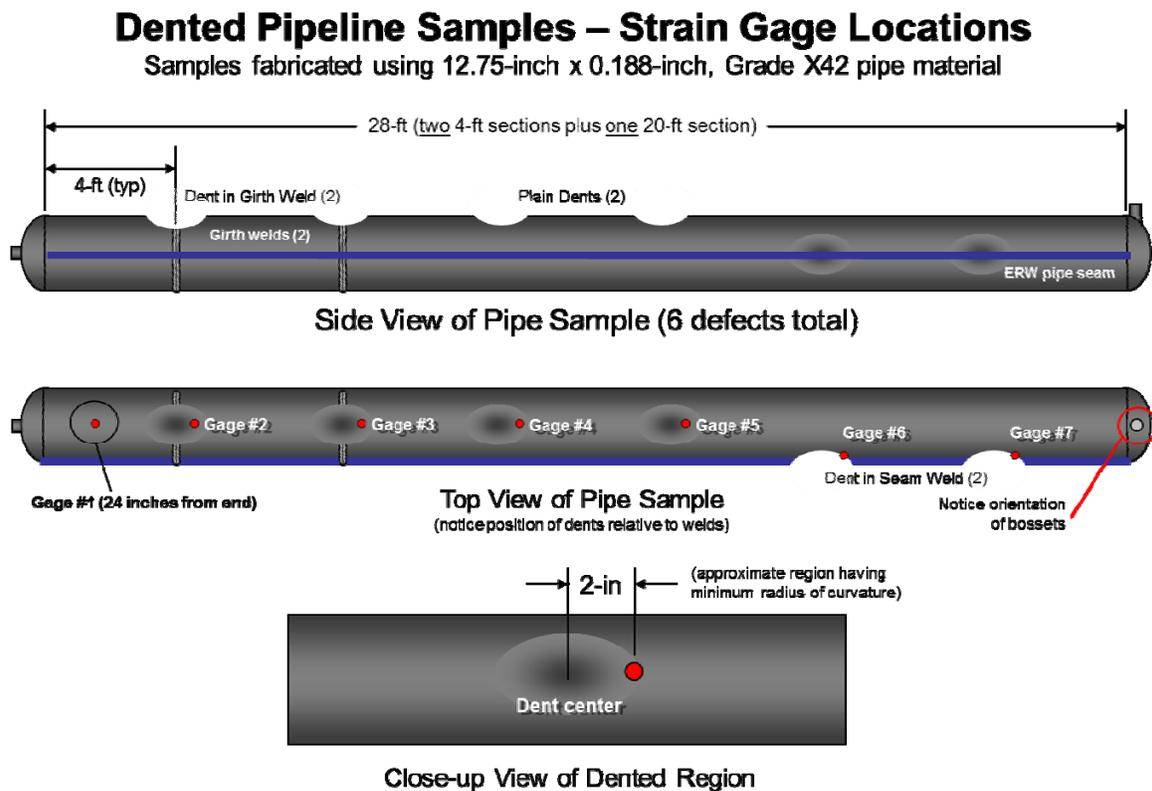
Figure 3 – Diagram showing set-up for the PRCI MATR-3-5 dent samples
