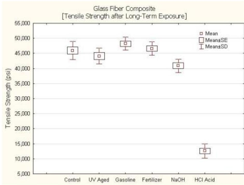
Figure 53 - Statistical mean values of the tensile strength of the glass fiber samples
