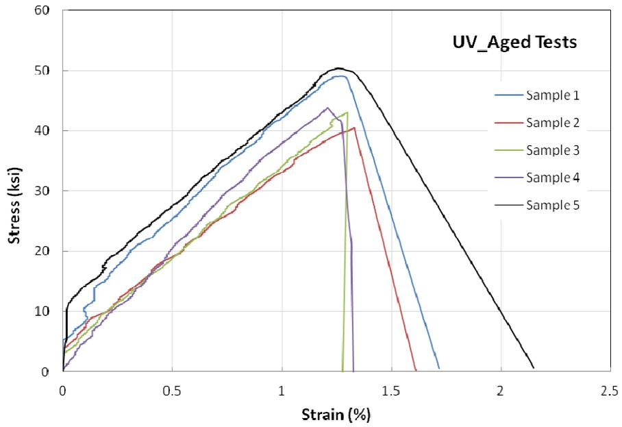
*Figure A-2 Fiber Glass Tensile Tests – UV Aged Samples*
