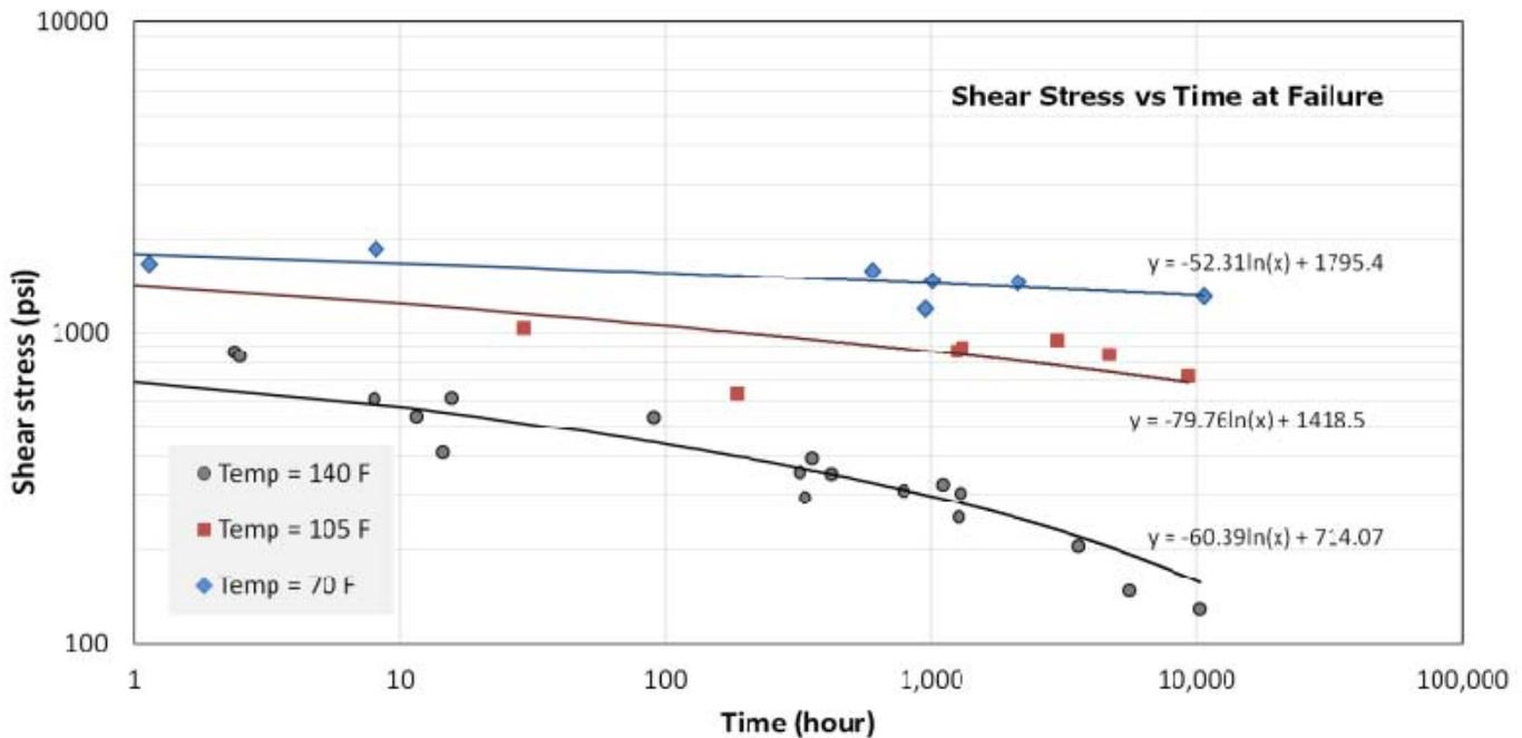
**FIGURE 5 - LONG-TERM RESULTS AT VARIOUS SHEAR LOADS FOR THE COMPOSITE**
