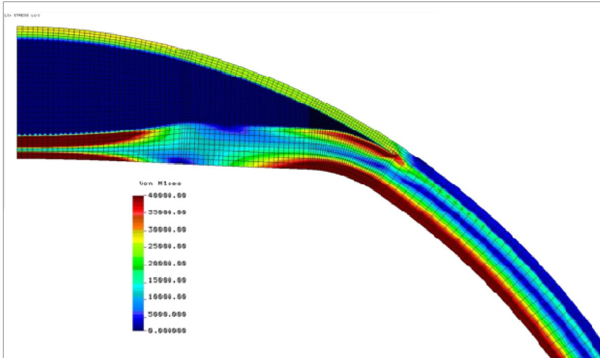
*Figure 11 - von-Misses stress plot at damaged area*
