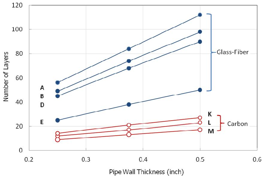
Figure 68 - Change of the repair thickness with pipe wall thickness
