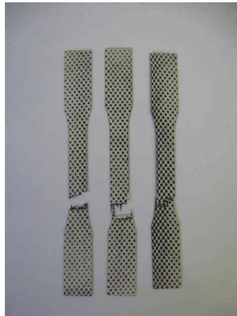
**Figures 1 & 2. Short-Term Tensile Ruptures for Fiberglass and Carbon**
