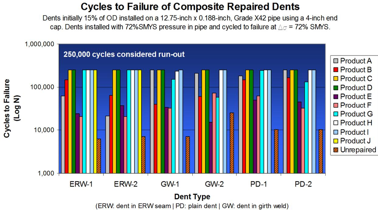
**Figure 4 – Pressure cycle to failure results for the PRCI MATR-3-5 dent samples**
