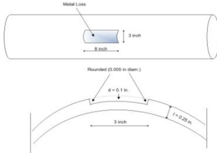
Figure 36 - Schematic of the metal loss in the pipe sample
