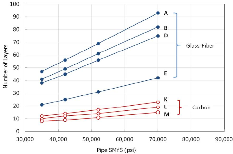
Figure 67 - Change of the repair thickness with pipe yield strength SMYS
