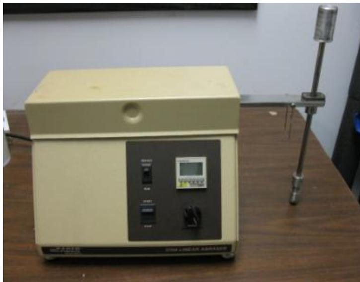
*Figure 61 - The Taber linear abraser device*
