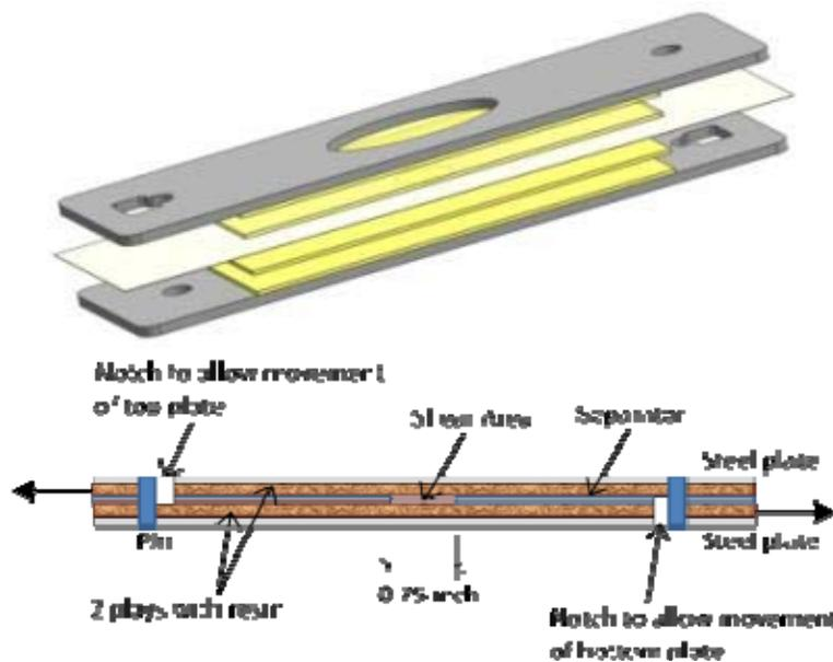
Figure 20 - Schematic and a cross section of the shear test specimen
