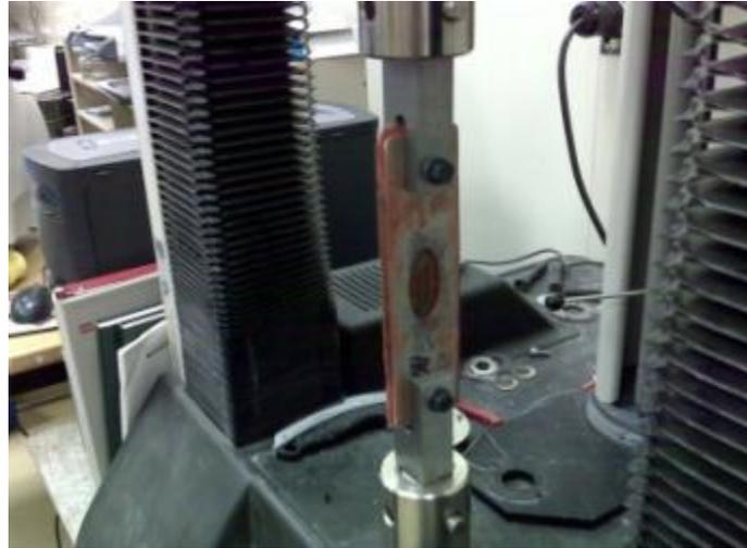
Figure 21 - Composite sample for short-term testing of the adhesive bond
