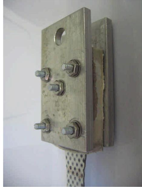
**Figures 11 & 12. Epoxy Block and Plate Clamp for Carbon Creep Tests**
