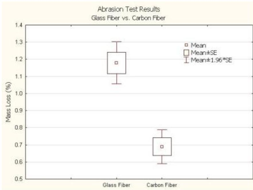
Figure 62 - Results of abrasion tests on the Glass and carbon Fibers
