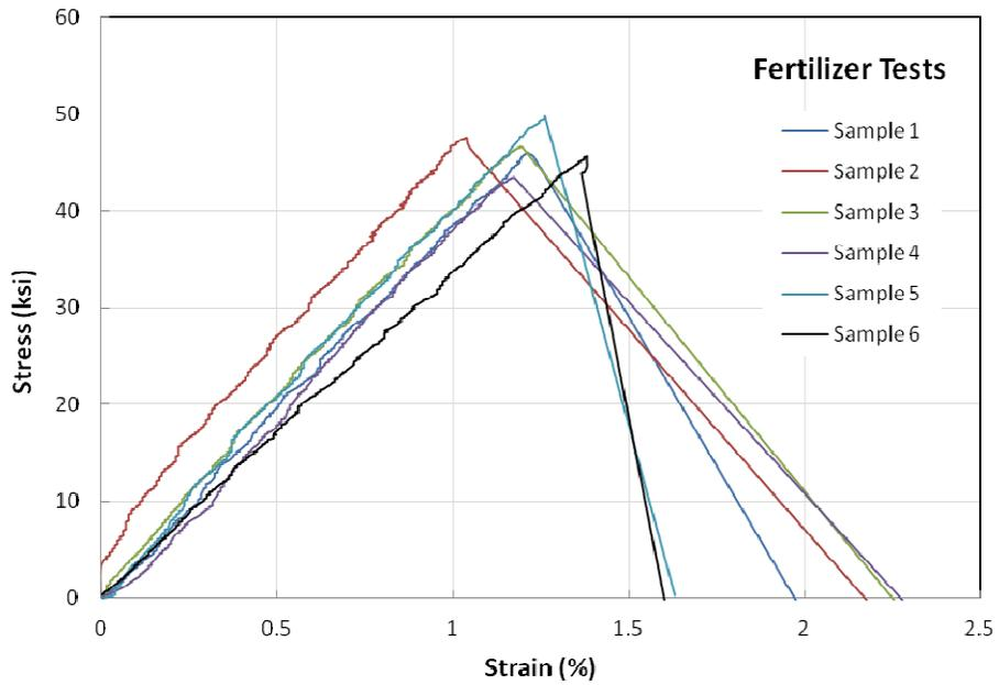
Figure A-4 Fiber Glass Tensile Tests – Fertilizer tested Samples
