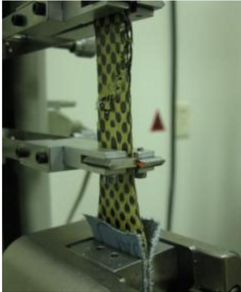
Figure 52 - Tensile test of UV-aged specimen
