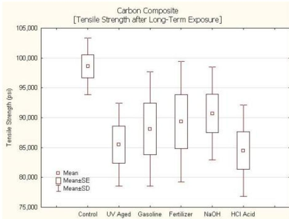
Figure 54 - Statistical mean values of the tensile strength of the carbon samples
