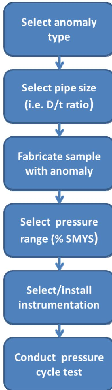
**Figure 1 – Flowchart showing elements of a pressure cycle test program**
