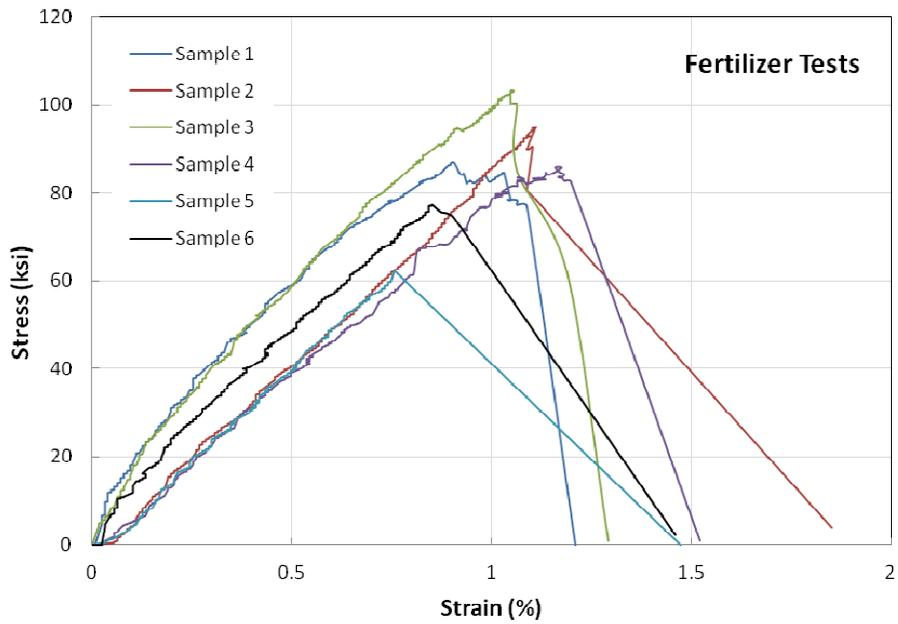
Figure A-10 Carbon Tensile Tests – Fertilizer Tested Samples
