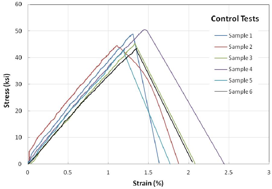
*Figure A-1 Fiber Glass Tensile Tests – Control Samples*
