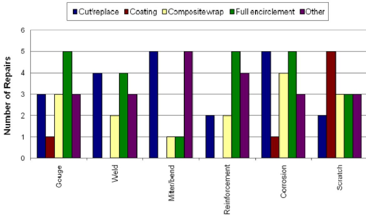
Figure 7 - Repair methods per given pipe condition
