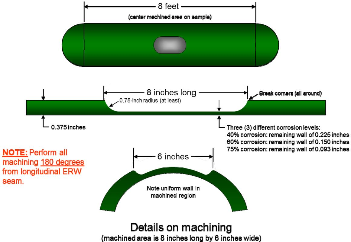
Figure 2 – Geometry for corrosion defects in PRCI MATR-3-4 stud
