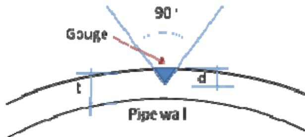
Figure 27 - Schematic of the gouge geometry in the pipe samples
