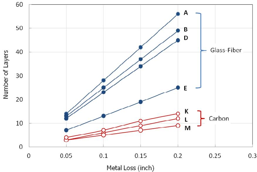
Figure 69 - Change of the repair thickness with pipe wall loss
