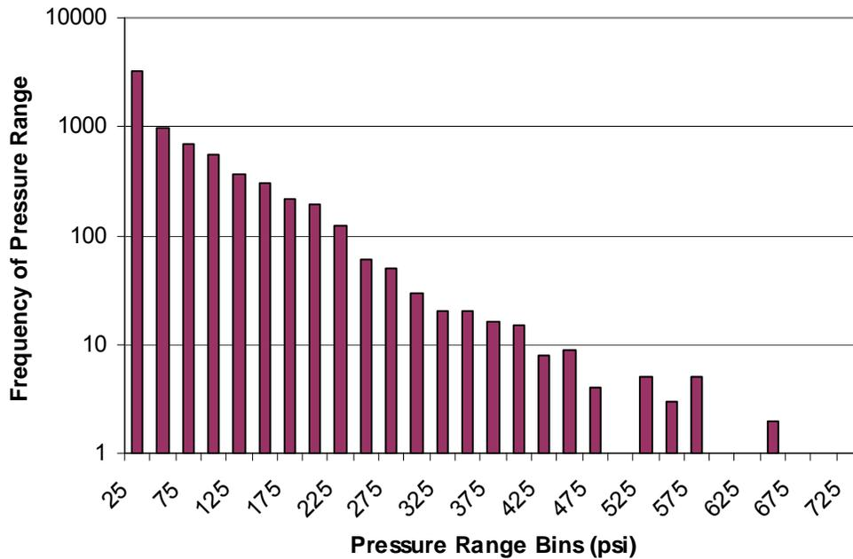
Figure 6 – Histogram of processed data from liquid transmission pipeline
