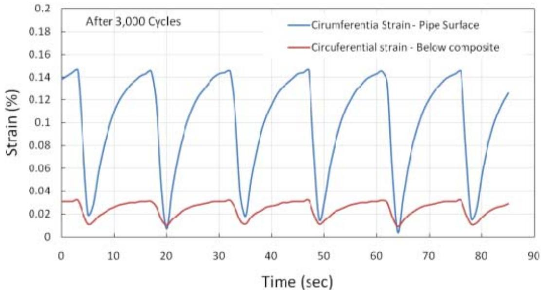
Figure 43 - Strain gages measurements on samples with and without repair
