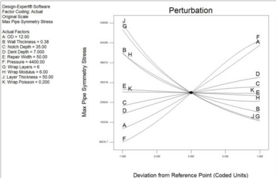
Figure 12 - Perturbation graph for maximum von-Mises stress in pipe (at notch location)
