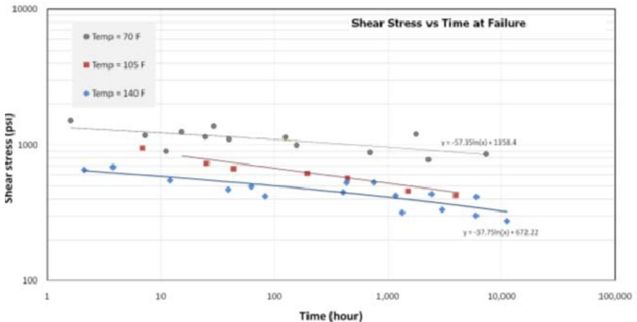
Figure 23 - Long-term bonding strength of composite U at various temperatures
