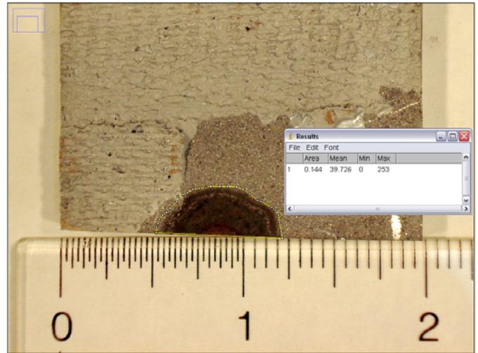
**FIGURE 8 - DIGITAL MEASUREMENT OF THE DISBONDED AREA IN A COMPOSITE WRAP**
