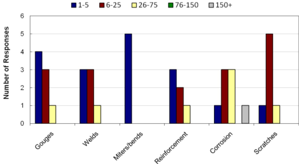
Figure 6 - Annual number of repairs per given pipe condition
