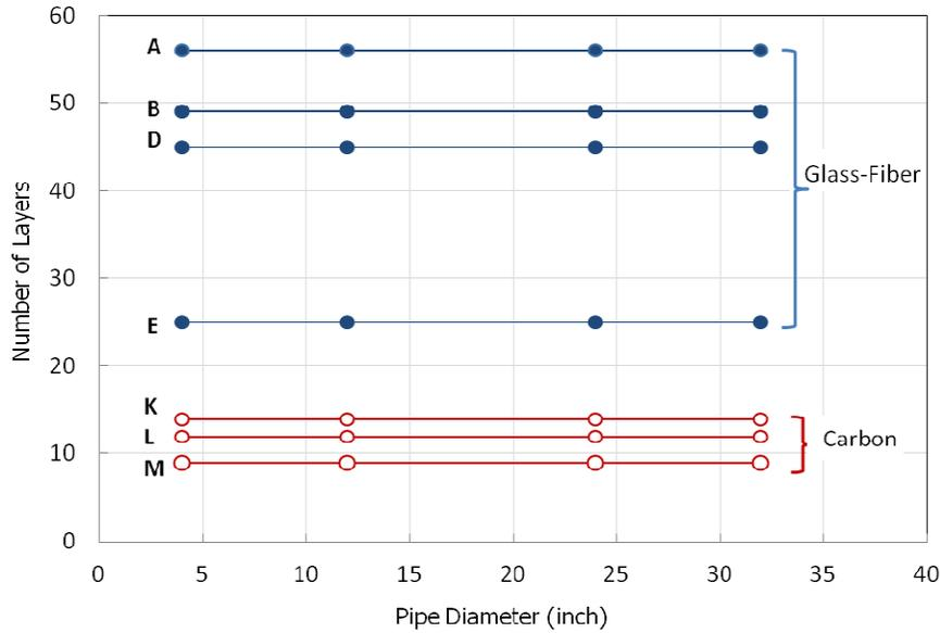
Figure 66 - Number of layers for various composite materials
