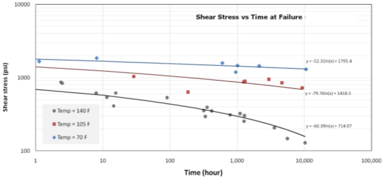
Figure 24 - Long-term bonding strength of composite H at various temperatures
