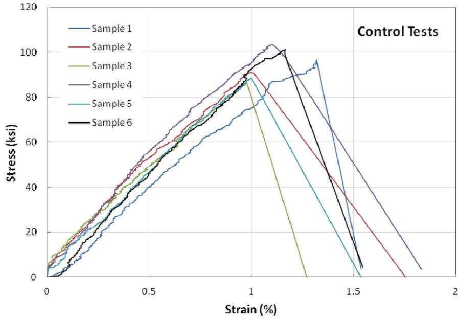
Figure A-7 Carbon Tensile Tests – Control Samples
