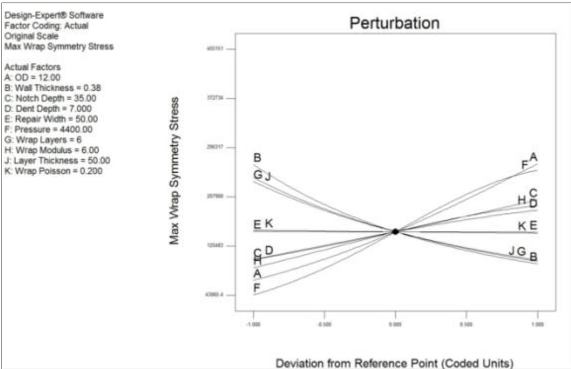
Figure 13 - Perturbation graph for maximum von-Mises stress in wrap (at notch location)
