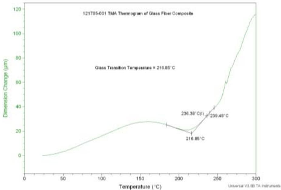
Figure 56 - TMA analysis for the of the  $T_g$  of the glass fiber
