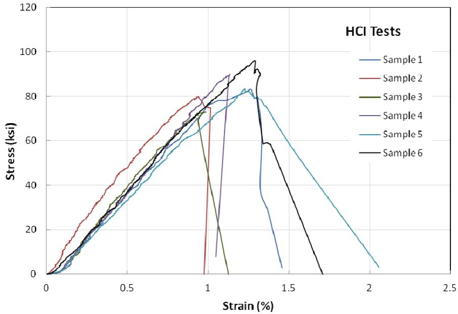
Figure A-12 Carbon Tensile Tests – Hydrochloric Acid Tested Samples
