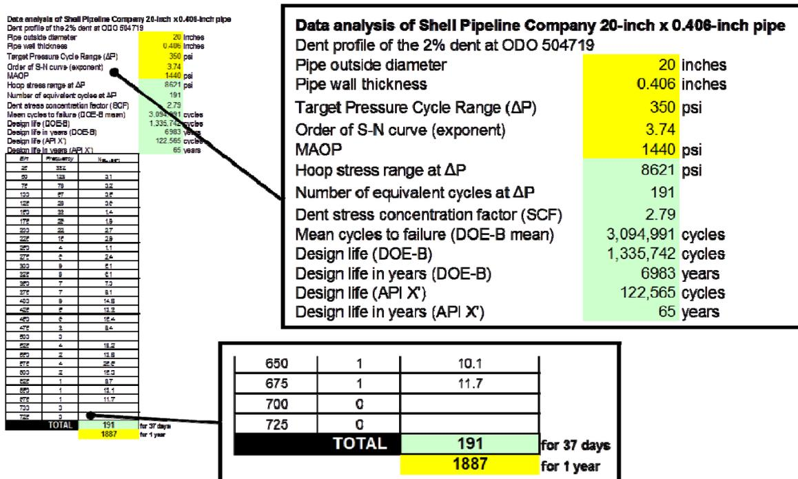
Figure 7 – Spreadsheet used to calculate an equivalent number of cycles
