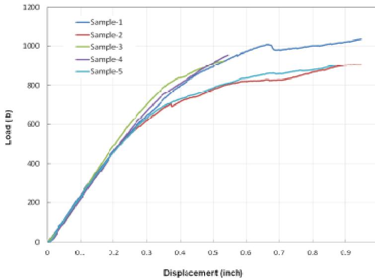
Figure 34 - Results of four-point flexural tests on the glass fiber composite
