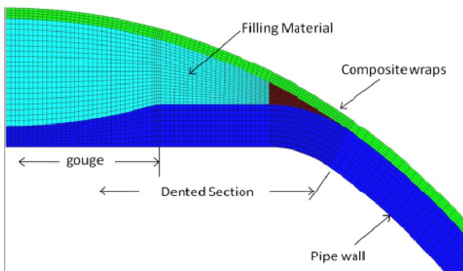
Figure 9 - Finite Element model geometry parameters
