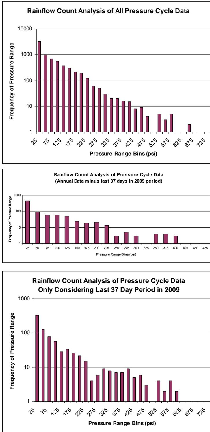
Figure C2 – Pressure Cycle Histograms for three time periods
