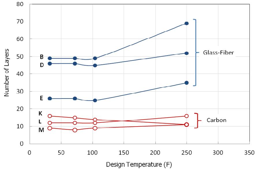
Figure 71 - Change of the composite thickness with temperature
