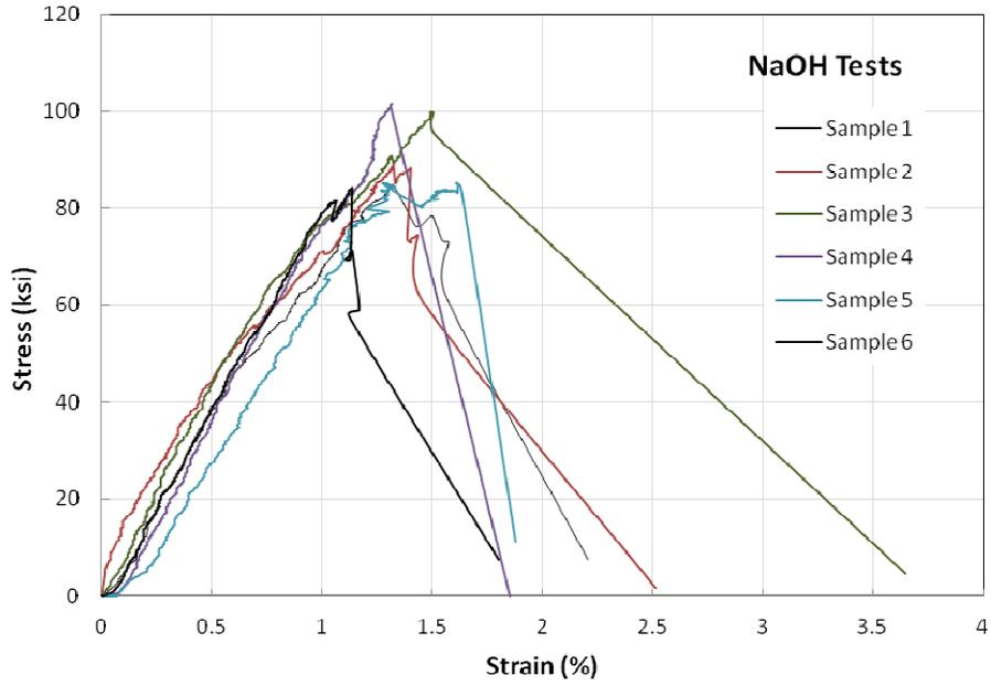
Figure A-11 Carbon Tensile Tests – Sodium Hydroxide Tested Samples
