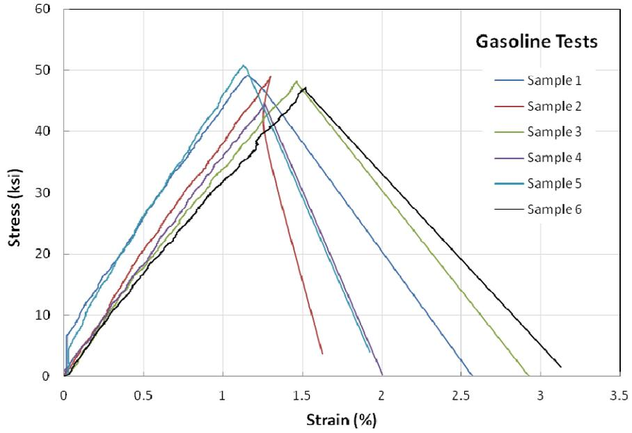
Figure A-3 Fiber Glass Tensile Tests – Gasoline Tested Samples
