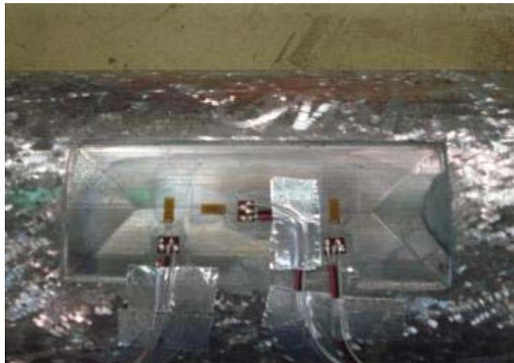
*Figure 41 - Strain gages installed on the pipe sample*
