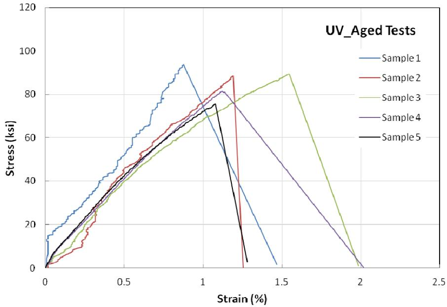
Figure A-8 Carbon Tensile Tests – UV Aged Samples
