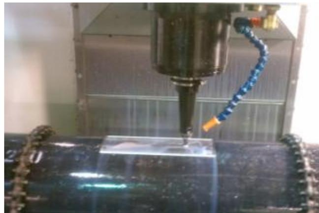
Figure 37 - Machining of the sample to simulate metal loss
