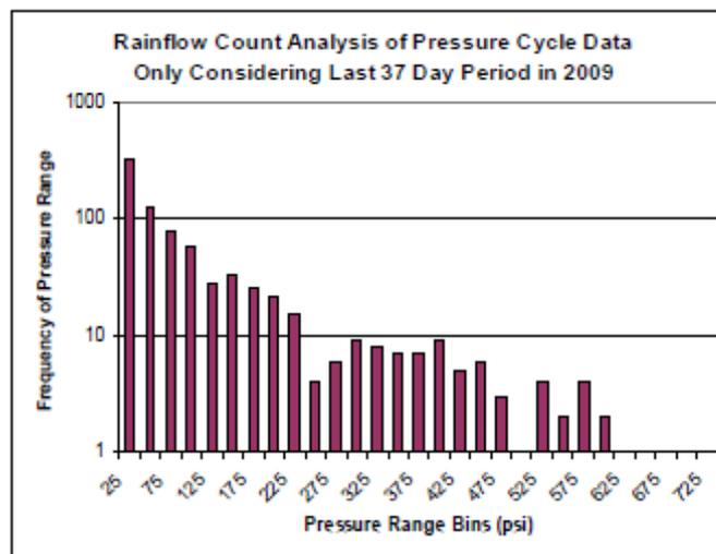
Figure 44 - Example of the frequency of pressure cycles (After SES Report, Appendix C)
