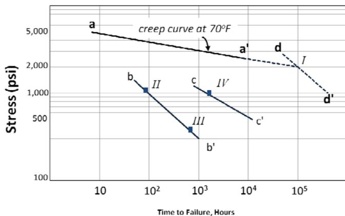
**FIGURE 6 - EFFECT OF TEMPERATURE ON THE LONG-TERM PERFORMANCE OF THERMOPLASTIC MATERIAL [8]**
