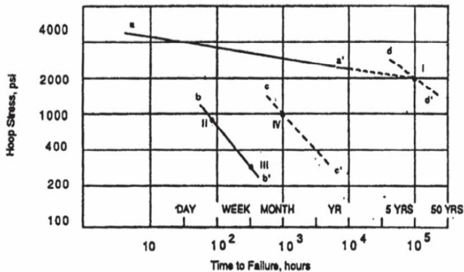
Figure 25 - Temperature effect on the long-term performance of thermoplastic material
