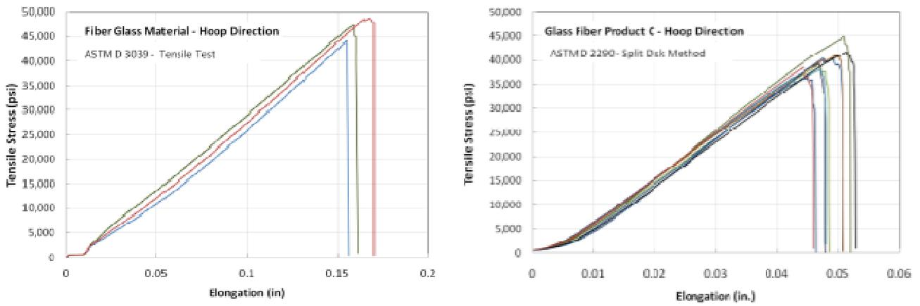
Figure 16 - Tensile test results for the glass fiber product
