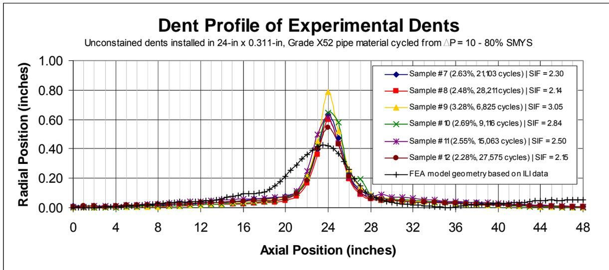
Figure 8 – Analytical versus experimental dent profiles in pipe
