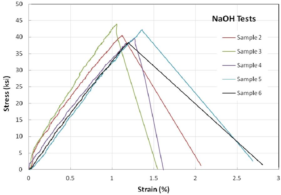
Figure A-5 Fiber Glass Tensile Tests – Sodium Hydroxide Tested Samples
