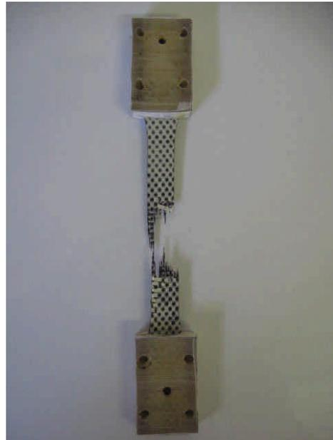
**Figures 9 & 10. Creep Ruptures for Fiberglass and Carbon at 60% UTS**
