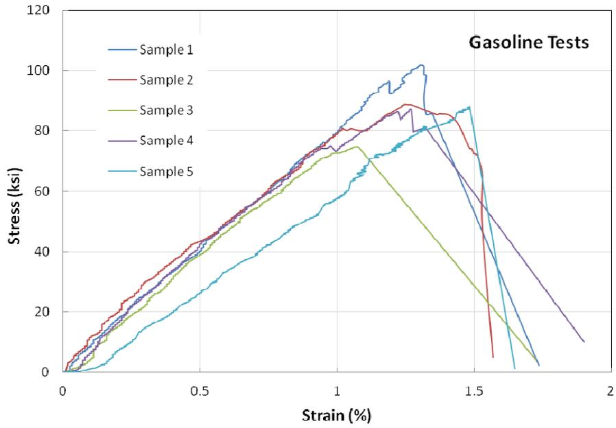
Figure A-9 Carbon Tensile Tests – Gasoline Tested Samples
