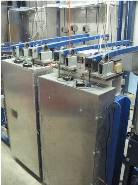
**Figure 3. Conventional Creep Frames**
