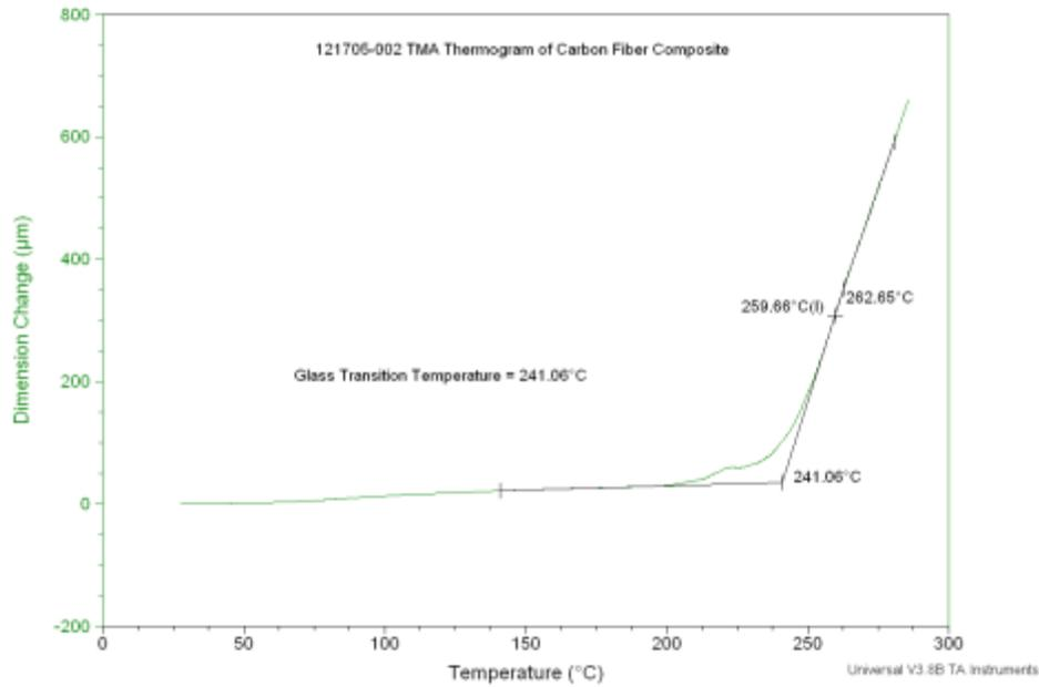
Figure 57 - TMA Analysis for the of the  $T_g$  of the carbon fiber
