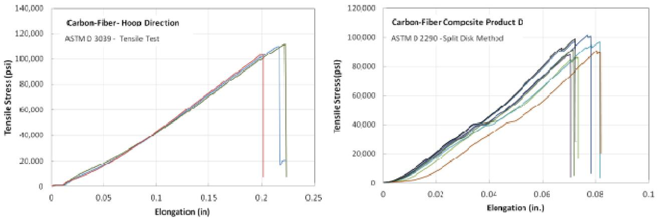
Figure 17- Tensile test results for the carbon fiber product
