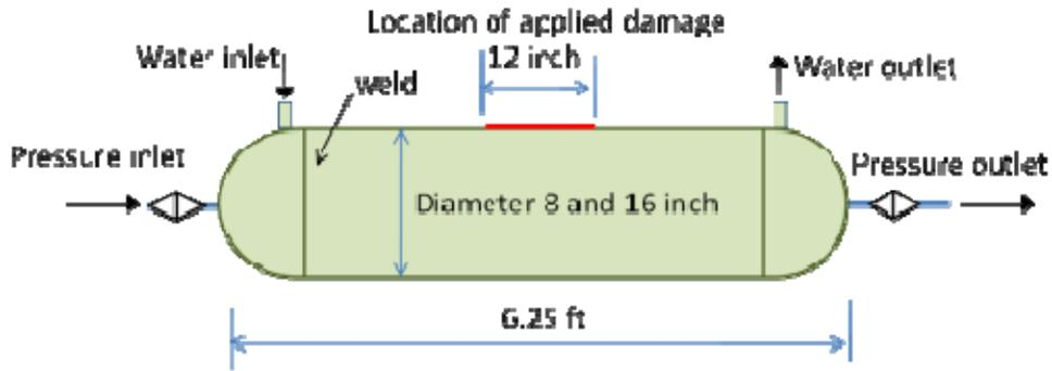
Figure 26 - Schematic of the hydrostatic pressure test specimen
