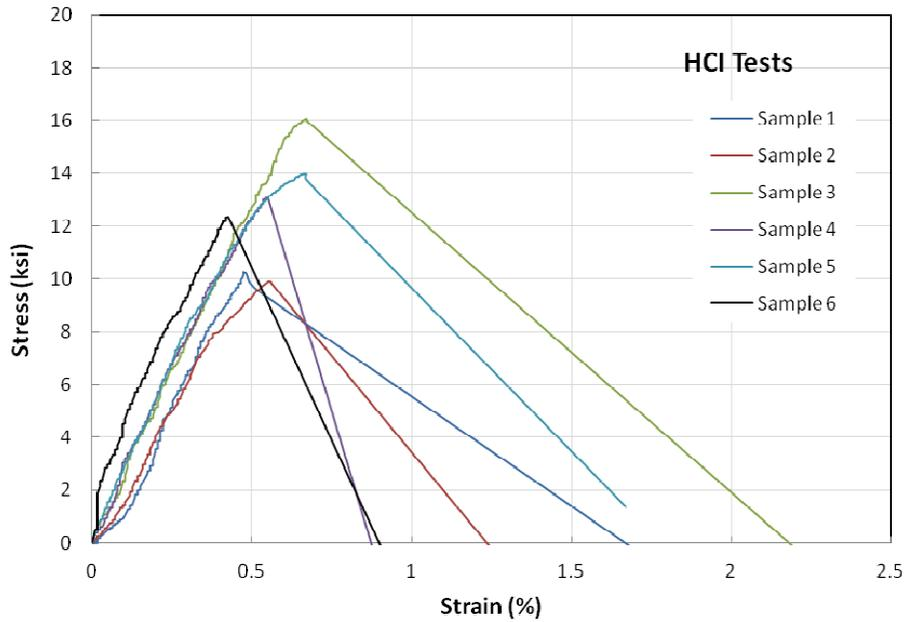
Figure A-6 Fiber Glass Tensile Tests – Hydrochloric Acid Tested Samples
