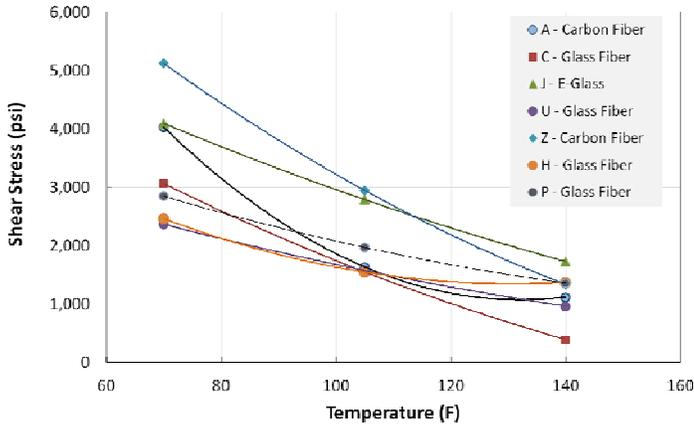
**FIGURE 4 - RESULTS OF SHORT-TERM SHEAR TESTS ON THE COMPOSITE SPECIMENS**
