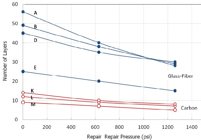
Figure 70 - Change of the composite thickness with pipe repair pressure
