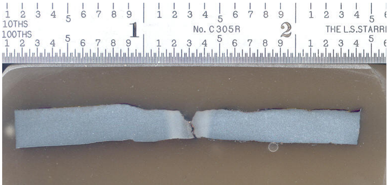
Figure 9. Appearance of the Selective Seam Weld Corrosion Associated with SSWC Failure Number 2
