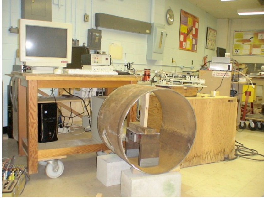
Figure 7-14: Pipe section BEA161 with MFL magnetic inside
