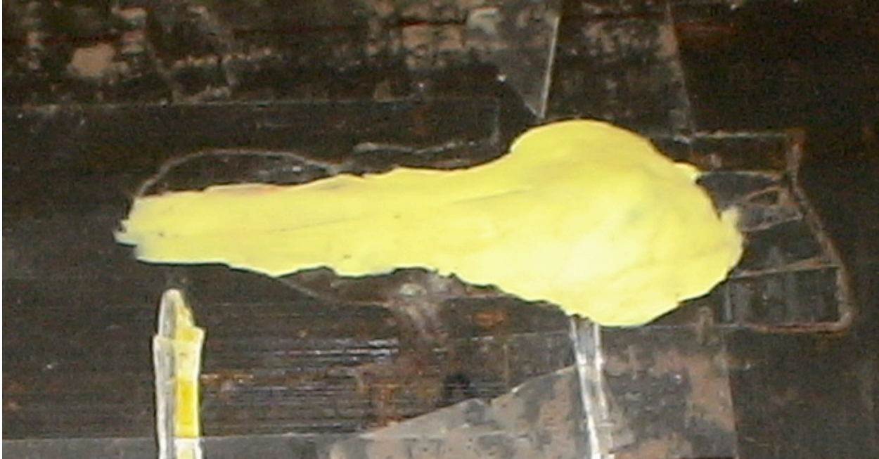
Figure 6- 3: Photograph of the gouge defect 5B, which has been covered with clay to allow a smooth path for the MFL detector probe.
