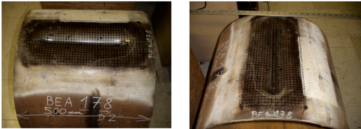
Figure 7-19: Photographs of gouge+dent BEA178 in pipeline section sent to NIST for residual strain measurements.
