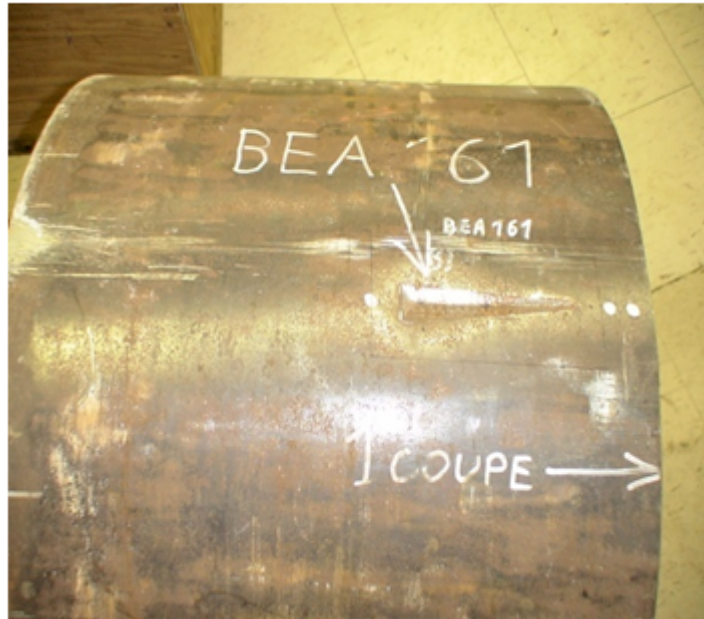
Figure 7-13: Pipe section containing showing gouge BEA161 location
