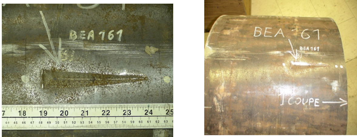
Figure 8- 1: Photographs of BEA161 – on the left is a closeup of the gouge, with a ruler indicating the size. On the right is shown the pipe ring that was sent to NIST and Queen’s which contained the gouge. Note the close proximity of the gouge to the end of the pipe ring - this was done deliberately to facilitate neutron diffraction measurements at NIST.
