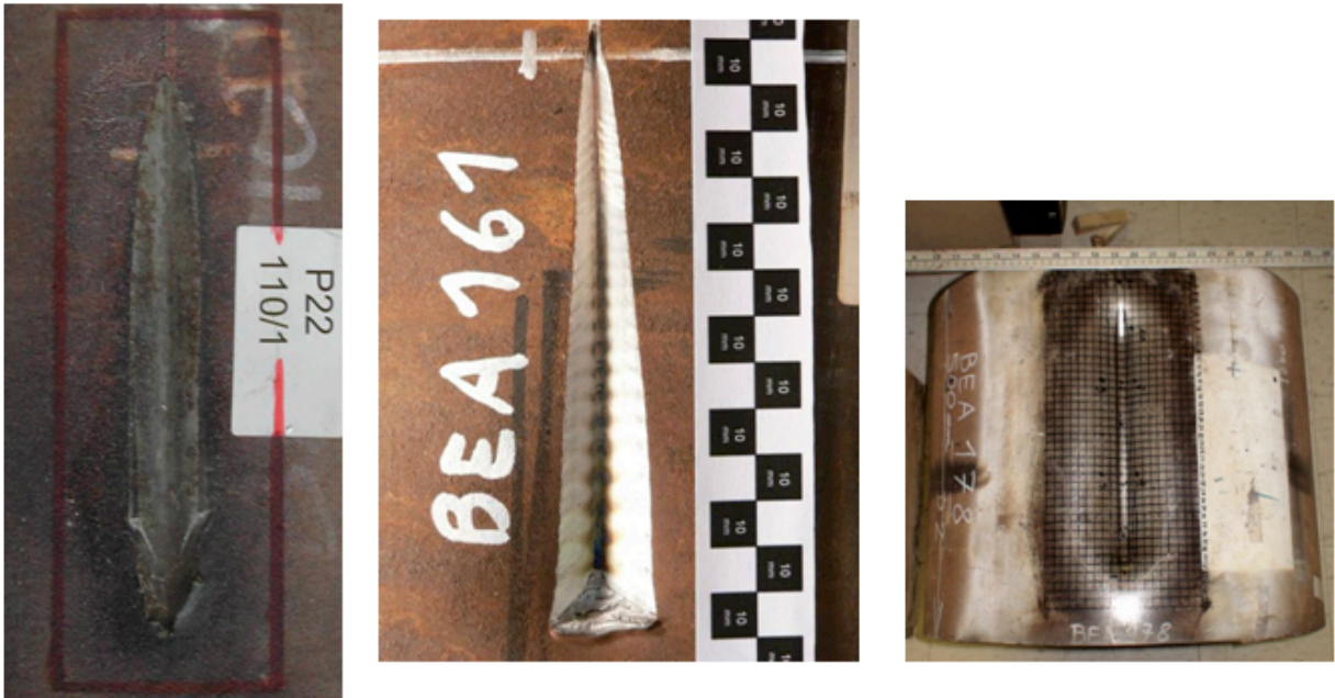
Figure 7-2: The three gouges examined using neutron diffraction. Sample P22 (left) is a coupon sample containing a 17 cm gouge (tool entry at top end). Sample BEA161 (center) is a 13 cm long wedge-shaped gouged contained in a 60 cm long, 60cm diameter pipe ring of X52 steel (tool entry at top end) . Sample BEA178 (right) is also a pipe ring sample (X52 steel) containing a long gouge with a significant associated dent.
