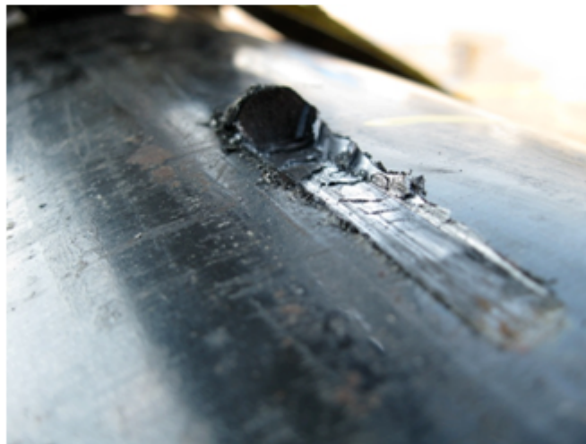
Figure 6- 2: Two examples of typical gouge geometries produced using the SES gouging apparatus, shown at different angles. The length of the gouge is approximately 5cm. Note that the gouging process did not produce this gouge geometry in the Pipe 1 samples – in fact the samples appeared barely scratched.
