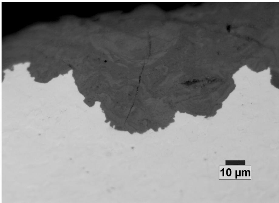
**Figure 2.12. Cyclic Four Point Bend (FPB) tests on pipeline sample (sample#14) tested in commercial grade fuel grade ethanol (FGE) with 51ppm chloride tested at maximum cyclic load of 4500 lbs. This sample did not show any SCC**
