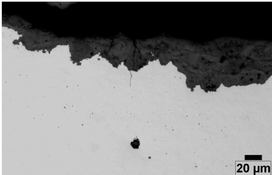
**Figure 2.11. Cyclic Four Point Bend (FPB) tests on pipeline sample (sample#14) tested in commercial grade fuel grade ethanol (FGE) with 51ppm chloride showed SCC even at the Maximum cyclic load of 5000 lbs.**
