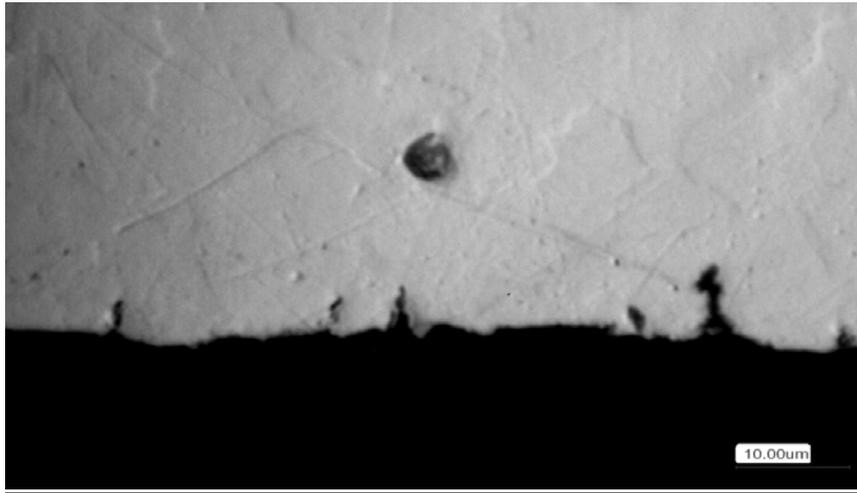
**Figure 1.2. Cyclic TTTM sample exposed to SFGE-3 (50 ppm Cl) for 15 days. Sample showed small pits and small SCC propagating from these pits. Equivalent constant load tests did not show crack propagation.**
