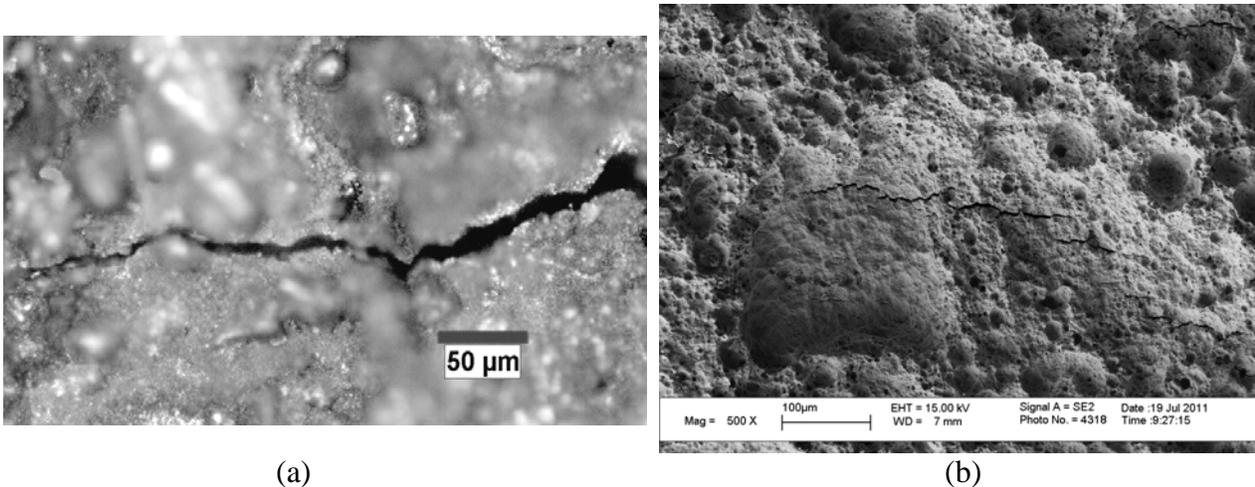
**Figure 2.5. Surface cracks in the mill scaled surface of Cyclic FPB tests on pipeline sample (sample#7), a) with mill cracked mill scale at the surface, b) After mill scale removal, showing SCC in the pipeline steel**
