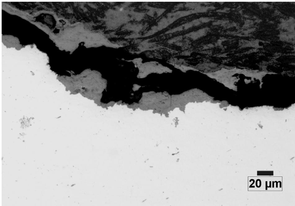
**Figure 2.10.** Cyclic Four Point Bend (FPB) tests on pipeline sample (sample#13) showed no SCC in commercial grade fuel grade ethanol (FGE-S). Maximum cyclic load for this test was 5000 lbs.
