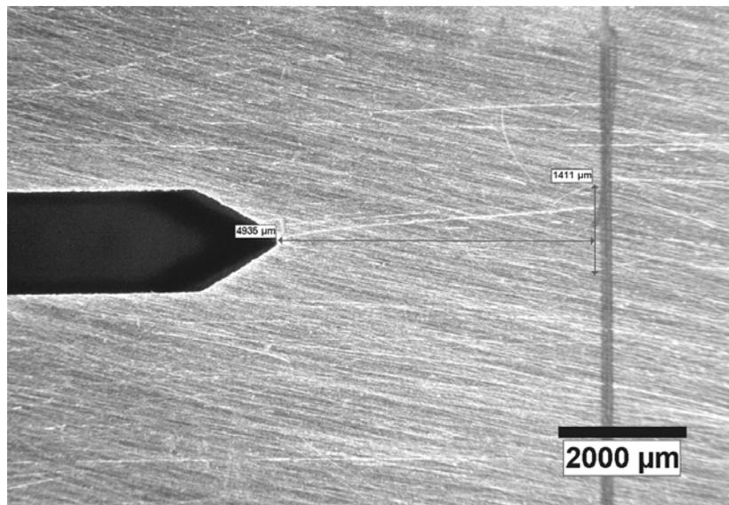
**Figure 20. Precracked DCB samples used in this study. Crack length and sample dimensions are measured to calculate the stress intensity after wedge loading.**
