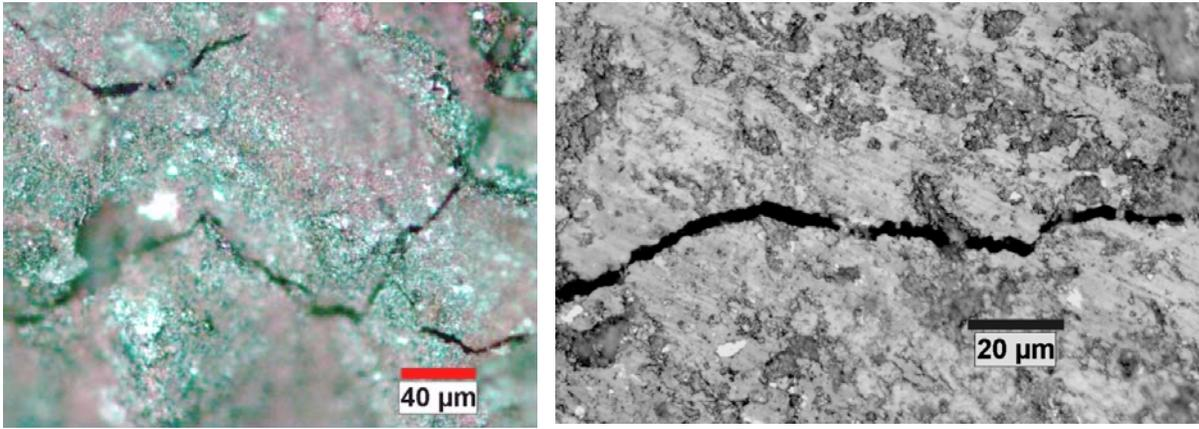
**Figure 2.2** Surface cracks in the mill scale of tested four-point bend samples.
