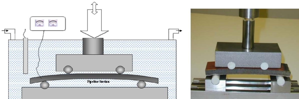
Figure 2.1 Four point bend tests on pipeline sections for SCC initiation under pipeline operating conditions, with and without mill scale.
