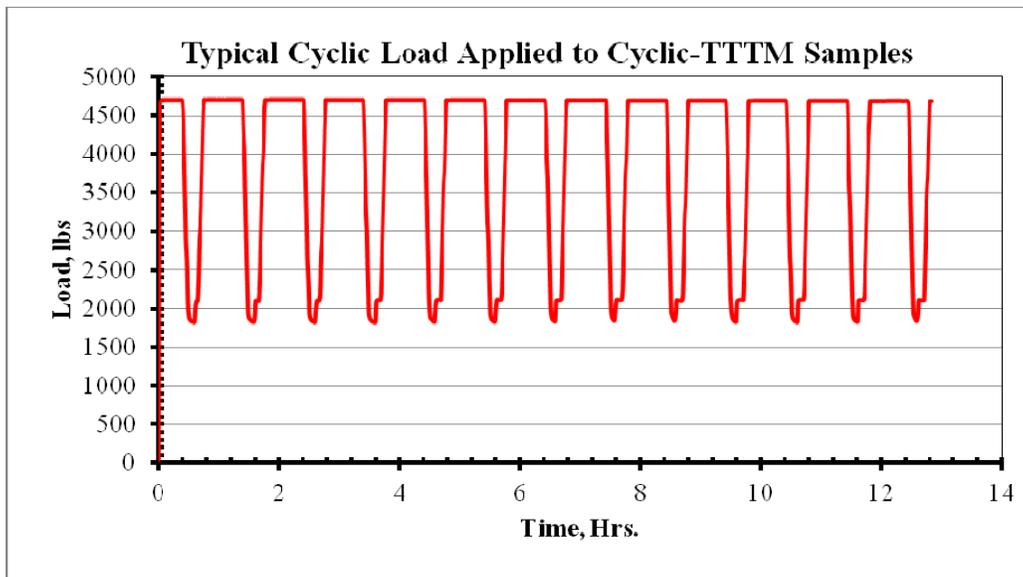
**Figure 1.1 Typical cyclic loading used to test TTTM samples.**
