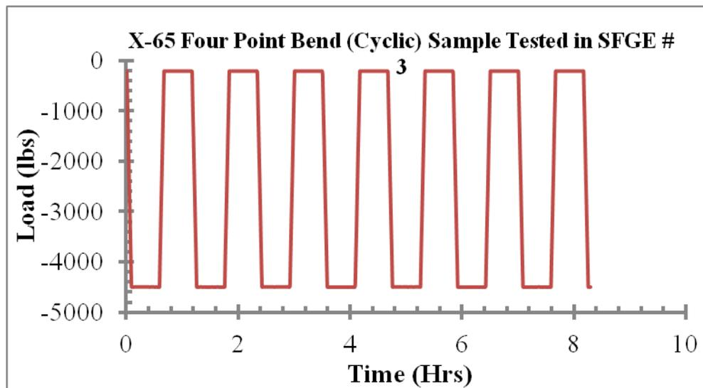
**Figure 2.4.** Showing typical cyclic load/displacement conditions used for cyclic FPB tests in this study. Maximum load was varied for different test samples but the minimum load was kept constant at 200 lbs.
