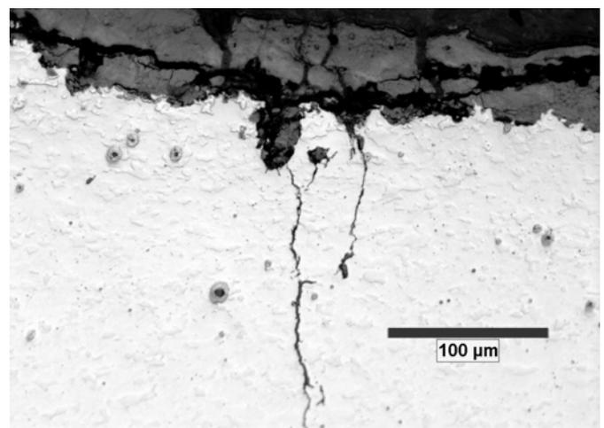
**Figure 2.6. Cyclic Four Point Bend (FPB) tests on pipeline sample (sample#7), with mill scale intact on the inner surface, in SFGE-3 (with 50 ppm Cl). Maximum cyclic load of 6500 lbs. Examination of surface or the sectioned sample did not show any signs of SCC on these samples in SFGE-3**
