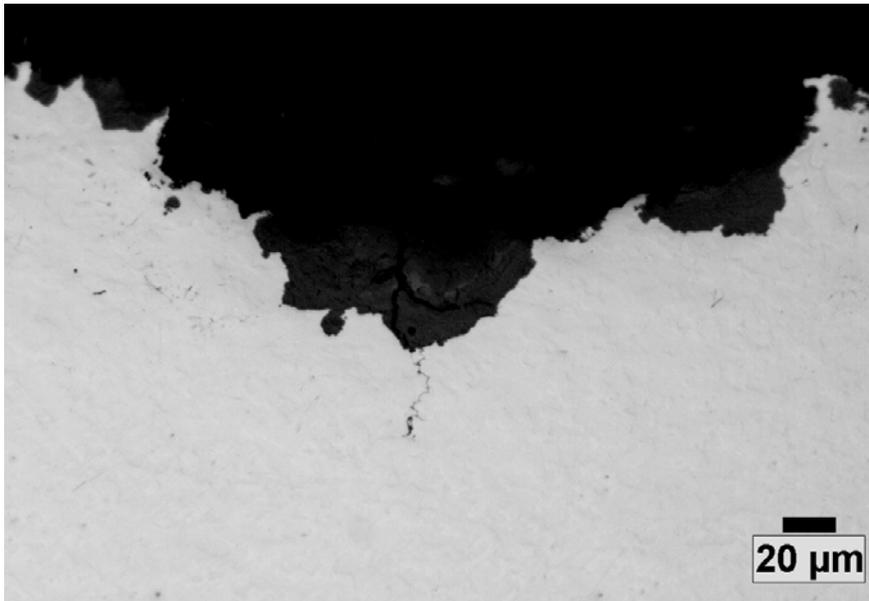
**Figure 2.9.** Cyclic Four Point Bend (FPB) tests on pipeline sample (sample#12) showing a small SCC originated from mill-scaled surface tested in commercial grade fuel grade ethanol (FGE-S) without any addition or modification. Maximum load per cycle was 5500 lbs.
