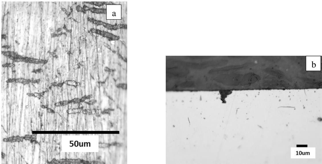
**Figure 4.1. Surface (a) and cross section (b) of SSRT in Cl- containing FGE-WOI**
