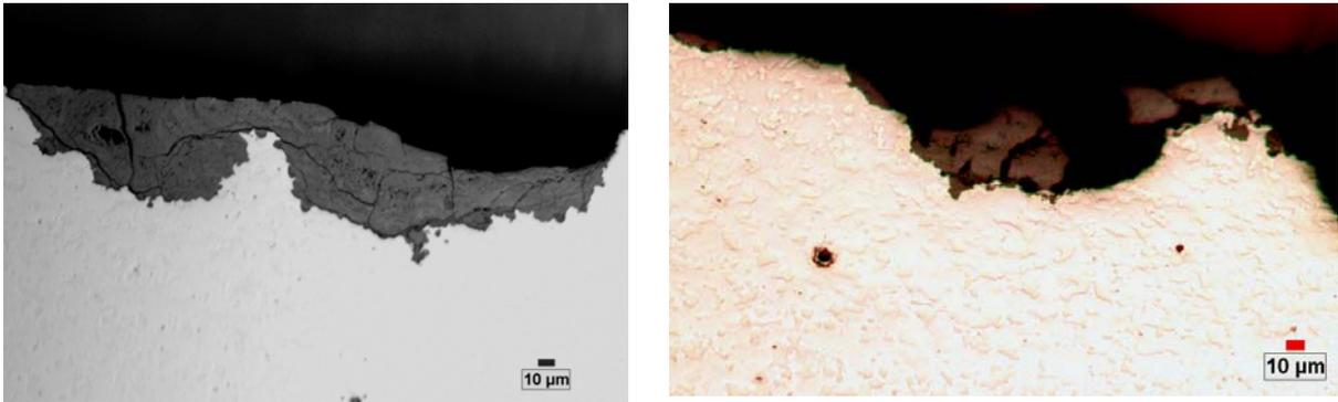
**Figure 2.3** Cross section of FPB sample tested under monotonic strain conditions did not show any crack propagation in the metal for any tested pipeline steel sample.
