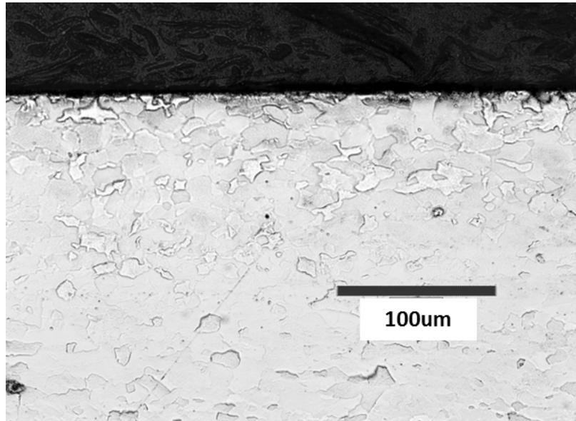
**Figure 4.1. Polished cross section of sample cyclically strained in FGE lot 8**
