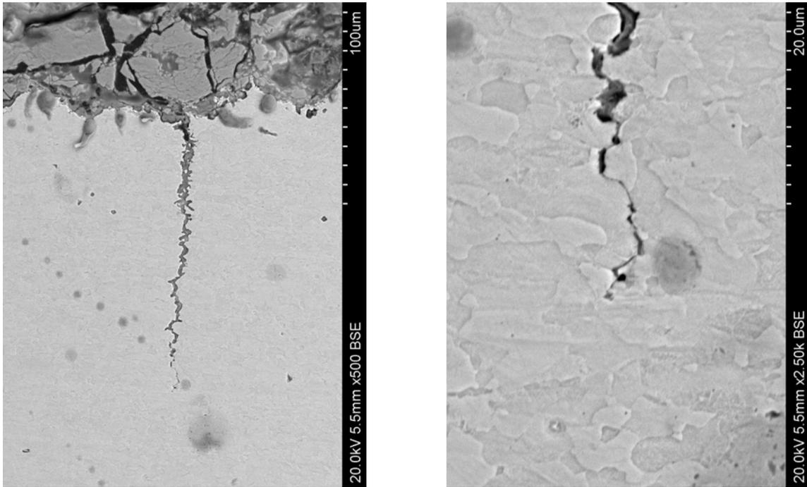
**Figure 2.7. Cyclic Four Point Bend (FPB) tests on pipeline sample (sample#8) tested in commercial grade fuel grade ethanol (FGE) without any addition or modification. Maximum load per cycle was 6500 lbs. Notice that the SCC originated from notches of mill-scaled surface.**
