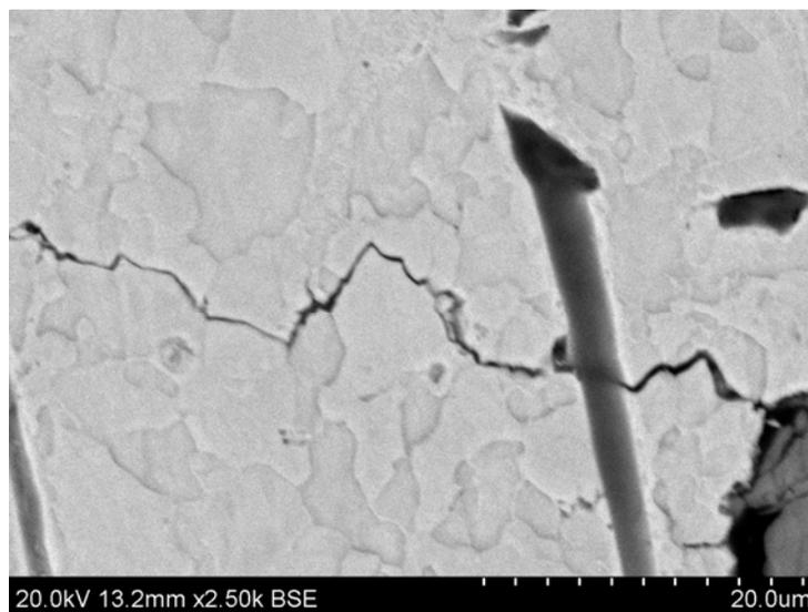
**Figure 2.8. Cyclic Four Point Bend (FPB) tests on pipeline sample (sample#9) tested in FGE-S with 51ppm Cl added, showing a small SCC originated from mill-scaled surface. Maximum load per cycle was 6500 lbs.**
