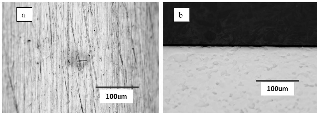
**Figure 4.3. Galvanically coupled sample surface (a) and cross-section (b)**
