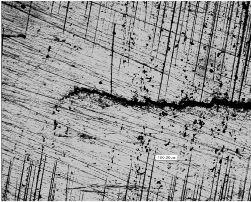
**Figure 21. Crack tip of DCB samples#12 after exposure to SFGE-4 for 12 days.**
