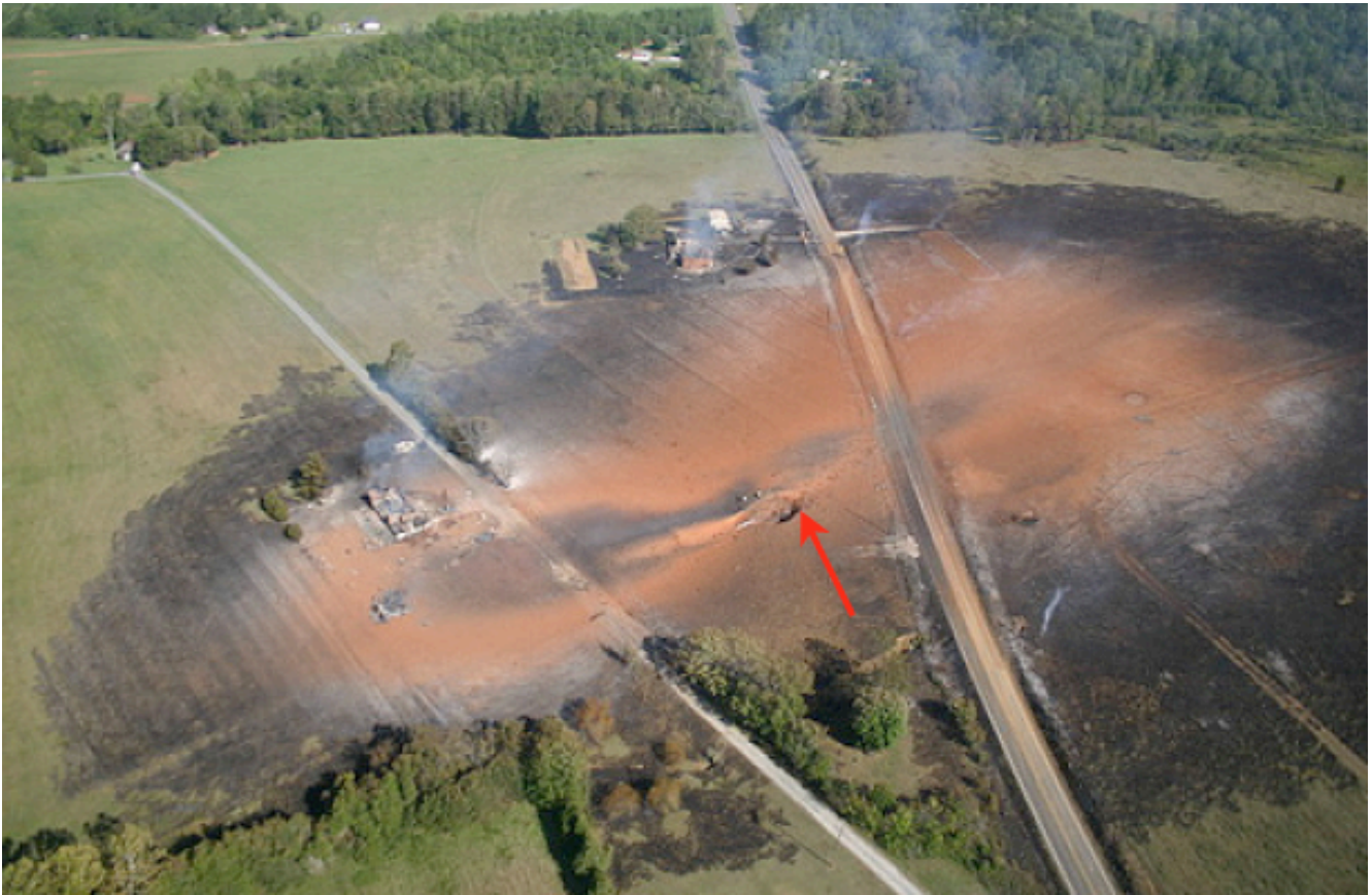
Failure of a natural gas transmission pipeline. Arrow shows point of failure. Note how far from point of failure houses were destroyed
