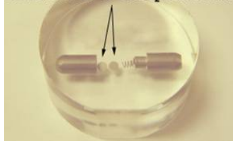
Iridium 191 wafers before activation & encapsulation
