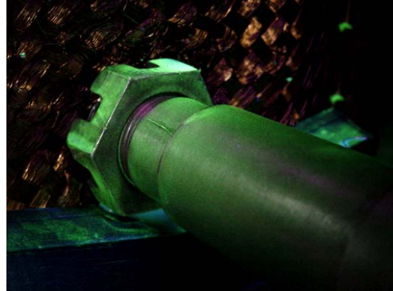
Fluorescent, Wet Particle Method
