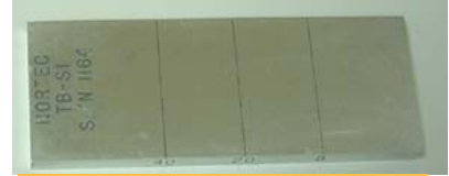
EDM Notches (Crack Simulation)
