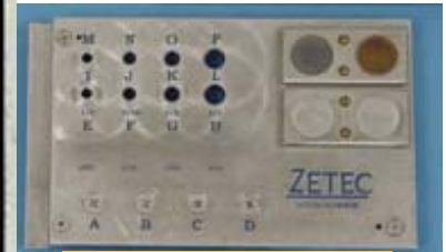
Multipurpose - EDM Notches and Conductivity
