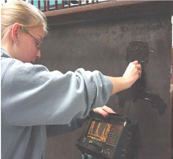
Signal showing multiple back surface echoes in an unflawed area.
