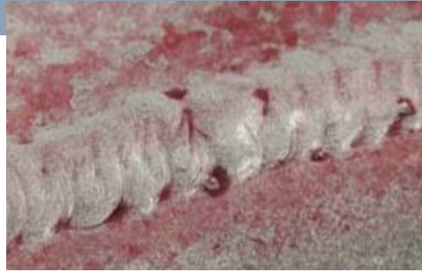
Non-relevant weld geometry indications
