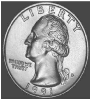
Gray scale image produced using the sound reflected from the front surface of the coin
