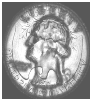
Gray scale image produced using the sound reflected from the back surface of the coin (inspected from "heads" side)
