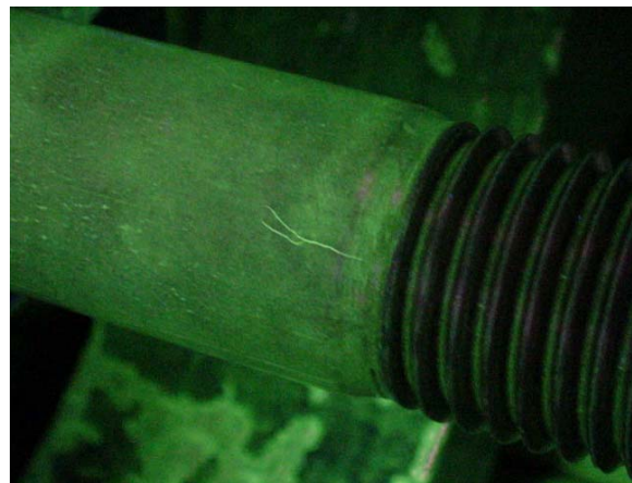
Fluorescent, Wet Particle Method
