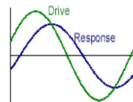
Sinusoidal Excitation and Response
