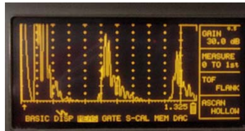
Signal showing multiple back surface echoes in an unflawed area.
