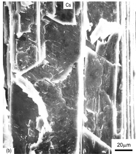
FIGURE 28 - SEM of cleavage-like {0001} fracture surfaces for pure magnesium produced by (a) slow crack growth ( \sim 10^{-3} mm/s) in a NaCl + K 2 CrO 4 solution at 20°C, and (b) rapid crack growth in liquid caesium at 30°C. (Lynch (22,23) )
