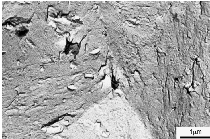
FIGURE 39 - TEM of replica of fracture surface produced by slow crack growth in gaseous hydrogen, showing very fine details on apparently smooth areas shown in the previous figure. (Lynch (19,23) )
