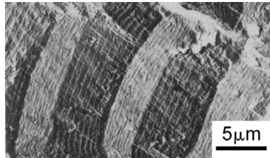
FIGURE 49 - TEM of replica of corrosion fracture surface of a 7075 Al alloy showing abrupt changes from ductile to brittle striations (and vice versa), produced at cathodic and anodic potentials, respectively. (Adapted from Pelloux (127) )
