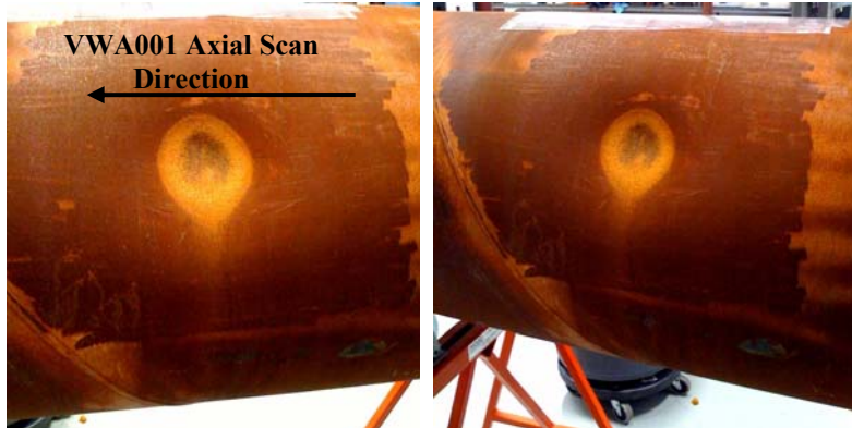
Figure 71. 24-in. diameter pipe section with plain dent. The scan directions for the VWA001 and FA24 MWM-Arrays are indicated.
