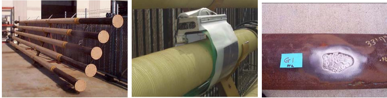
Figure 54. (Left) Simulated pipeline riser sections with embedded corrosion defects. (Center) Photograph of a prototype external scanner. (Right) Photograph of one of the defects.
