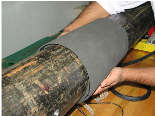
Figure 94. Photograph of the flexible MR-MWM-Array wrapped around a 6-in. diameter pipe section with an extra layer of 0.25-in. thick Neoprene wrapped around the sensor array.
