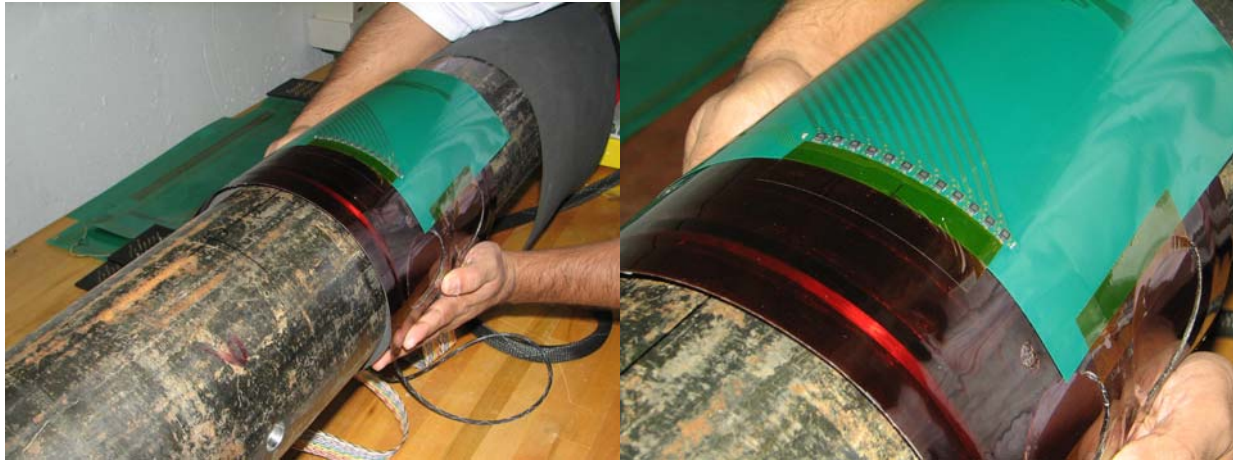
Figure 93. Photographs of the flexible MR-MWM-Array wrapped around a 6-in. diameter pipe section with several 25.4 mm (1-in.) diameter flat-bottom regions machine out of the inner surface.
