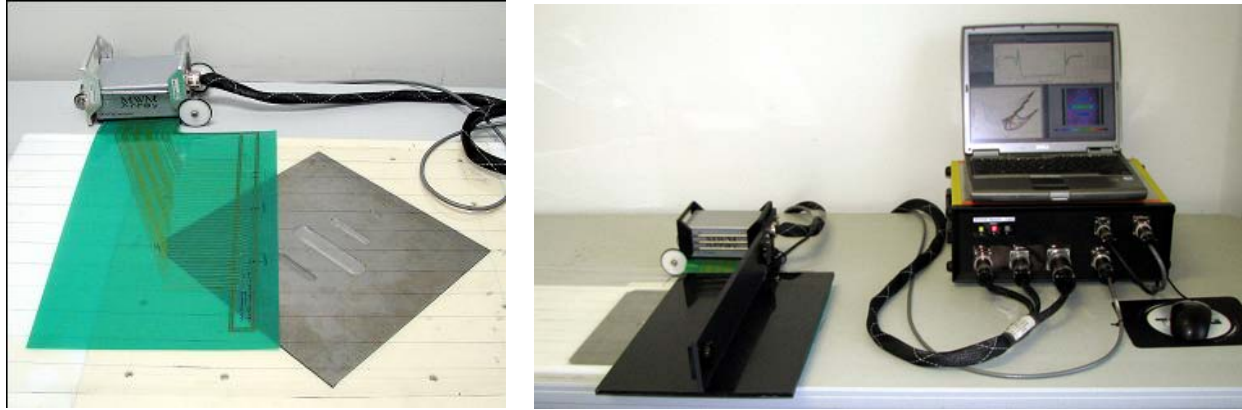
Figure 18. (Left) Photograph of the medium-sized FA122 and a machined steel plate. (Right) Photograph of the instrument and FA122 MWM-Array mounted to a scanning fixture. Note that the FA122 is underneath the plastic scanner fixture.
