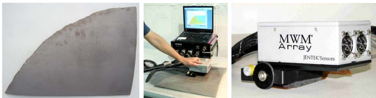
Figure 77. Photographs of (left) the steel pipeline section having clusters of SCC damage, (middle) the scanning setup, and (right) the MWM-Array sensor cart assembly.
