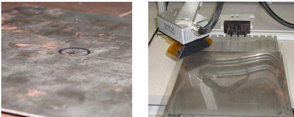
Figure 65. (Left) A dented steel plate. (Right) Plate with an FA24 MWM-Array and a 0.020-in. plastic sheet.
