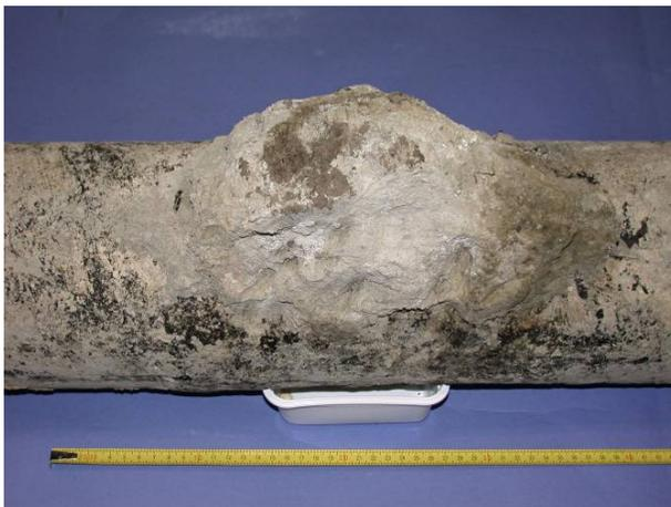
**Figure A5—The pipe with a cap of solidified soil covering the leak.**
