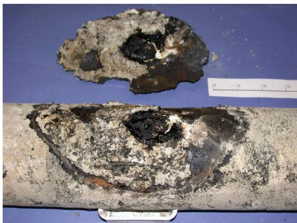
**Figure A6—Cap removed. The leak is located in the center of the black spot.**
