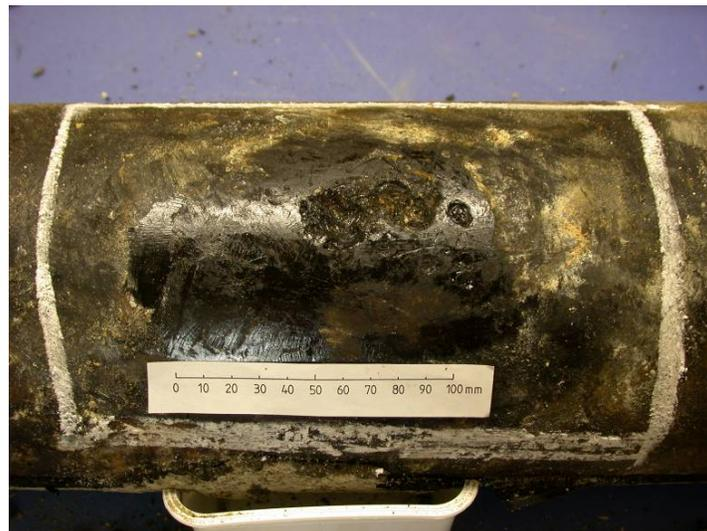
**Figure A8—Pipe surface after removal of the coating.**
