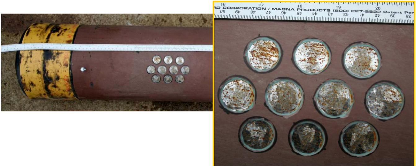
**Figure 55. Examples of distributed defects (10 individual 1 sq. inch defects) on 20 inch (top) and 8 inch (bottom) sections.**
