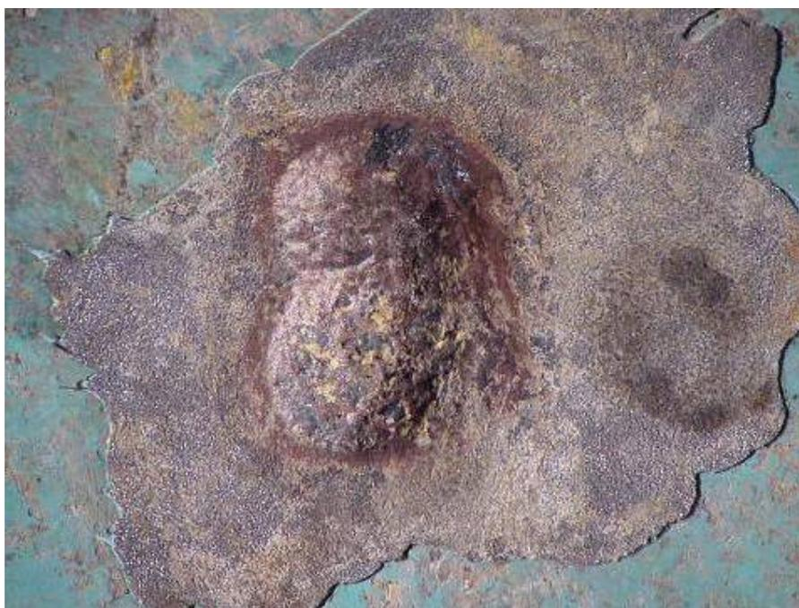
**Figure A1. Location of external through-wall corrosion pit.**
