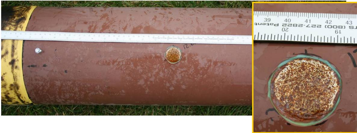
**Figure 54. Examples of centrally positioned 1 sq. inch defects in 8 inch (above) and 20 inch (below) pipeline sections.**
