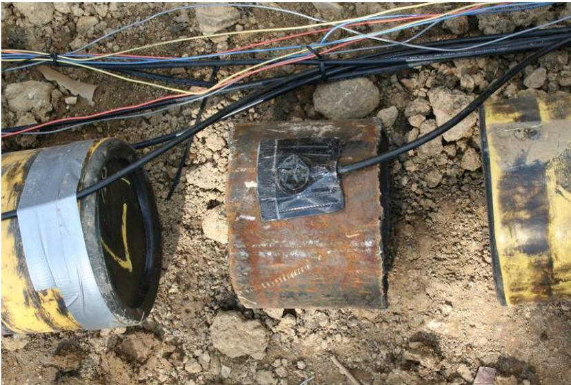
**Figure 62.** Section of bare pipeline inserted between two 8 inch pipeline sections.
