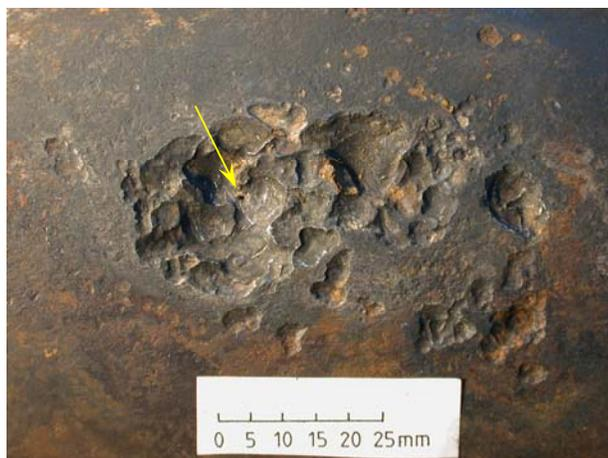
**Figure A9—The corroded area after cleaning. The arrow indicates the leak.**
