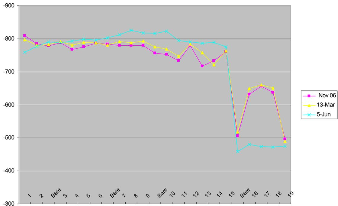
**Figure 66. CIS profile of 8 inch pipeline segments (potentials are in mV against copper/copper sulfate reference electrode).**
