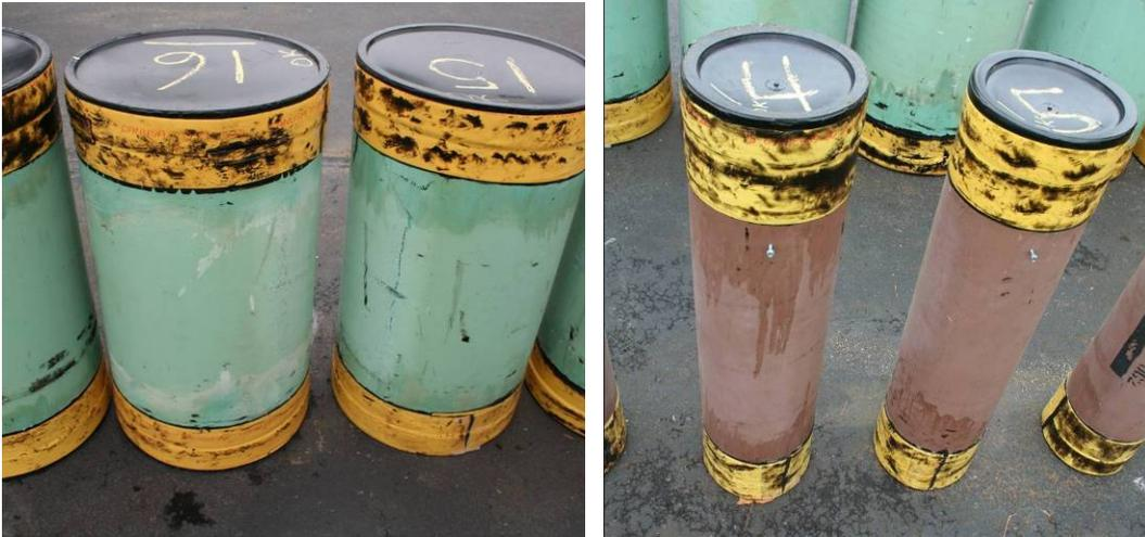
**Figure 50. Pipeline sections (20" diameter, left, 8" diameter, right) with end caps.**
