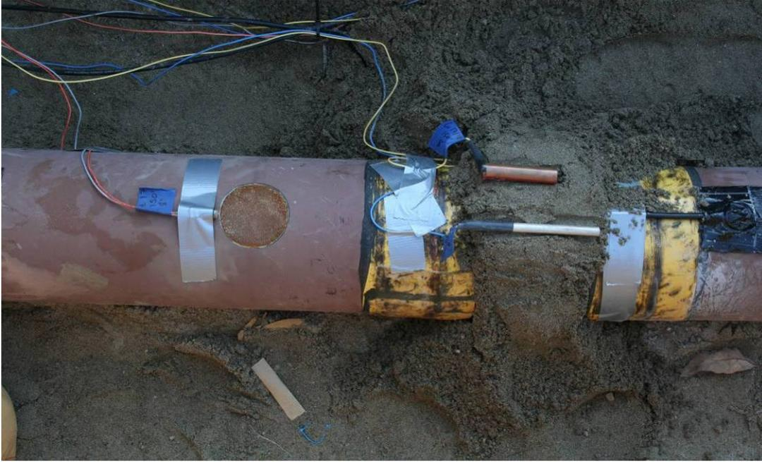
**Figure 59. Reference electrode (left) attached next to an off-center 10 sq. inch defect on 8 inch pipeline section; magnesium electrode (right, lower) and copper electrode (right, upper) placed in between two adjacent pipeline sections.**
