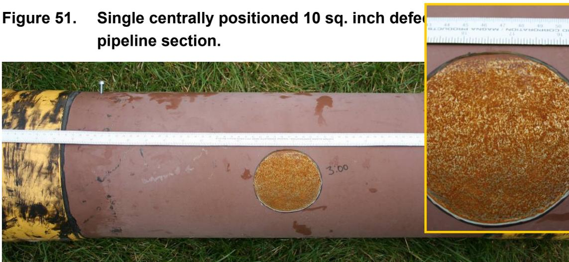
**Figure 52. Single centrally positioned 10 sq. inch defect in 8 inch pipeline section.**
