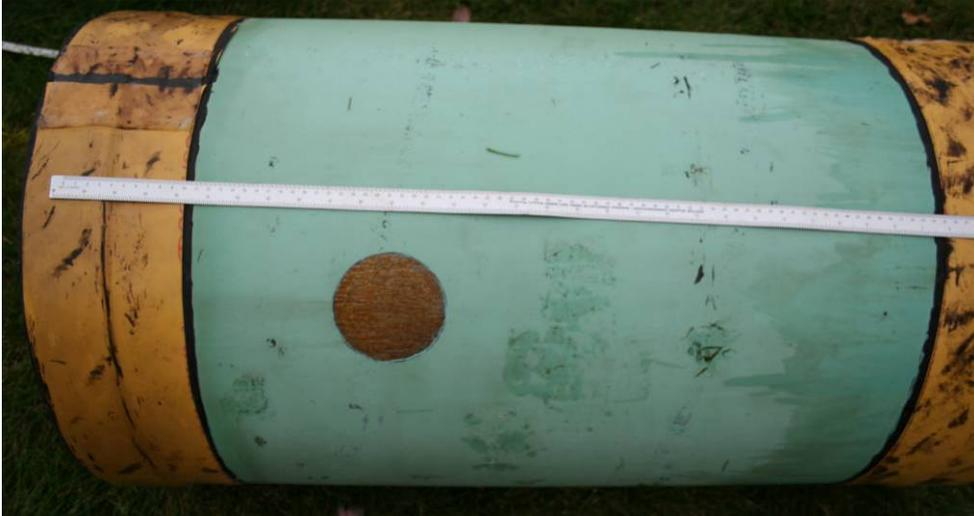
**Figure 53. Examples of offset 10 sq. inch defects in 8 inch (above) and 20 inch (below) pipeline sections.**
