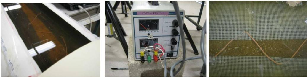
Figure 4. PVC pipe filled with salt water solution (left), power supply used to impress the electric current (middle), and fiberglass mesh wrapped around pipe sample (right)
