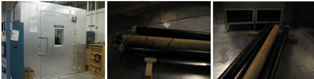
Figure 55. Environmental chamber (left) and three coated pipe samples (middle and right)
