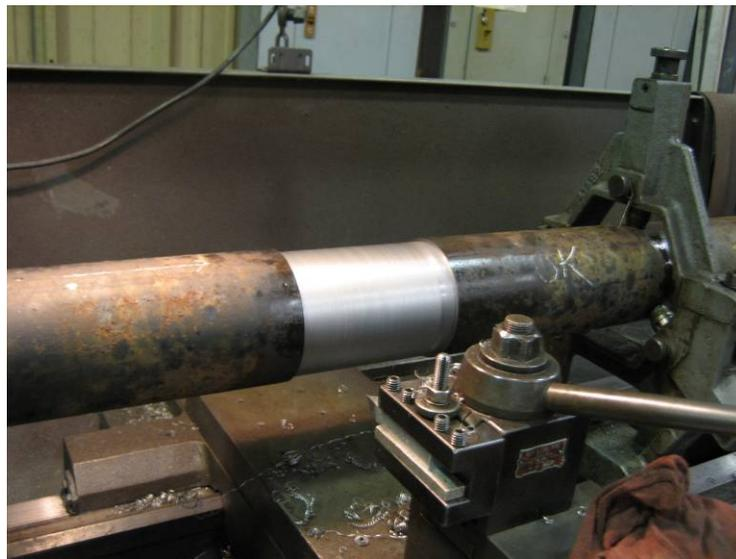
Figure 6. Photo of 4.5-inch-OD, 0.337-inch-wall pipe sample with 6-inch-long machined-in 360-degree notch
