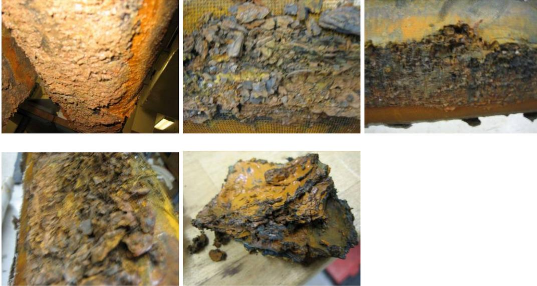
Figure 65. Photos of pipe surface on the bottom side (upper left), on sides (upper middle and right) and a piece of corrosion product (lower right)
