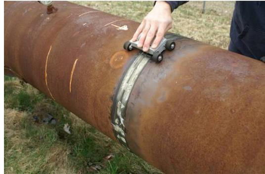
Figure 2. Manual magnetization of the alloy strips
