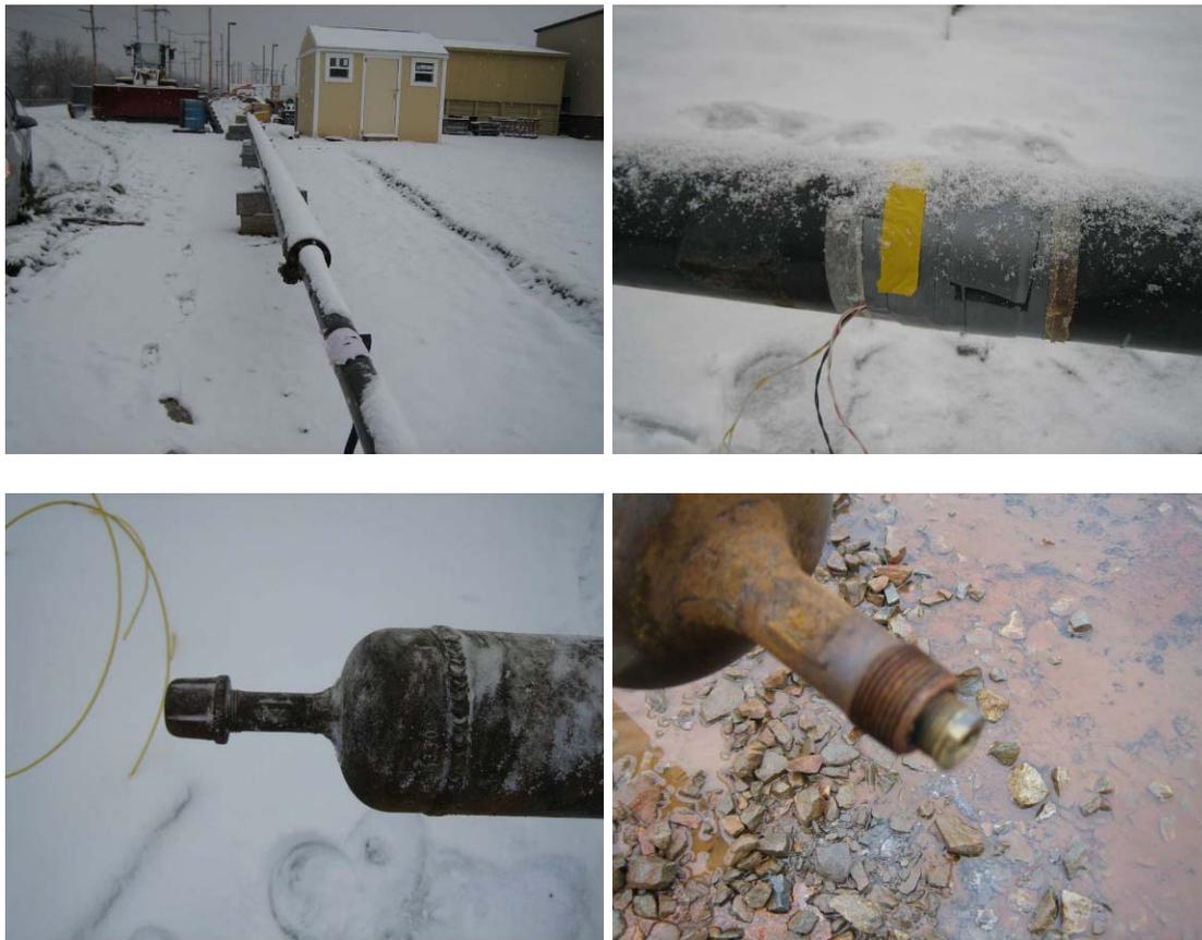
Figure 41. Photos taken during the testing on the 2<sup>nd</sup> mockup: test pipe (top left), MsS probes (top right), and ends of test pipe (bottom)
