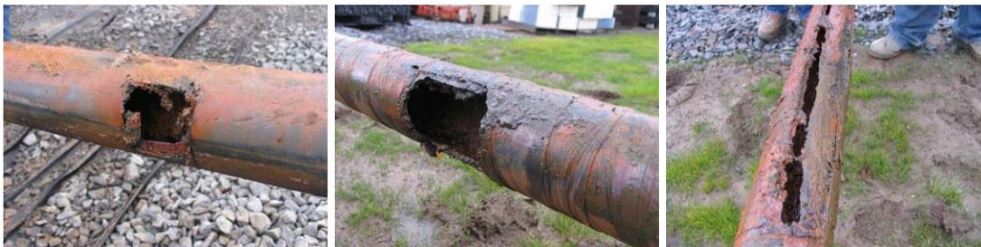
Figure 43. Photos of defects induced in the 1<sup>st</sup> RG&E test pipe: large defects (left two) and 2.8% CSA defect around the weld location (right)
