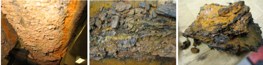
Figure 5. Corrosion products on the pipe surface
