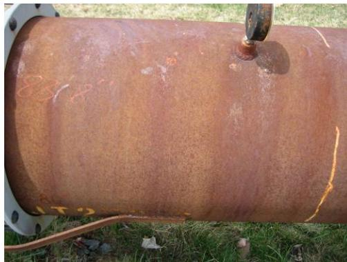
II. Above ground 16-inch-OD coal tar TGF-3 coated pipe with 20-inch casing
