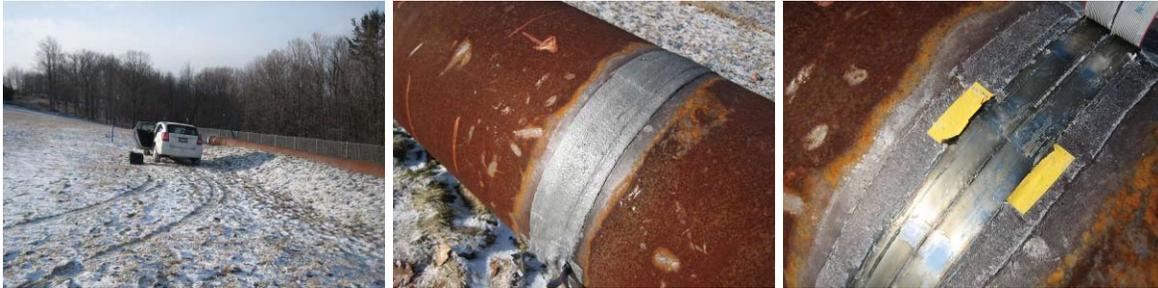
Figure 38. Photos from the 2<sup>nd</sup> SHM testing: scenery of the test bed (left), installed sensors on 20-inch bare pipe (middle), and the iron-cobalt strips exposed after the wax tape and MsS ribbon coils were removed (right)
