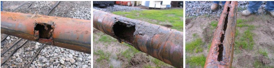
Figure 2. 1<sup>st</sup> RG&E Test Pipe Defects: Large defects (left two) and 2.8% CSA defect at the weld location (right)
