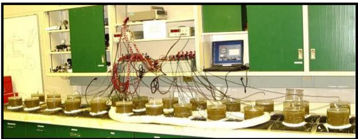
Figure 14a - Cathodic Disbondment Experimental Setup
