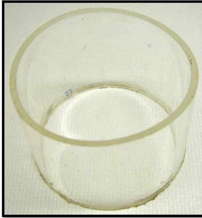
**Figure 11 – Typical HPCC Coated Pipe Sample Section**
