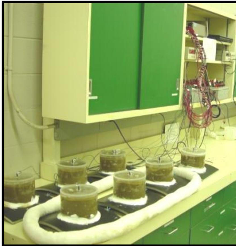
**Figure 13b – Cathodic Disbondment Testing for All Project Samples**
