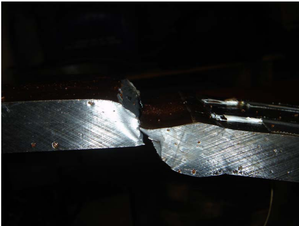
Figure 24 – Failure of Test Sample HLR2
