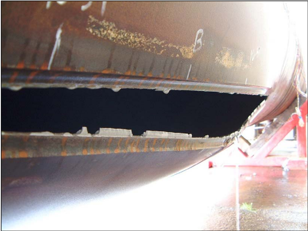
Figure 35 – Test 1 Vessel After Rupture
