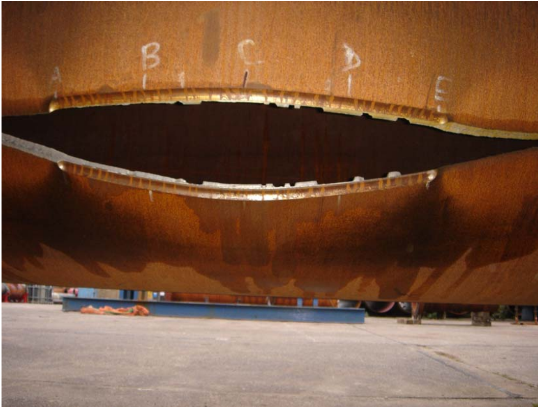
Figure 36 – Test 2 Vessel After Rupture
