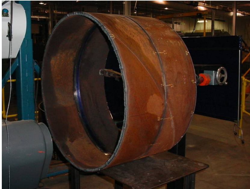
Figure 48. 36-in.-Diameter X80 Pipe Joint
