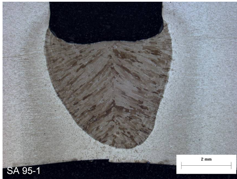
Figure 52. Macrosection of Weld SA-95 Made in X80 Pipe in the Flat Position (Wire feed speed/travel speed ratio: 12.8., travel speed: 0.7 m/min, throat thickness: 4 mm, magnification: 14×.)
