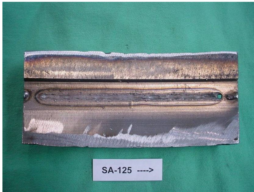
Figure 58. Root Bead Penetration in X80 Pipe Section for Weld SA-125
