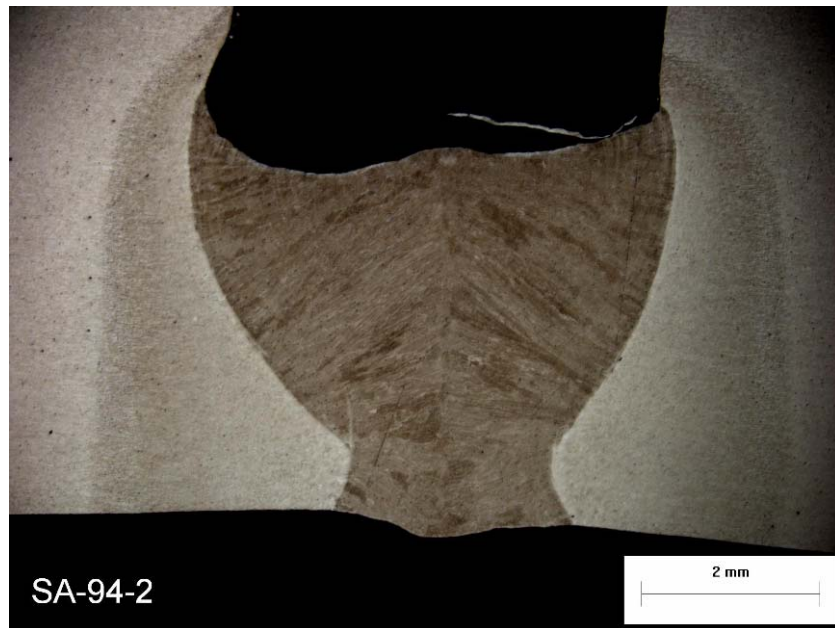
Figure 46. Macrosection of Weld SA-94 Showing a Good Fusion Profile (Wire feed speed/travel speed ratio 11.5, travel speed: 0.7 m/min.)
