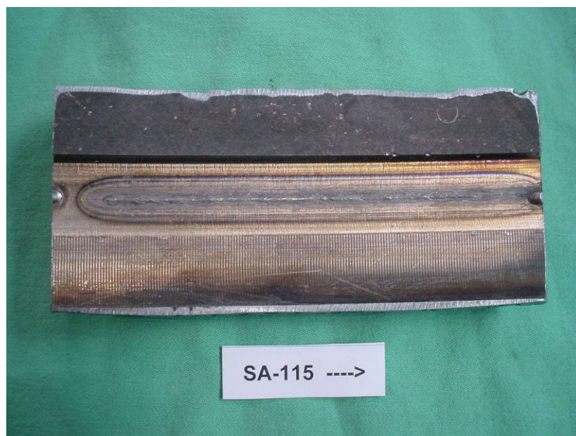
Figure 55. Root Bead Penetration in X80 Pipe Section for Weld SA-115
