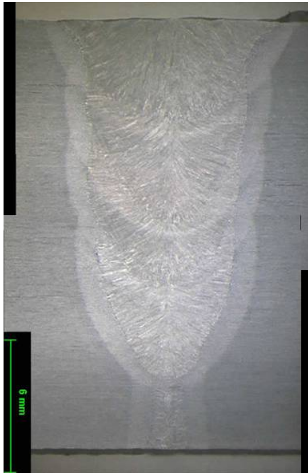
Figure 90. Laser Root Weld Plus Tandem GMAW-P Fill
