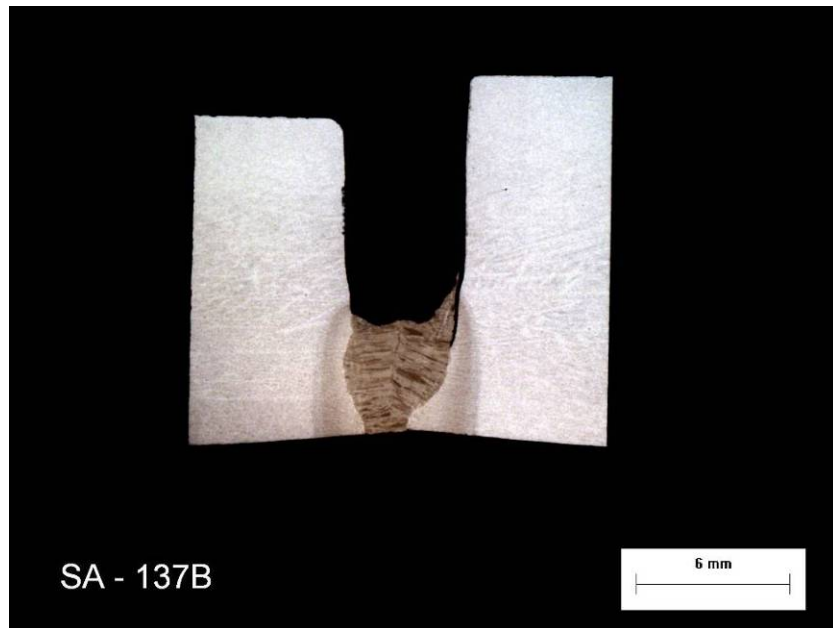
Figure 68. Second Macrosection of Weld SA-137 Made with ER90S-G Wire in X80 Pipe in the Vertical-Down Position Showing Absence of Cracking (Wire feed speed/travel speed ratio: 11.9 , travel speed: 1.2 m/min, throat thickness: 4.6 mm, magnification: 4×.)
