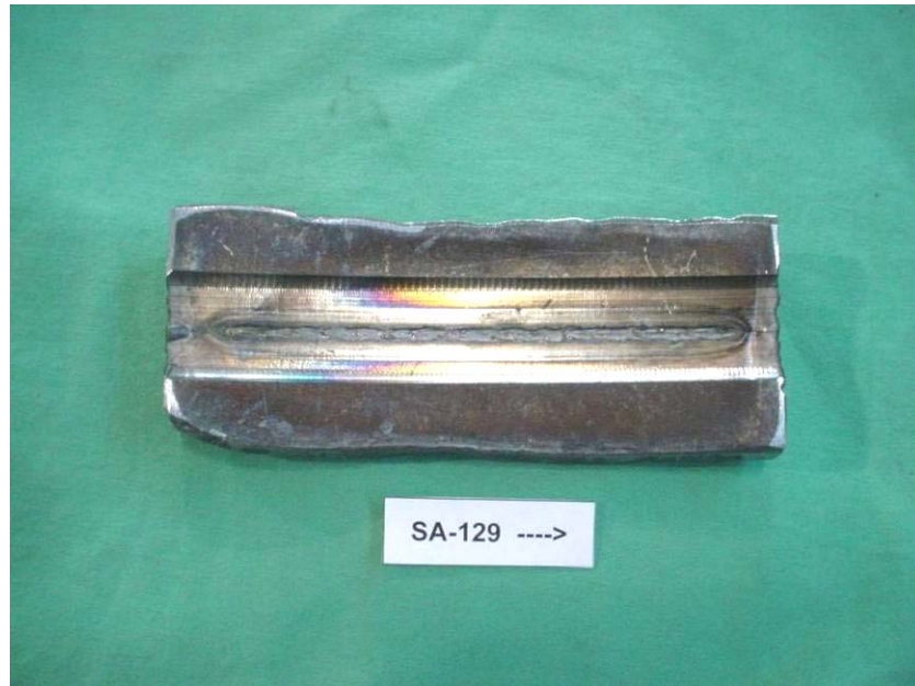
Figure 64. Root Bead Penetration in X80 Pipe Section for Weld SA-129
