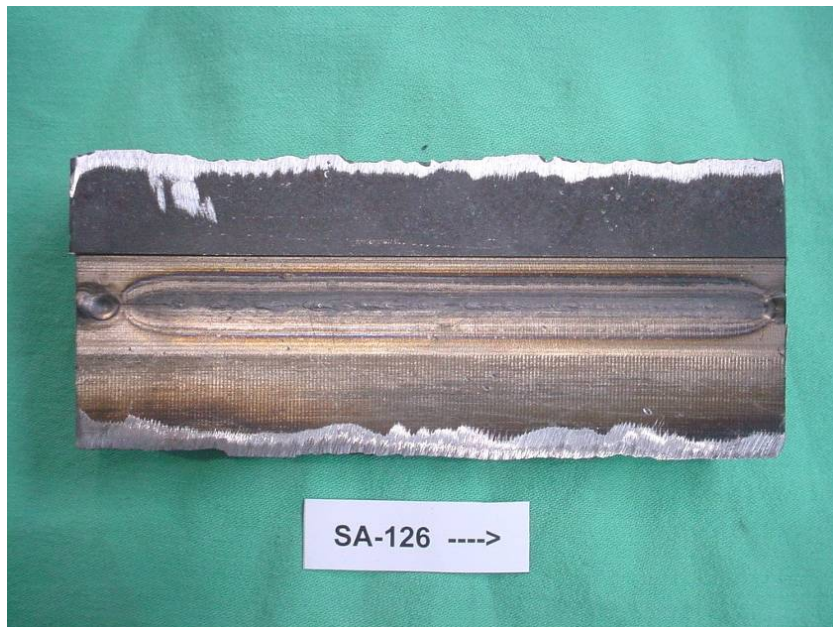
Figure 61. Root Bead Penetration in X80 Pipe Section for Weld SA-126
