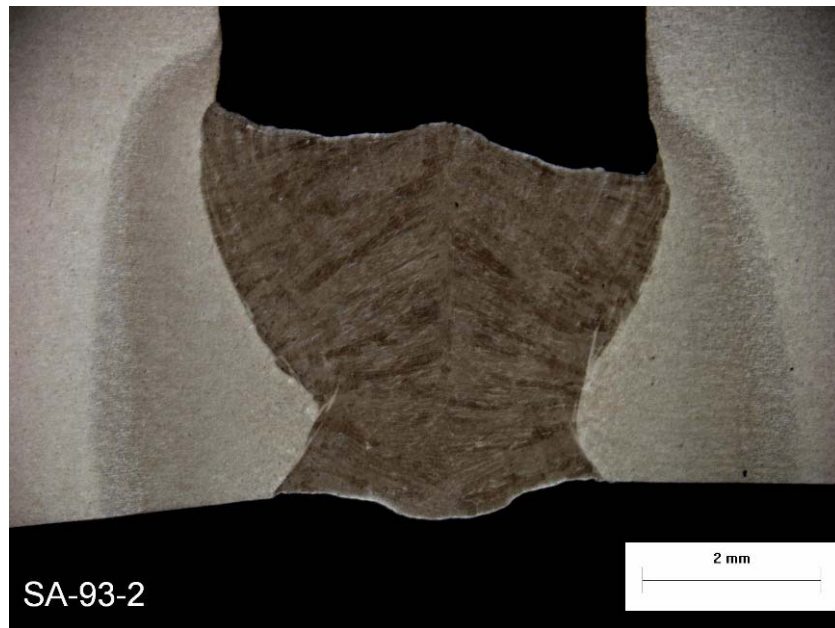
Figure 44. Macrosection of Weld SA-93 Showing a Good Fusion Profile (Wire feed speed/travel speed ratio 12.3, throat thickness: 4 mm, travel speed: 0.7 m/min.)
