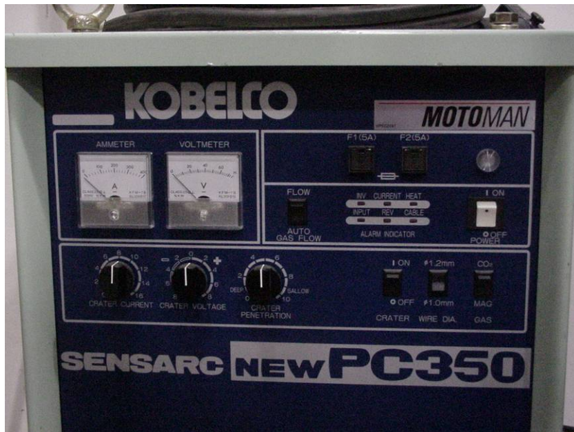
Figure 5. Motoman/Kobelco PC 350 GMAW-VP Power Source Front Panel
