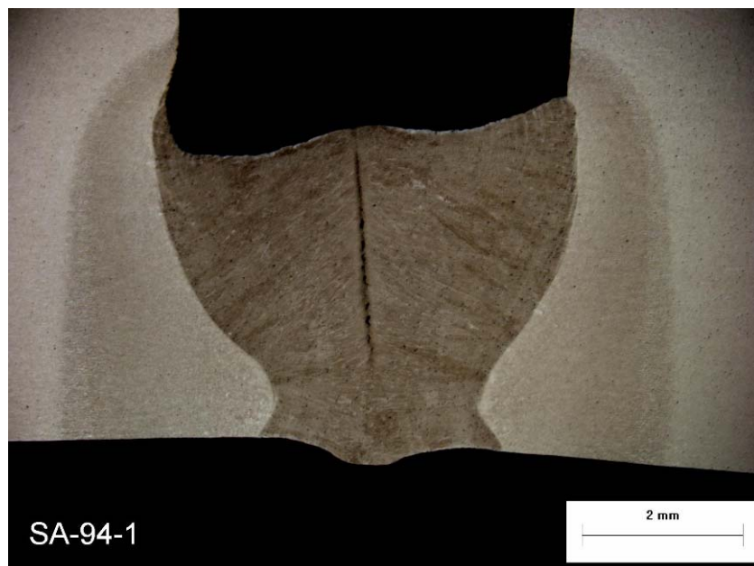
Figure 45. Macrosection of Weld SA-94 Showing Subsurface Centerline Hot Crack (Wire feed speed/travel speed ratio: 1.5, travel speed: 0.7 m/min.)
