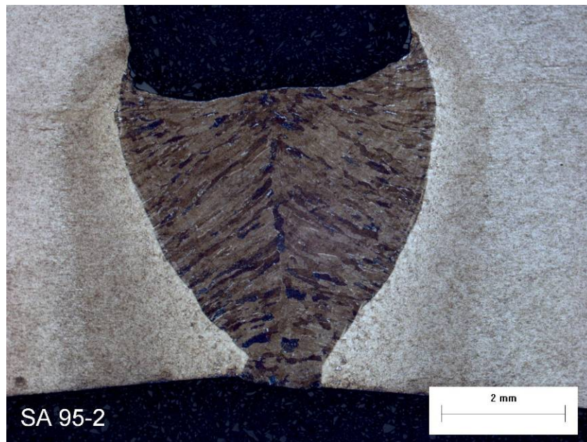
Figure 51. Macrosection of Weld SA-95 Made in X80 Pipe in the Flat Position (Wire feed speed/travel speed ratio: 12.8, travel speed: 0.7 m/min, through thickness: 5 mm, magnification: 14×.)
