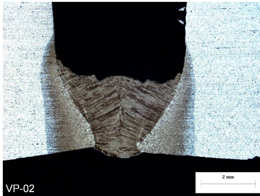
Figure 20. Macrosection of Weld VP-02 Made in the Flat Position using GMAW-VP
