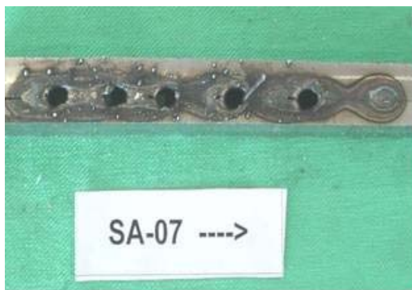
Figure 31. View of Typical Penetration Bead Profiles in Welds SA-7 and SA-8
