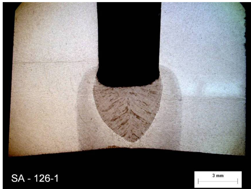
Figure 63. Macrosection of Weld SA-126 Made with ER80S-D2 Wire in X80 Pipe in the Vertical-Down Position (Wire feed speed/travel speed ratio: 12.9, travel speed: 0.7 m/min, throat thickness: 4.2 mm, magnification: 7×.)
