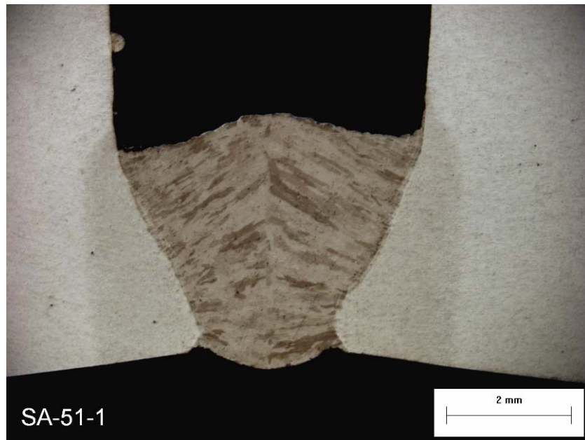
Figure 38. Macrosection of Weld SA-51 Showing a Good Fusion Profile (Wire feed speed/travel speed ratio: 9.1, travel speed: 1.5 m/min, throat thickness: 4 mm, magnification: 14×.)
