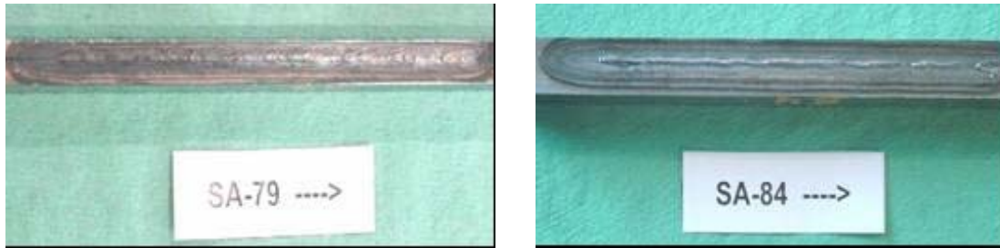
Figure 40. View of Typical Penetration Bead Profiles in Welds SA-79 and SA-84, and Macrosection of Weld SA-79 Showing Buried Solidification Crack
