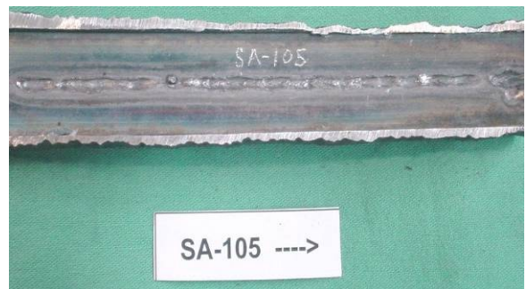
Figure 53. View of Penetration Bead Profiles in Welds SA-100 and SA-105
