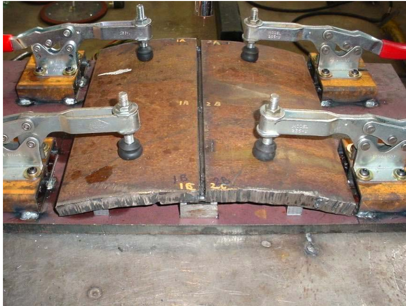
Figure 3. Tacking Fixture Loaded with X80 Pipe Sections for Plate-Type Welding Procedure Development
