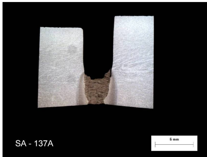
Figure 67. Macrosection of Weld SA-137 Made with ER90S-G Wire in X80 Pipe in the Vertical-Down Position Showing Absence of Cracking (Wire feed speed/travel speed ratio: 11.9, travel speed: 1.2 m/min, throat thickness: 4.1 mm, magnification: 4×.)
