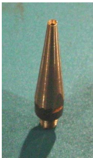
Figure 12. Tapered Contact Tip Machined for Narrow Gap Pipe Joint Access
