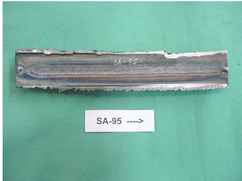
Figure 50. Root Bead Penetration in X80 Pipe Section for Weld SA-95
