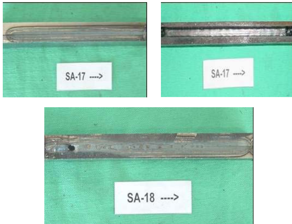
Figure 33. View of Typical Penetration Bead Profiles in Welds SA-17 and SA-18
