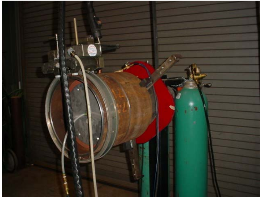
Figure 8. General View of the Pipeline Tractor and Track Mounted on a Development Pipe Girth Weld Test Piece (Gas backing was used here, but discontinued for work on GMAW-RE.)
