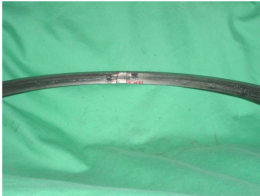
Figure 29. Spin Arc Weld W21 – Inside View of Penetration Bead
