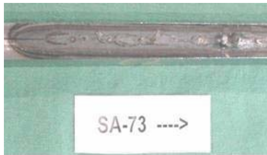
Figure 39. View of Typical Penetration Bead Profiles in Welds SA-72 and SA-73
