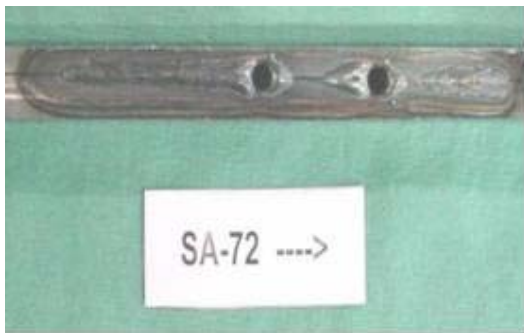
Figure 39. View of Typical Penetration Bead Profiles in Welds SA-72 and SA-73
