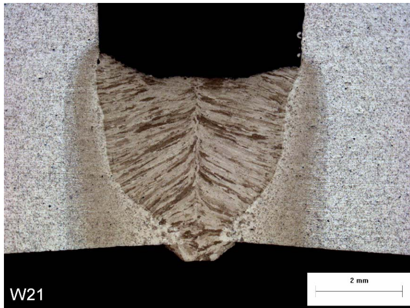
Figure 30. Macrosection of Spin Arc Weld W21 Weld 4.2-mm Throat Thickness
