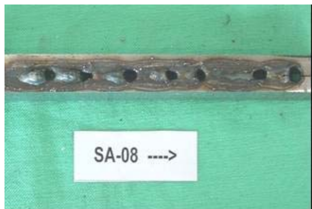
Figure 31. View of Typical Penetration Bead Profiles in Welds SA-7 and SA-8
