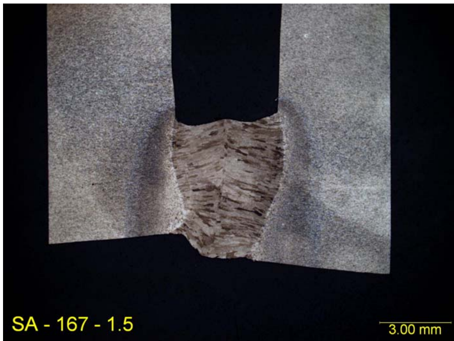
Figure 75. Macrosection Showing Fusion Profile and Root Bead Profile with 1.5 mm High/Low Root Mismatch
