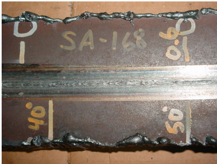
Figure 72. Root Bead Profile for 0.5 mm High/Low Root Mismatch
