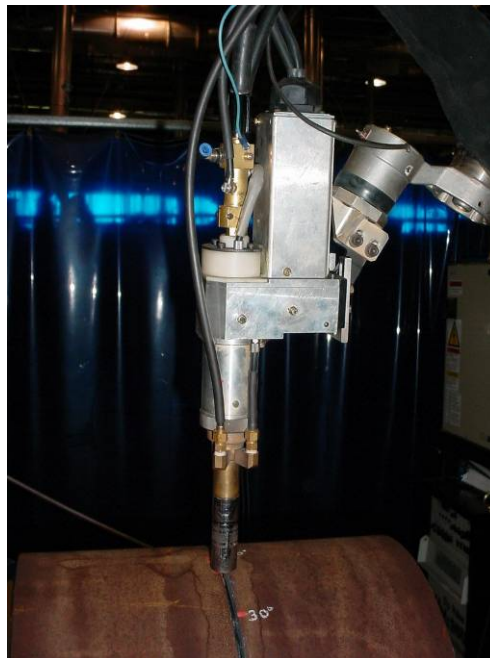
Figure 11. Spin Arc Torch Mounted on Robot Arm
