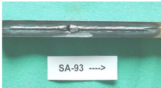
Figure 42. View of Penetration Bead Profiles for Weld SA-93
