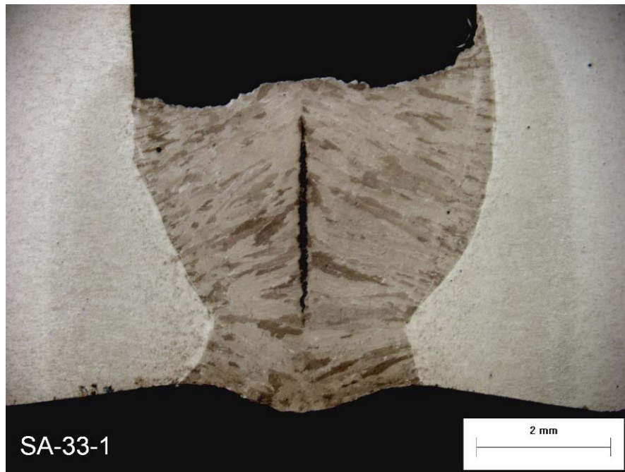
Figure 36. Macrosection of Weld SA-33 Showing Subsurface Centerline Hot Crack (Wire feed speed/travel speed ratio: 15.1, throat thickness: 4.7 mm, travel speed: 0.7 m/min, magnification: 14×.)
