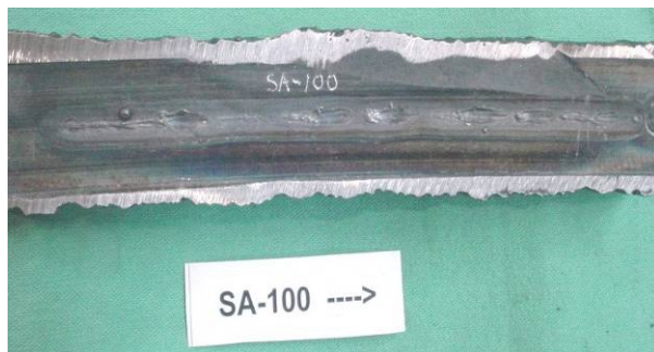
Figure 53. View of Penetration Bead Profiles in Welds SA-100 and SA-105
