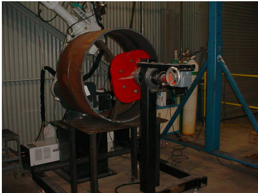
Figure 47. 36-in.-Diameter X80 Pipe Joint Setup for Robotic Spin Arc GMAW-RE
