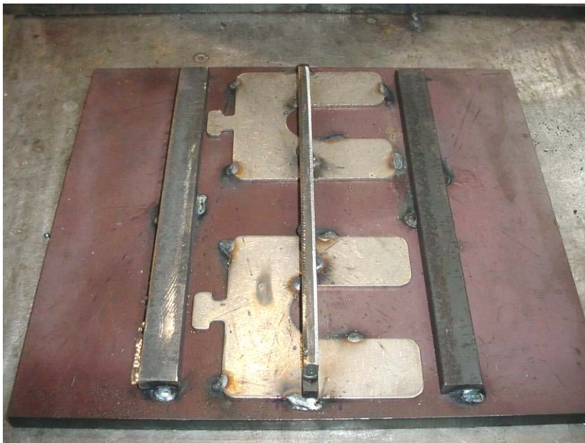
Figure 4. Tacking Fixture for X80 Plate Butt Joints
