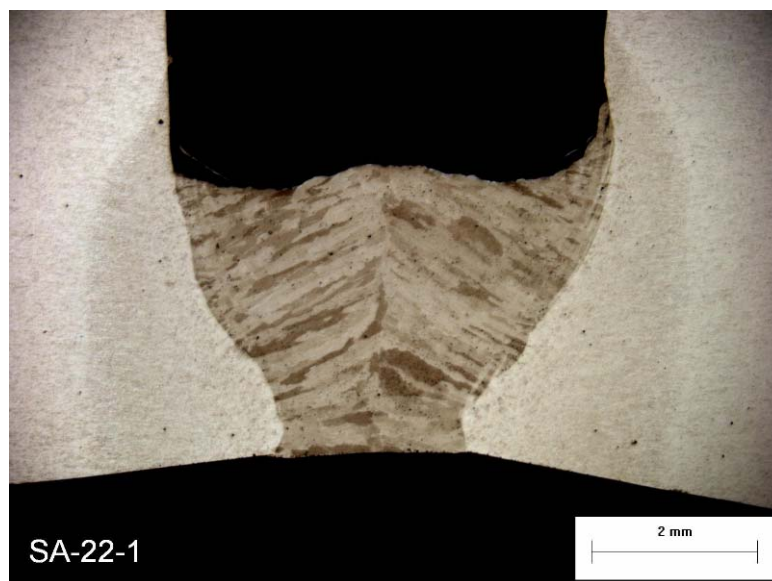
Figure 35. Macrosection of Weld SA-22 (Wire feed speed/travel speed ratio: 11.1, throat thickness: 3.5 mm, travel speed: 0.8 m/min.)
