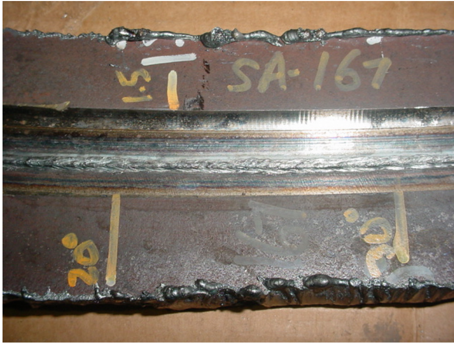
Figure 74. Root Bead Profile for 1.5 mm High/Low Root Mismatch
