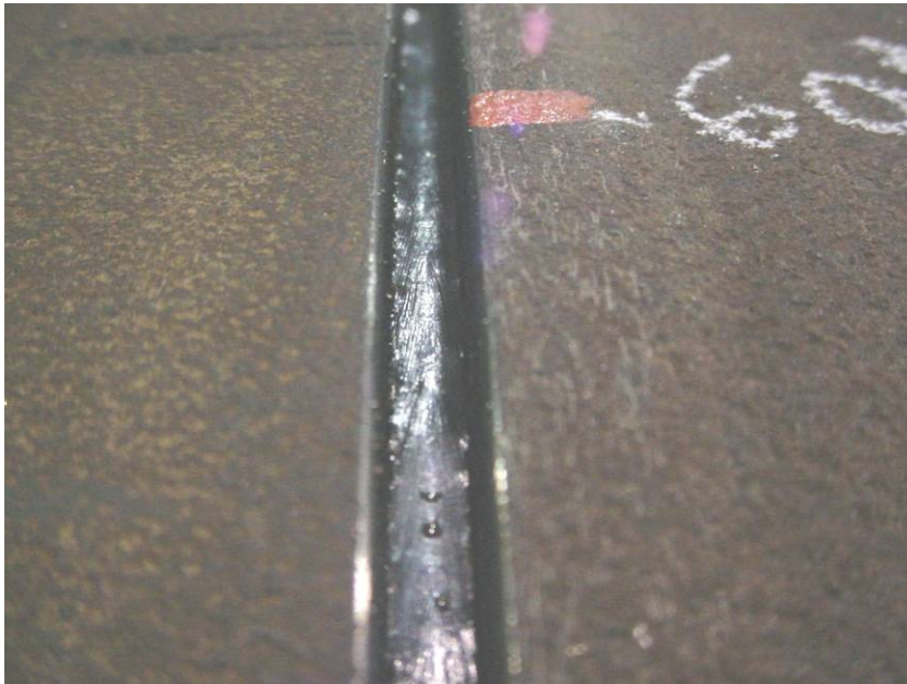
Figure 23. External View of Spin Arc GMAW Root Pass Weld W13 about 60 Degrees from TDC
