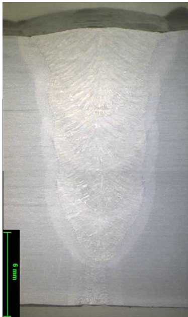
Figure 3. L3 Macro (No visible defects, flat root bead.)
