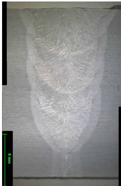
Figure 4. L4 Macro (No visible defects, flat root bead.)
