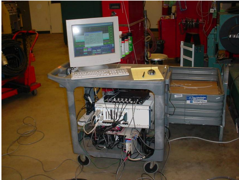
Figure 7. PXI Industrial Computer System Controls Spin Arc and Data Acquisition
