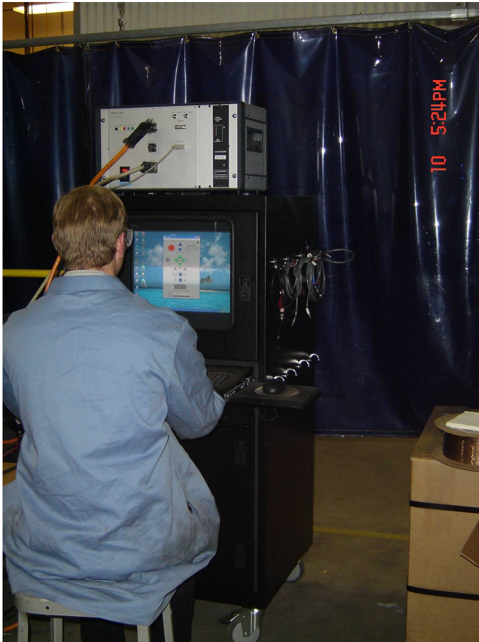
Figure 14. Operator at the Industrial Control Cabinet Housing the Integrated Hardware and Software for Process Control
