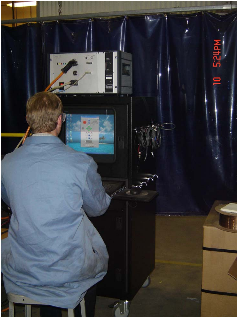
Figure 14. Operator at the Industrial Control Cabinet Housing the Integrated Hardware and Software for Process Control and DAQ
