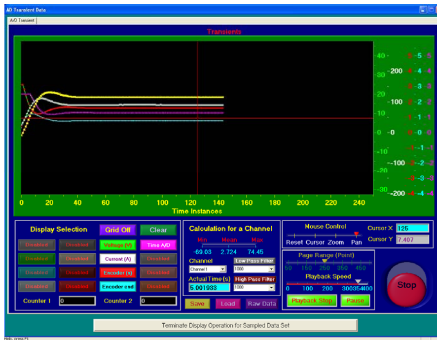
Figure 16. Intellicontrol Software Interface Module During Data Acquisition of Welding Parameters and Spin Arc Control
