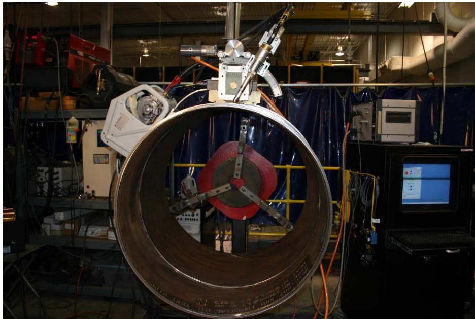
Figure 2. Front View of Torch Travel Angle Hardware Added to Standard STX Bug
