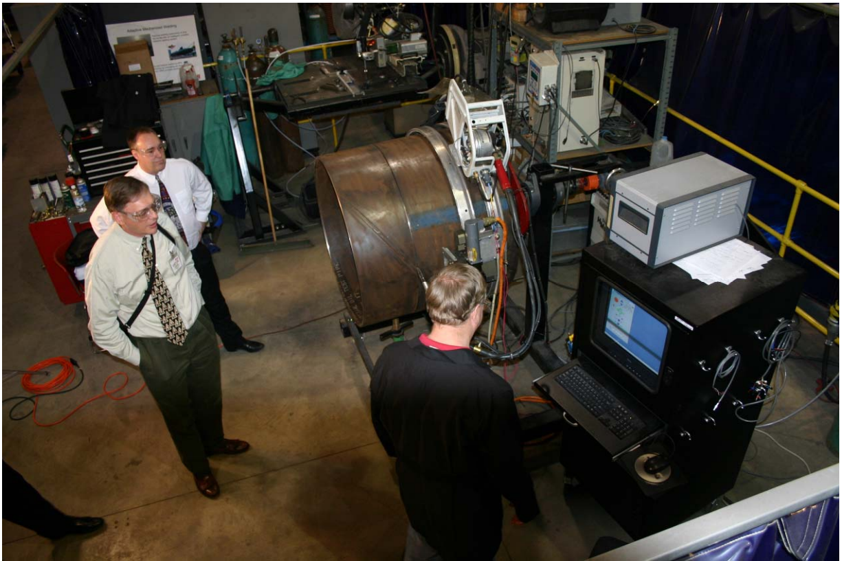
Figure 14. Demo Dry Run Showing Twin Tractor Relative Position when Welding is in the Vertical-Down Position
