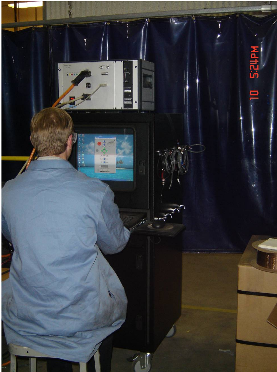
Figure 4. Operator at the Industrial Control Cabinet Housing the integrated Hardware and Software for Process Control
