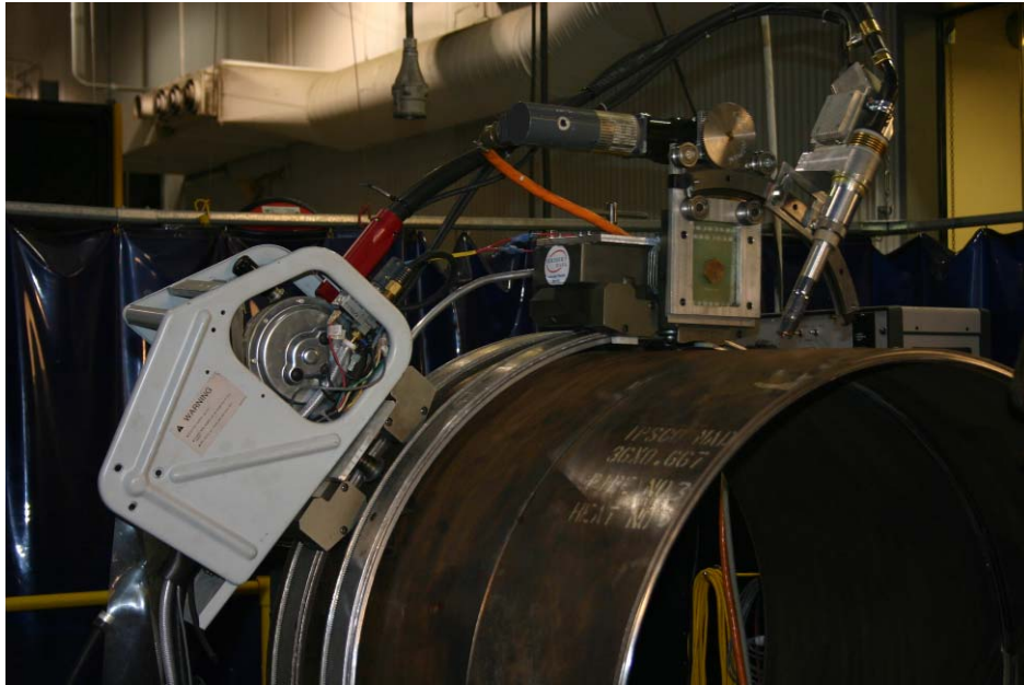
Figure 1. Torch Travel Angle Hardware Added to Standard STX Bug
