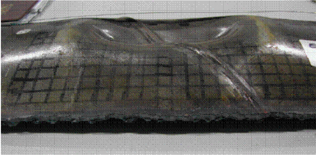
Figure 42: Side view of sample P43 – showing the interesting geometry that leads to the MFL signals in Figures 40 and 41.
