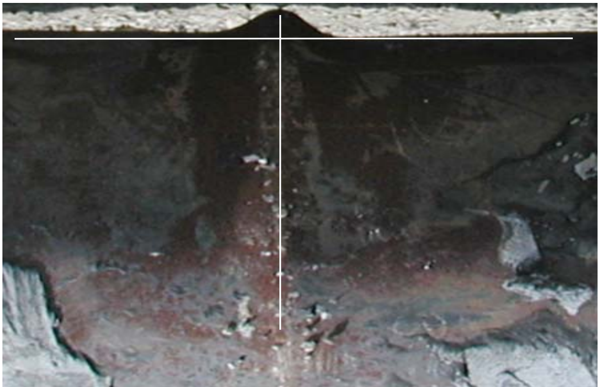
b) wrinkle that is asymmetric lengthwise along its crown
