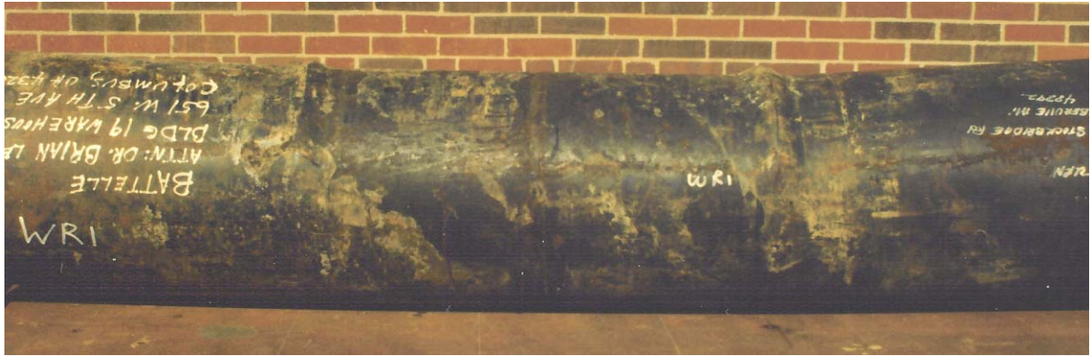
a) bend with angle equal to \sim 4 degrees comprises two wrinkles either side of a girth weld
