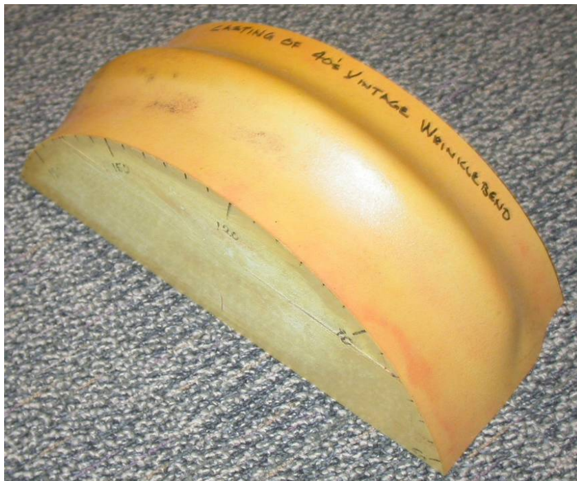
Figure B4. "Cast" of a wrinkle-bend running ~160-degrees around the circumference
