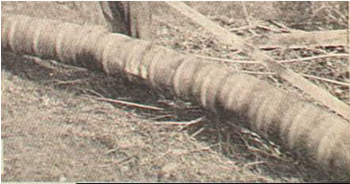
Figure A8. Typical bend produced with the A-Frame fixture shown in Figure 7.
