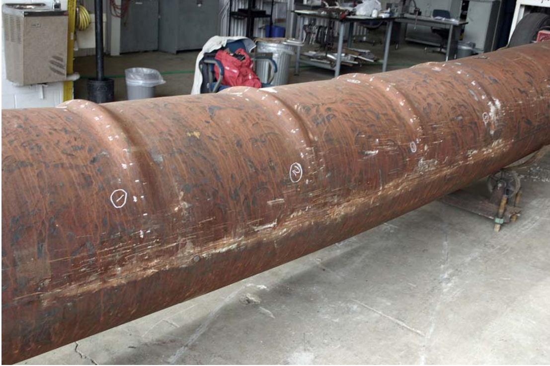
a) overview of segment E and wrinklebends 1 (closest) through 4 (furthest)
