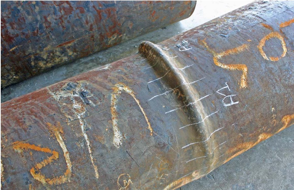
b) views of one of the more severe appearing wrinkles in segment A
