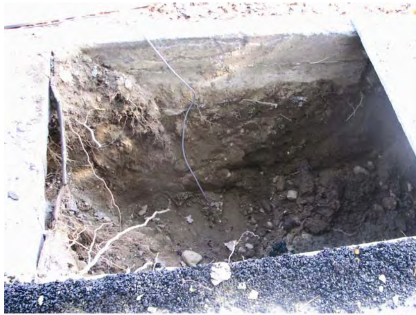
Figure 46. One PIGPEN sensors was buried approximately 5 feet below grade in the trench shown. A second sensor was located on the sidewalk in a box of soil.
