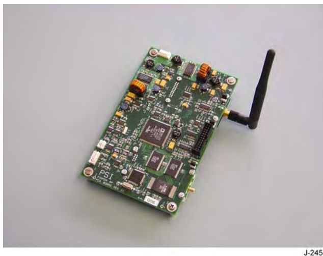
Figure 112. PIGPEN AP Power and Communications board. Top view.
