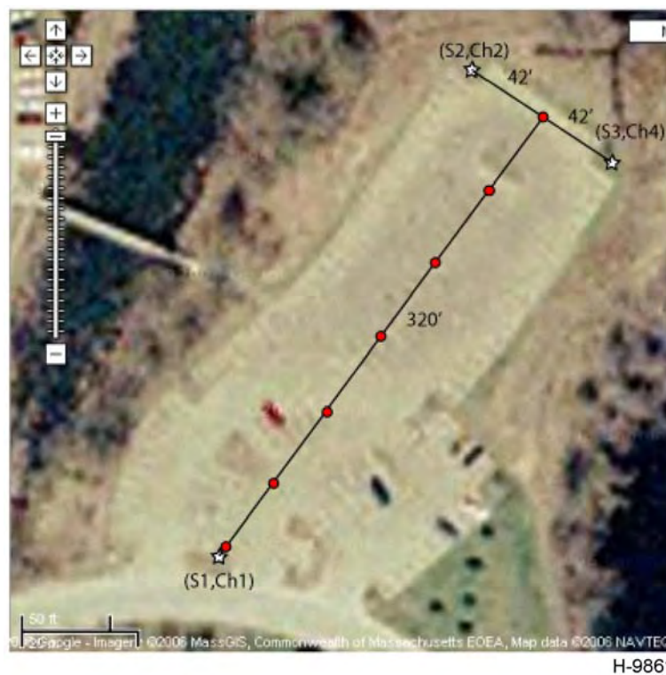
Figure 34. June 2006 triangulation test configuration.
