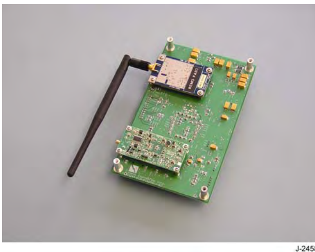
Figure 113. PIGPEN AP Power and Communications board. Bottom view.
