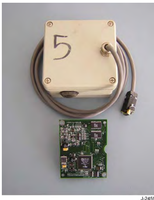
Figure 114. Sensor chassis and DSP board before installation in the chassis.
