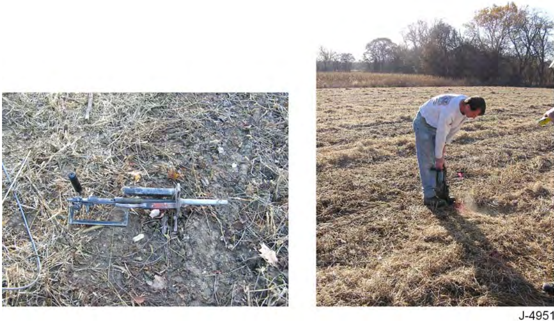
Figure 52. The downhole gun close-up (left) and in operation (right).
