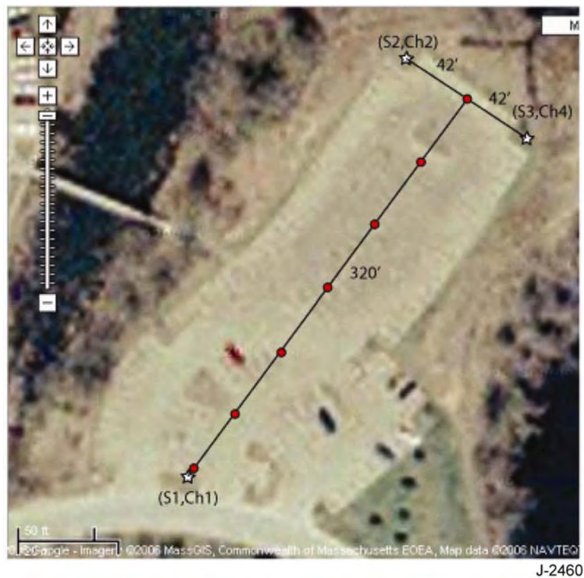
Figure 39. Sensor and threat locations for the 17 August field test.
