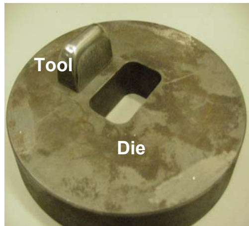
Figure 5. Tool and die used for creating elongated dents in the present study. Note that the tool and die are completely separate items and in this photo, which shows the tool simply resting on the die.
