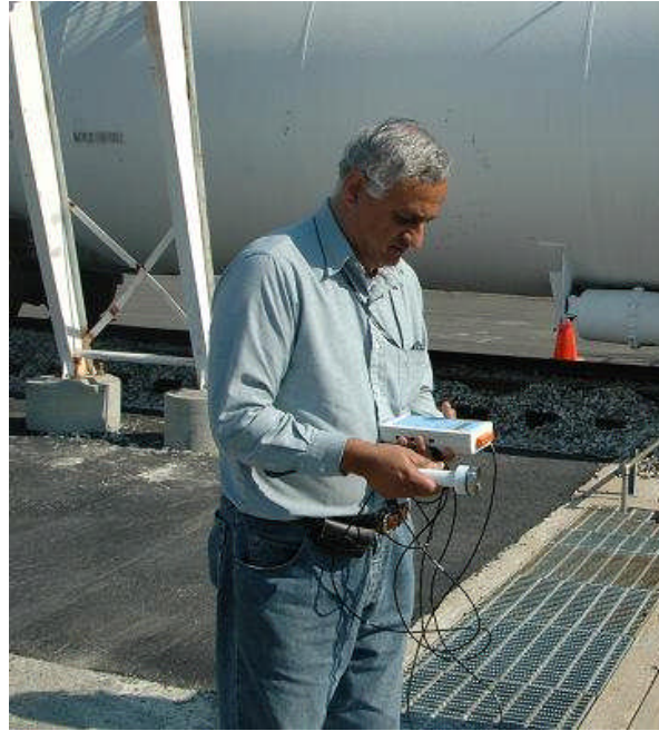
Figure 2-8: Handheld radiometer and illustration of its use in the field
