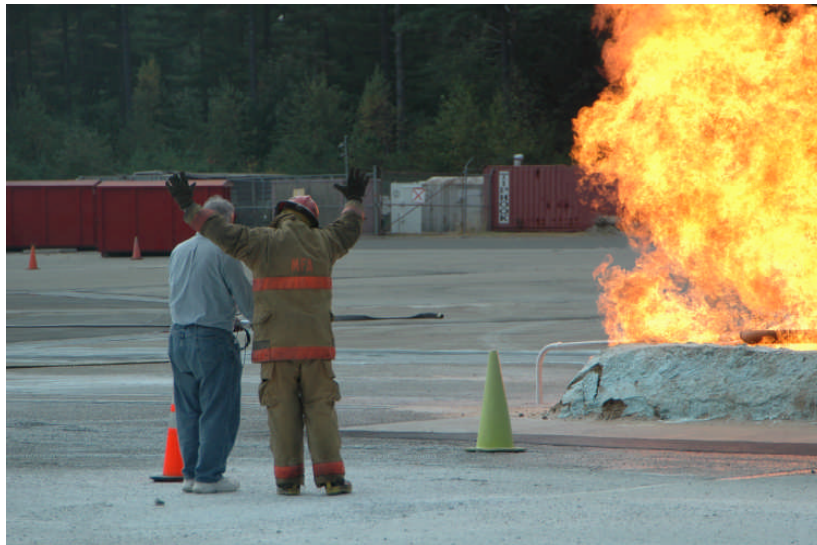
Figure 2-10: A location where the handheld radiometer indicated a 5 \text{ kW/m}^2 radiant heat flux (at about 30 ft from dike center)
