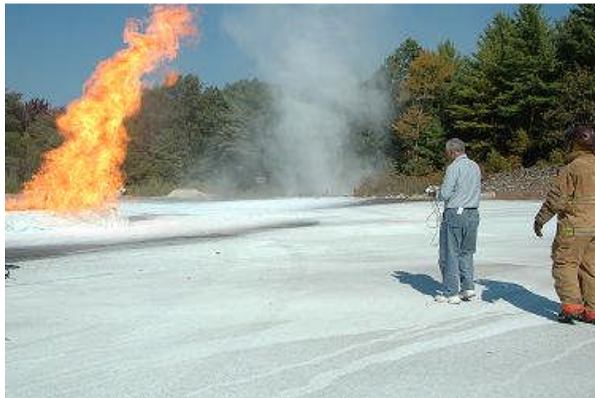
Figure E-3: The author facing the fire in civilian clothes. The handheld radiometer indicates the heat flux level to which he is being exposed
