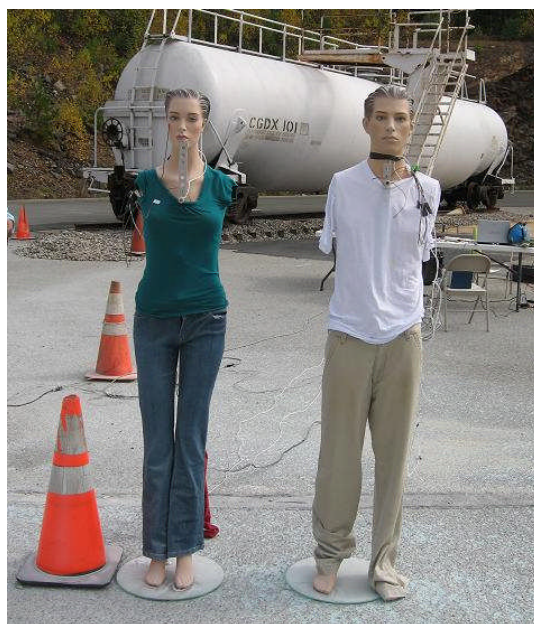
Figure 2-6: Picture of the fiberglass mannequins used in the field experiments
