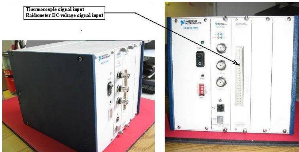
Figure A-12: Data Acquisition and Control Unit with thermocouple and radiometer signal input connector modules
