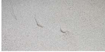
Figure 32. Photograph of mechanical damage on a pipeline section.
