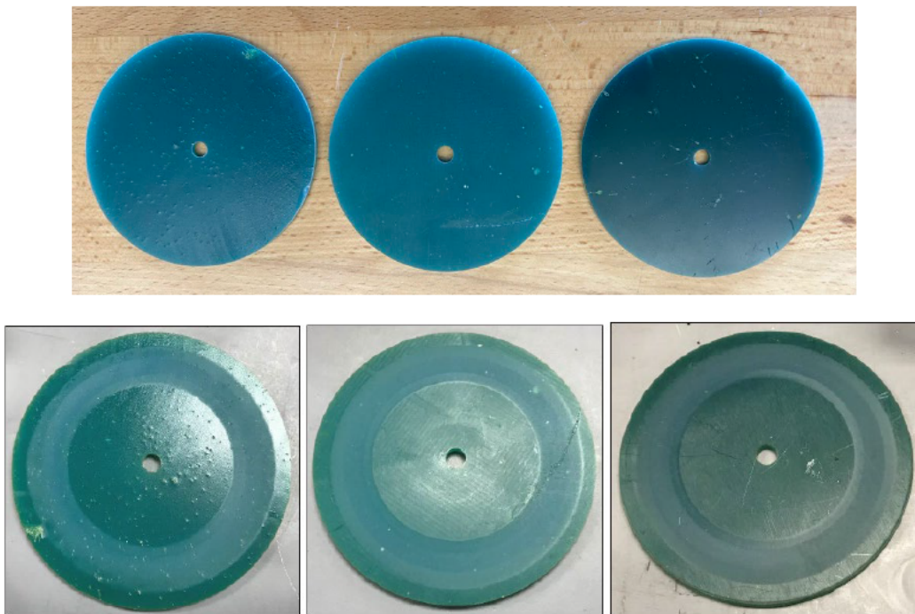
Figure 8. The images of the prepared discs for the abrasion test before (top) and after (bottom).
