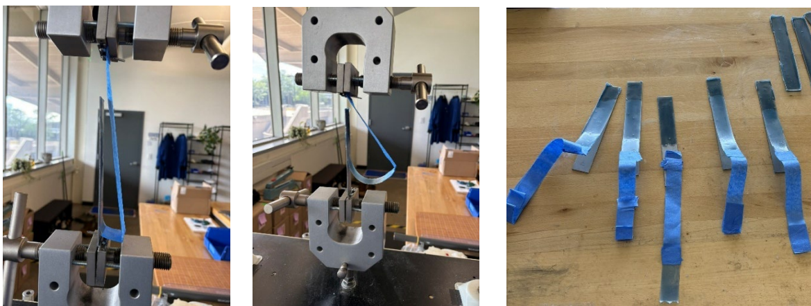
Figure 6. ASTM D903 testing trials with prepared specimens. Left: Attached specimen to the UTM instrument. Center: During the measurement/peeling. Right: Specimens after the test.
