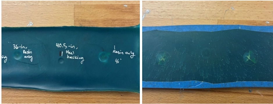
Figure 13. The preliminary test was performed with the resin only specimen. Strike from 46” and 36” cause failure/damage at the back of the resin.
