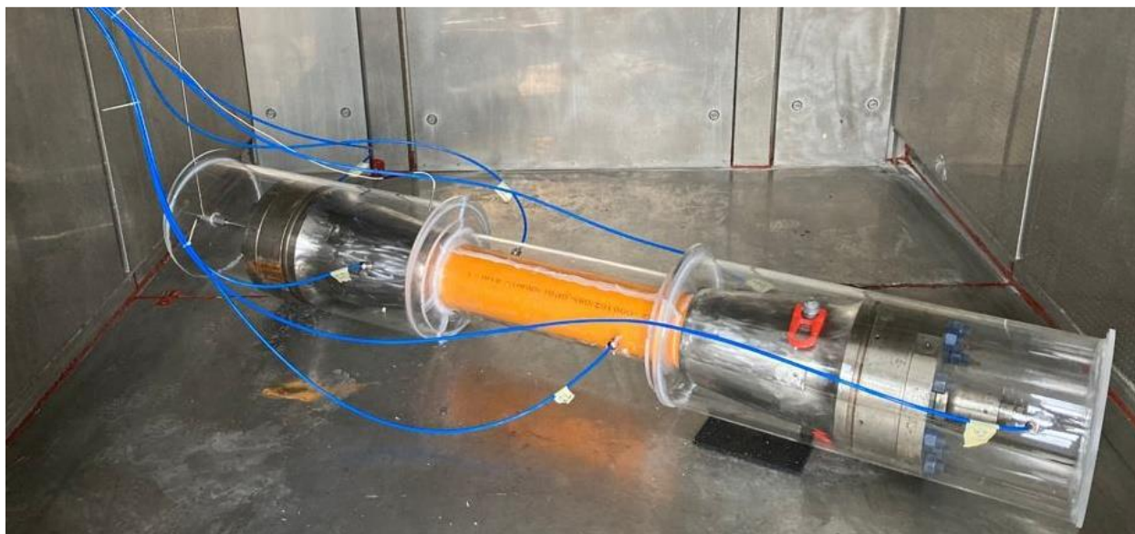
Figure 39. Pipe and End-Fitting Permeation Testing at Full Scale. (Frans Janssen, 2023)
