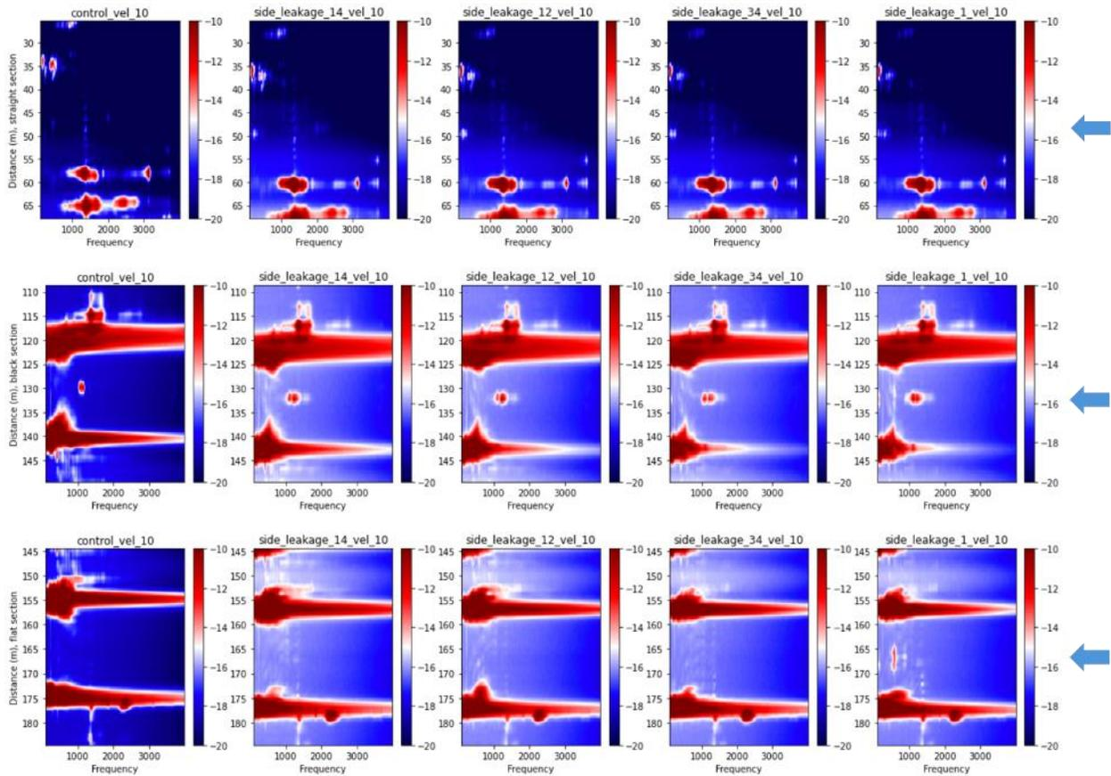
Figure 6. 2D spectra of fiber sections with varying leakage hole sizes at the side of the pipe, measured at a flow rate of 10 m/s. The top row displays the straight cable section, followed by the black, and the flat cable sections. Columns from left to right represent the control experiment (no leakage), followed by leakage sizes of  $\frac{1}{4}$ ",  $\frac{1}{2}$ ",  $\frac{3}{4}$ ", and 1", respectively. The color scale is measured in dB. Blue arrows indicate the leakage locations.
