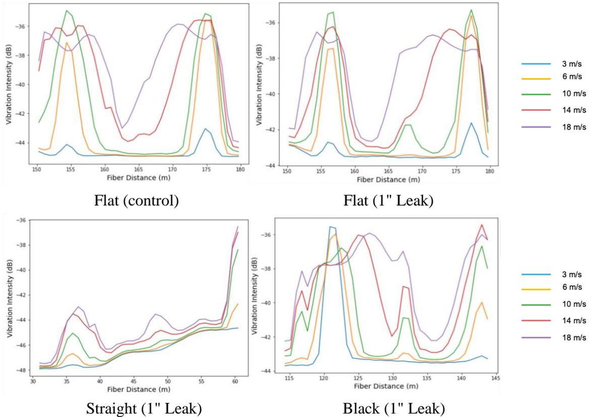
Figure 4. Comparison of the leakage detection sensitivity during a bottom leakage experiment across different cable types at varying flow velocities. Top left shows a flat cable without leakage as a control experiment. Top right features a flat cable with a leakage hole size of 1 inch. The bottom left, and bottom right sections present the straight, and black cables with the same leakage size of 1 inch, respectively.
