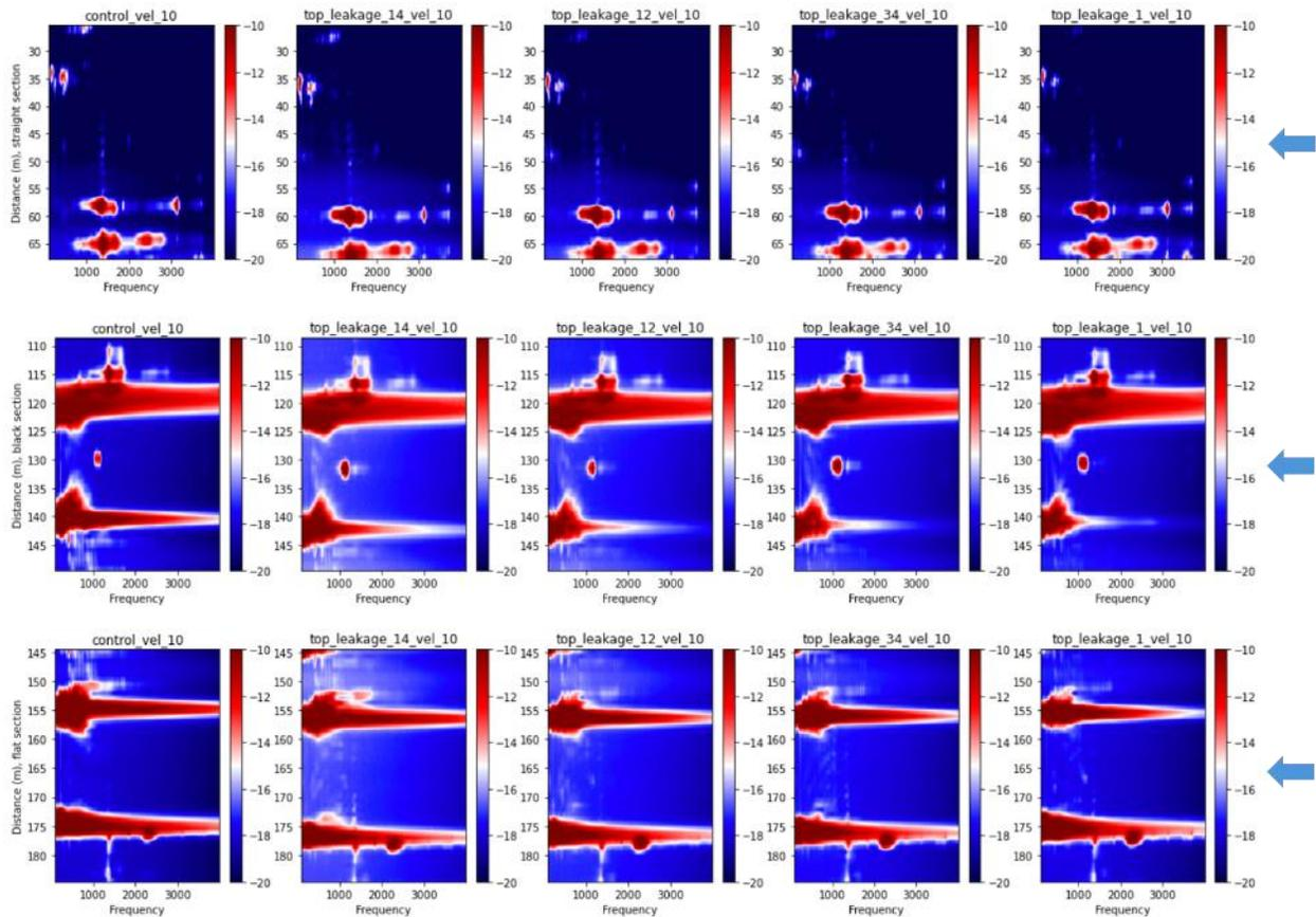
Figure 5. 2D spectra of fiber sections with varying leakage hole sizes at the top of the pipe, measured at a flow rate of 10 m/s. The top row displays the straight cable section, followed by the black, and the flat cable sections. Columns from left to right represent the control experiment (no leakage), followed by leakage sizes of  $\frac{1}{4}$ ",  $\frac{1}{2}$ ",  $\frac{3}{4}$ ", and 1", respectively. The color scale is measured in dB. Blue arrows indicate the leakage locations.
