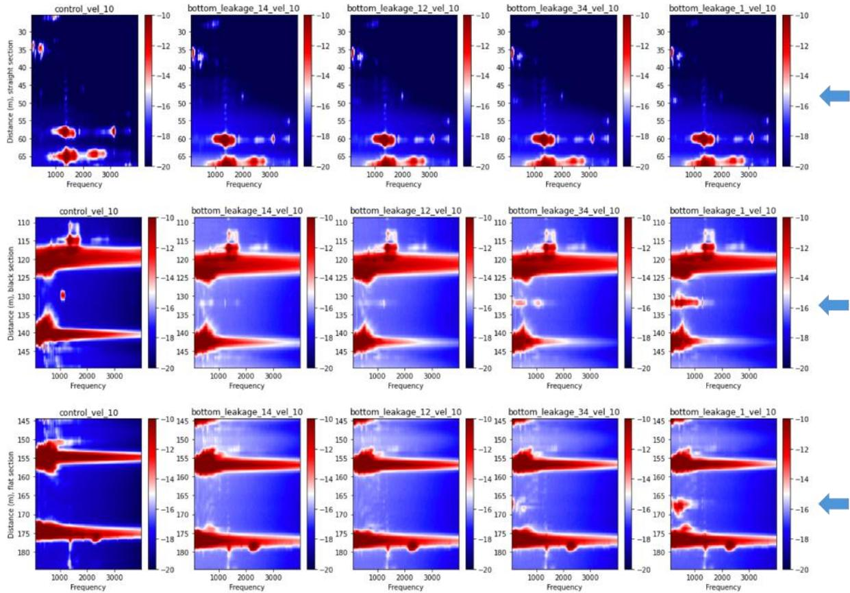
Figure 7. 2D spectra of fiber sections with varying leakage hole sizes at the bottom of the pipe, measured at a flow rate of 10 m/s. The top row displays the straight cable section, followed by the black, and the flat cable sections. Columns from left to right represent the control experiment (no leakage), followed by leakage sizes of  $\frac{1}{4}$ ",  $\frac{1}{2}$ ",  $\frac{3}{4}$ ", and 1", respectively. The color scale is measured in dB. Blue arrows indicate the leakage locations.
