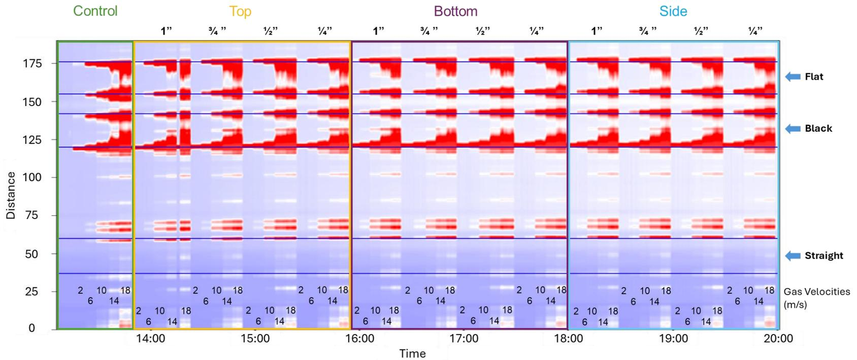
Figure 2. Magnitude of standard deviation values in straight external, black, and flat fiber sections during the control, top, bottom, and side leakage experiments with different hole sizes. The flow velocities inside the pipe change from 2, 6, 10, 14 and 18 m/s (indicated at the bottom left, which can be extended to other time period according to the vibration intensity or color). The arrows indicate the leakage location (at the center of all cable sections).
