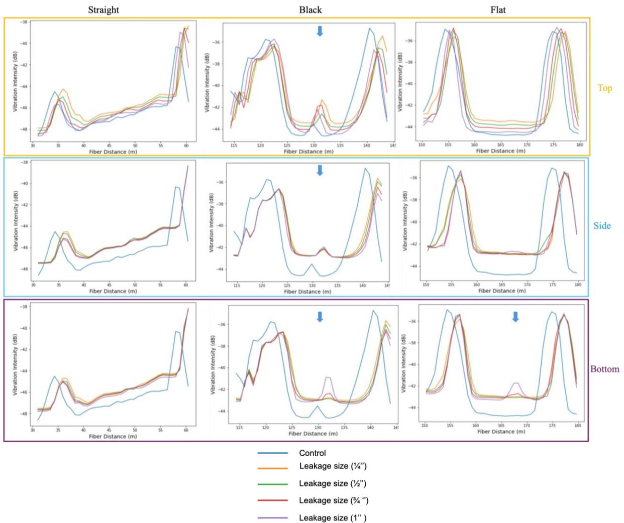
Figure 3. Vibration intensity profiles in straight external (left), black (middle), flat (right), fiber sections during the top, side, and bottom leakage experiments. The different curves represent vibration intensities associated with varying leakage hole sizes at a flow velocity of 10 m/s. Anomalies in vibration, induced by leakage holes and marked by blue arrows.
